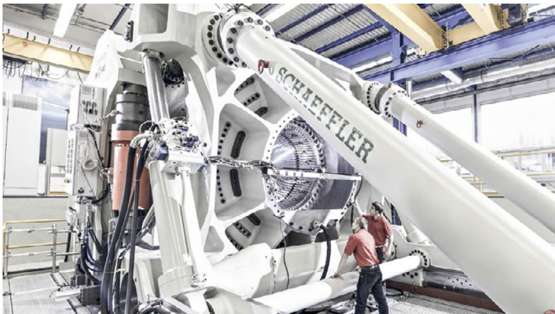
Impressive dimensions: the Astraios large-size bearing test stand in Schweinfurt
