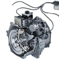
Double clutch with actuation and control unit
