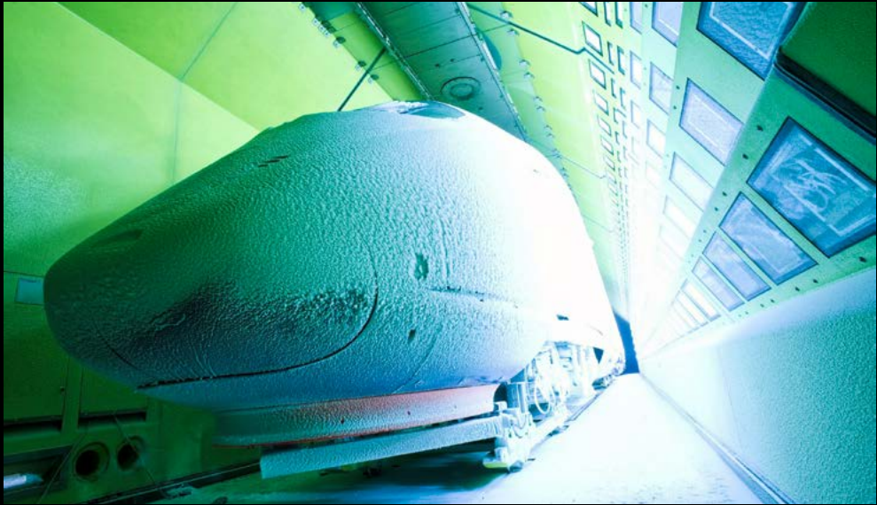
100 meters (328 feet) long and temperatures down to -45\text{ }^{\circ}\text{C} ( -49\text{ }^{\circ}\text{F} ) – RTA in Vienna is one of the world's largest climatic chambers
