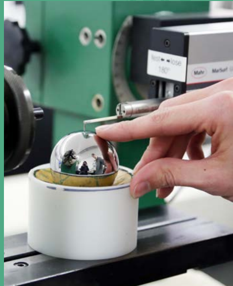
The Triondur-C-coated Schaeffler ball with a roundness of 160 nanometers (6.2992e-6 inches)
