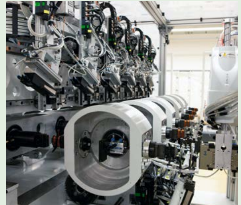
Six-spindle winding machine for high-volume production of up to one million units
