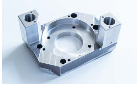
For this tool base frame of a press, two columns were "printed" onto a base plate using powder deposition welding in the 3D hybrid printer from DMG Mori depicted below and subsequently smoothed out by milling
