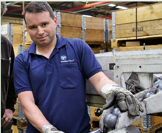
The balls Schaeffler assembles in rolling bearings have a size of up to 20 centimeters (7.9 inches)
