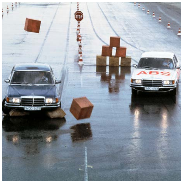
Braking, releasing, braking, releasing: the automatic cadence braking system ABS (anti-lock system) Mercedes introduced in high-volume production in 1978 ensures safe deceleration especially in slippery conditions
