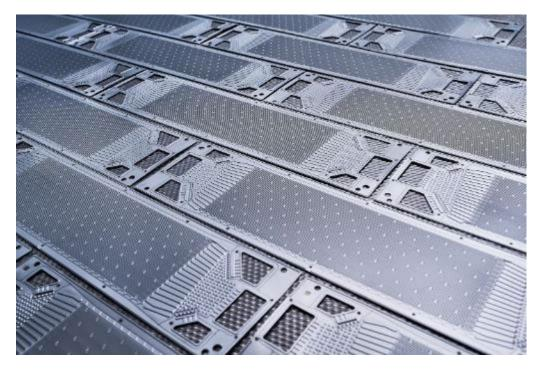
The newly established company Innoplate will accelerate the production of next generation bipolar plates (BPP) for the entire proton exchange membrane (PEM) fuel cell market. By 2030 the joint venture aims at producing around 50 million BPP annually, employing more than 120 people. (Photo: Schaeffler)
