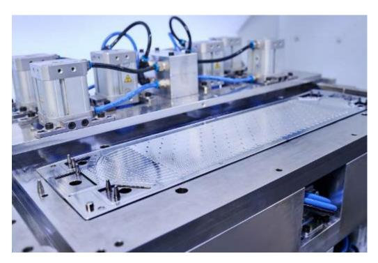
Metallic bipolar plates are a key element of fuel cell stacks. (Photo: Schaeffler)
