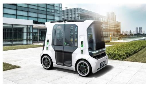
light is the Schaeffler Intelligent Corner Modules. In the four wheel modules, all drive and chassis components including the electric wheel hub motor are combined in one space-saving unit.
