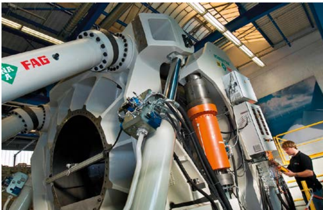
Large bearings with a diameter of up to 3.5 meters for wind turbines can be tested on the world’s only test rig for large-scale bearings Astraios – one of many forward-thinking solutions by Schaeffler
