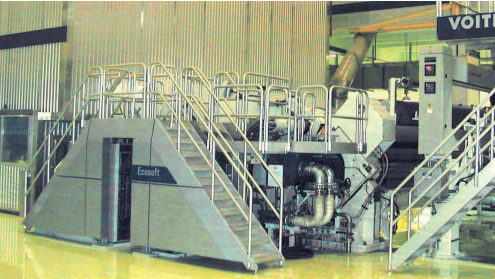
Calender for the new PM10 construction of the Shandong Huatai Paper Group
