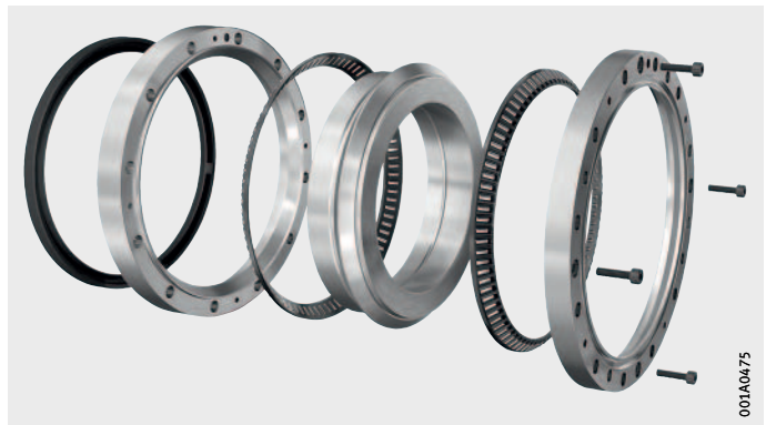
Figure 1 Exploded view of output bearing XZU
