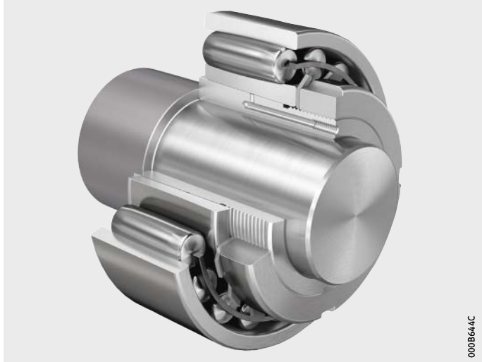
Figure 5 Shaft journal DEMO-MOUNTING.SHAFT-3.1 with toroidal roller bearing C2222-XL-K, adapter sleeve, locknut and tab washer
