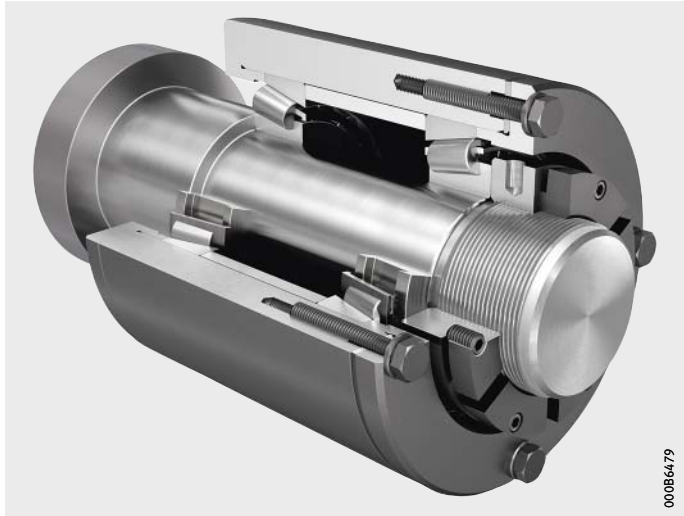
Figure 13 Shaft journal DEMO-MOUNTING.SHAFT-7.1 with tapered roller bearing 32210-A in O arrangement
