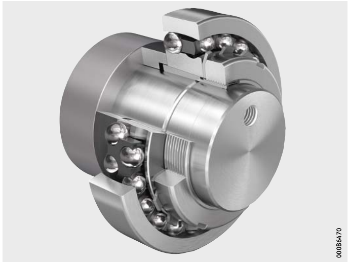
Figure 11 Shaft journal DEMO-MOUNTING.SHAFT-6 with self-aligning ball bearing 1213-K-TV-C3, L-section ring, adapter sleeve, locknut and tab washer
