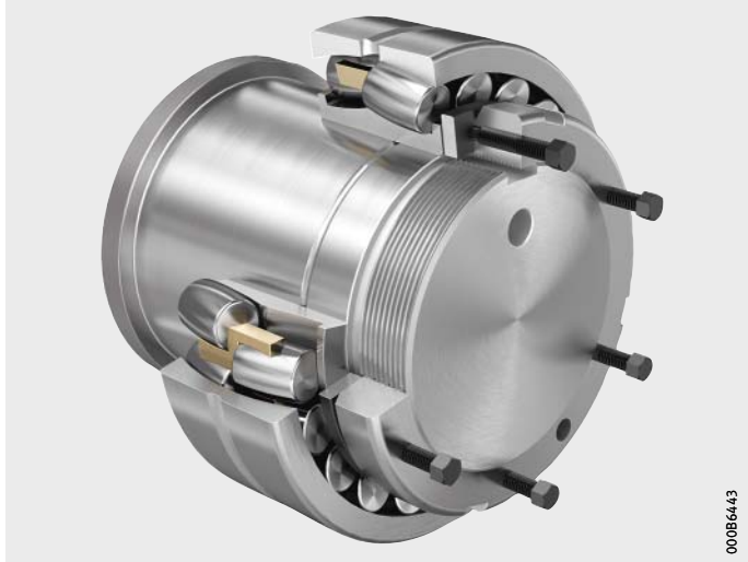
Figure 3 Shaft journal DEMO-MOUNTING.SHAFT-2 with spherical roller bearing 23120-E1A-XL-K-M-C3, spacer ring and locknut with pressure screws
