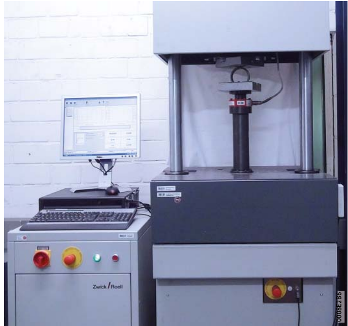
Figure 18 Dynamic radial loading of selector sleeve
