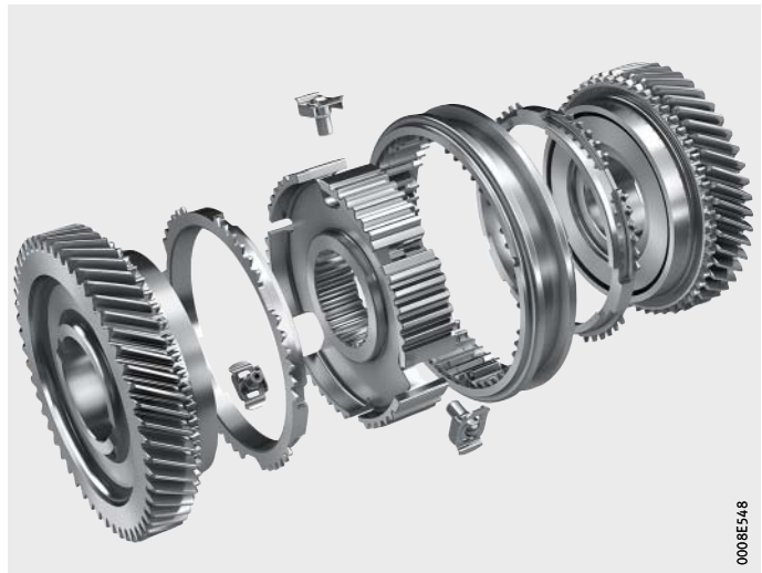
Figure 1 Conventional blocking synchromesh in accordance with the Borg-Warner or ZF-B system
