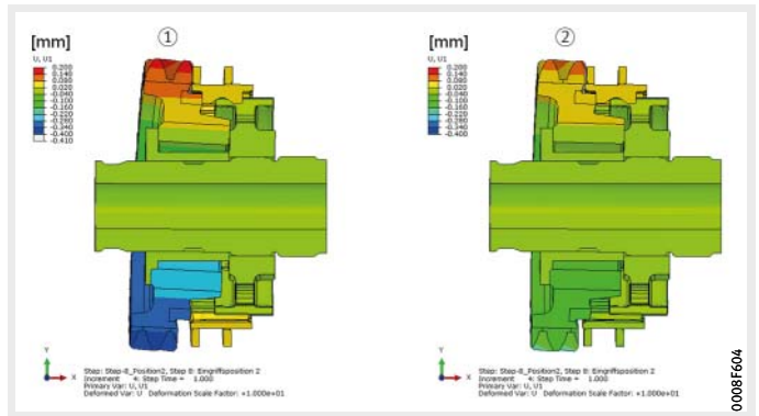
Figure 11 FEM calculation: stress distribution (dynamic)
