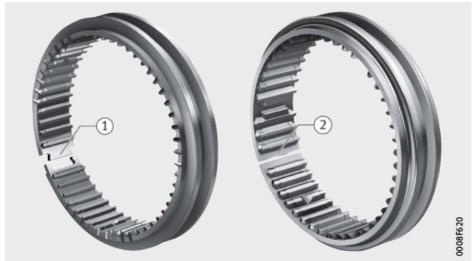
Figure 6 Selector sleeves with clinch and butt joint
