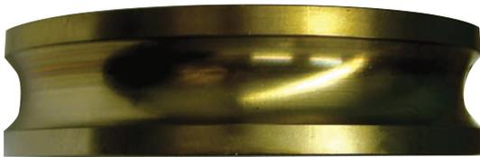
Fig7. Photograph of type 6217 inner ring showing running path offset from centre of raceway.
