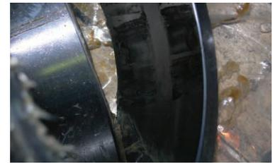
Fig14. Type 23036 spherical roller bearing outer ring raceway showing black corrosion stains.
