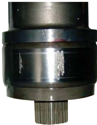
Figure 26. Damage on the bearing inner ring raceway of a gearbox output shaft
