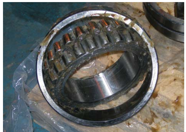
Figure 13. Type 23036 spherical roller bearing outer ring raceway showing black corrosion stains
