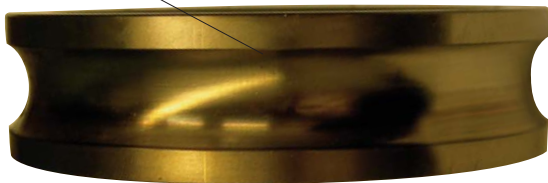
Figure 11. Photograph of type 6217 inner ring showing running path offset from centre of raceway
