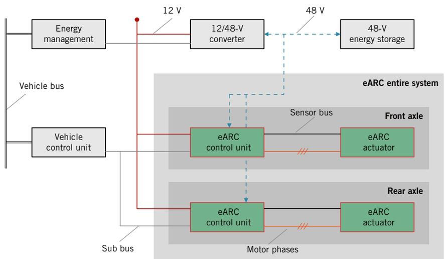
**FIGURE 1** Control unit topology and connecting of the eARC entire system to the vehicle architecture (© Schaeffler)
