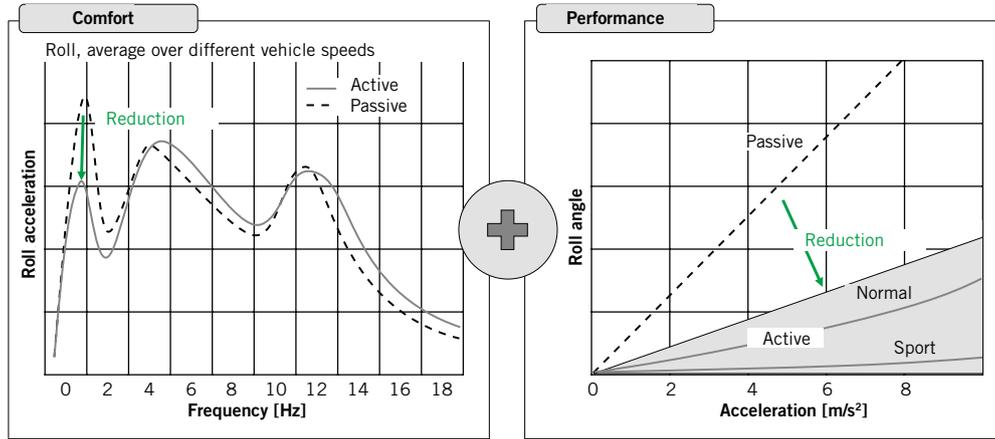
FIGURE 2 Qualitative presentation of reductions in roll accelerations and roll angles due to the eARC system for increase in comfort (left) and performance (right) [2] © Porsche
