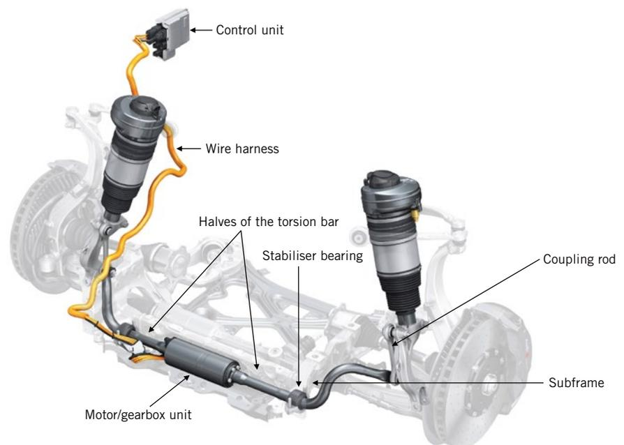
FIGURE 3 eARC system components and their installation in a front axle configuration for an Audi A7 © Audi, Schaeffler
