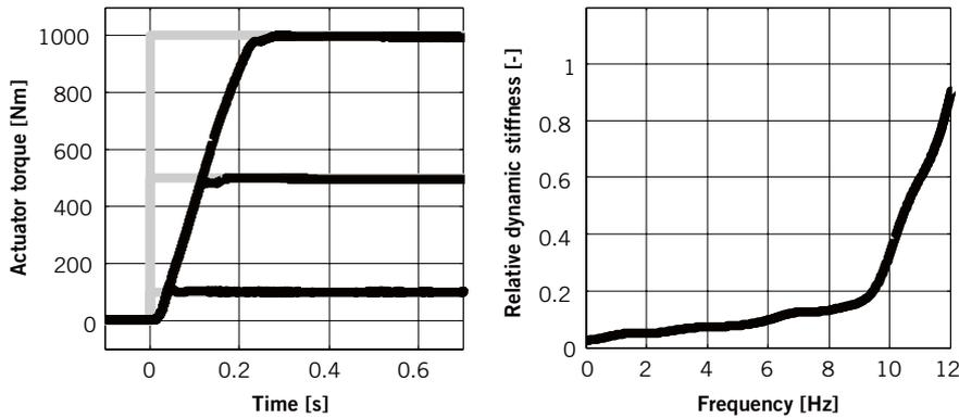
**FIGURE 6** Step response of the actuator torque (left) and relative dynamic rigidity of the actuator (right) (© Schaeffler)
