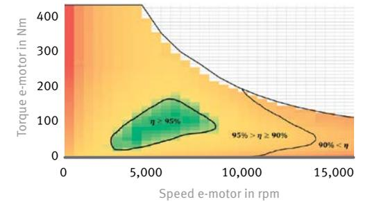
**4 Efficiency of the drive axle with 440 Nm PSM and power electronics**
