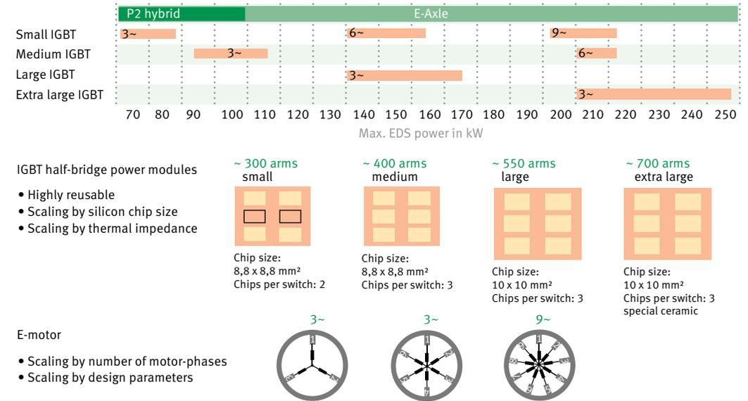
9 Power scaling through the size and number of IGBT semiconductors and the number of phases in the electric motor
