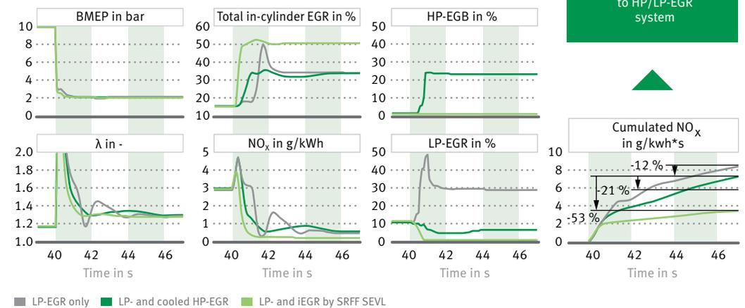
9 Switchable roller finger followers considerably reduce engine-out NO<sub>x</sub> emissions on a diesel engine
