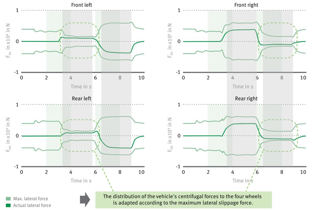
12 The driving dynamics controller controls the force distribution of the four wheel drives in such a way that the actual force is always below the friction contact limit
