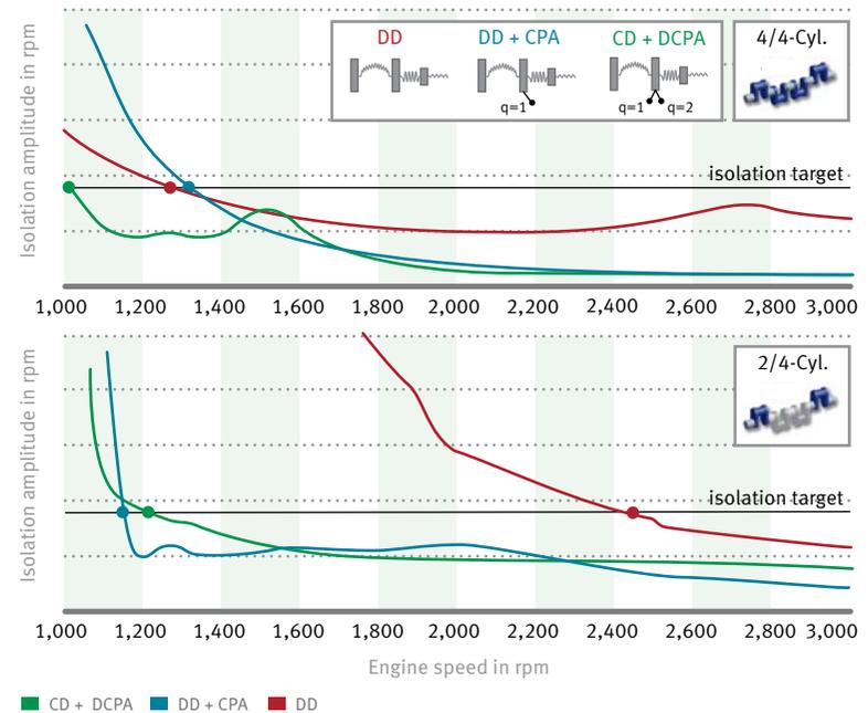
11 Isolation potential of torsion dampers with CPA and double CPA upon cylinder deactivation of two cylinders of a four-cylinder engine
