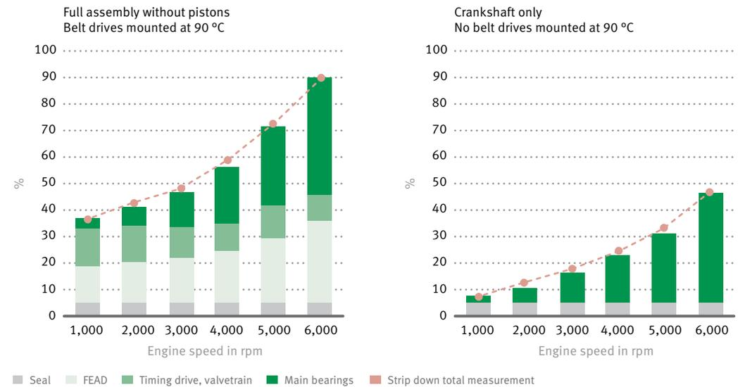
8 Comparison of measured and calculated friction values.
