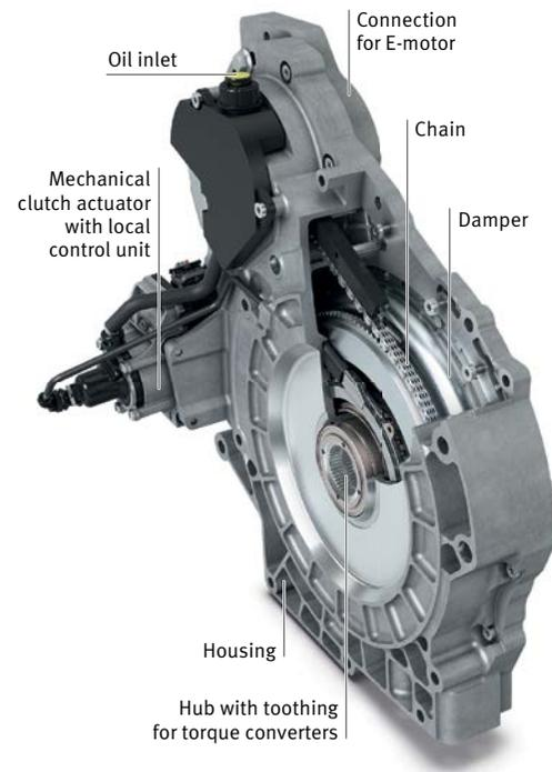
9 Subsystems of a high-voltage hybrid module for axially parallel installation
