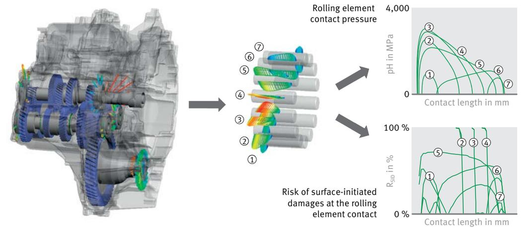
5 Modeling depth of BEARINX from the system level of the complete transmission to an individual contact
