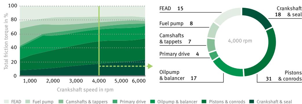
7 Breakdown of friction percentages using a strip-down measurement.
