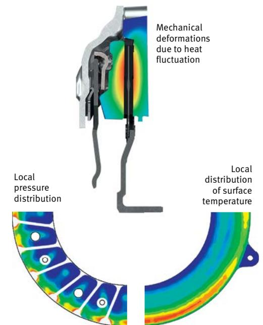
13 Interaction of pressure distribution with thermal and mechanical effects in the clutch
