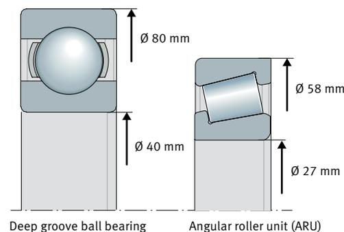
3 Comparison of the dimensions of a deep groove ball bearing and an angular roller unit with the same load rating
