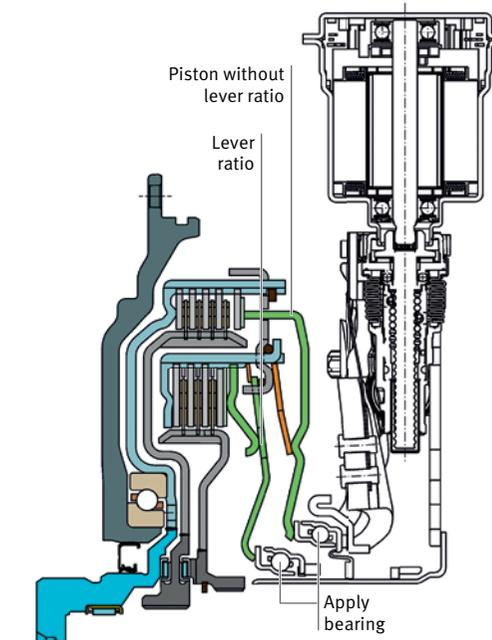
2 Half section of a wet double clutch with internal ratio on subclutch 2
