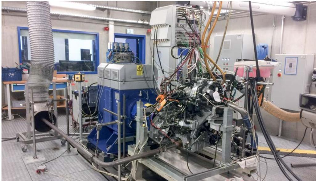
9 Set-up of the test bench for the fired engine tests
