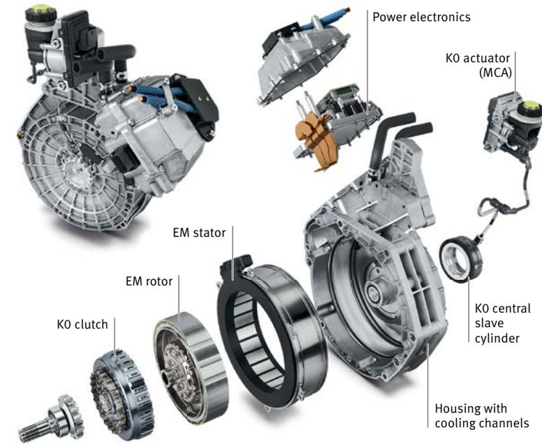
4 Design of the coaxial 48 volt P2 hybrid module with dry disconnect clutch KO
