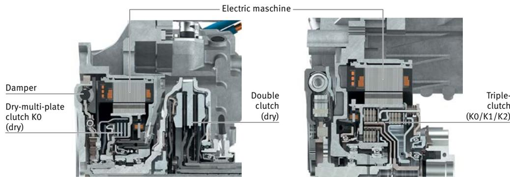
5 Cross-section through the coaxial 48 volt P2 hybrid module with damper on the engine side combined with either dry disconnect/double clutch option (left) or wet triple clutch (right)
