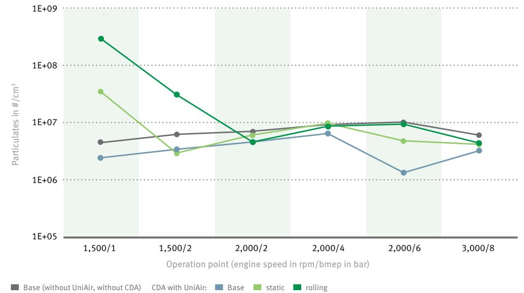
14 Measurement results of raw engine-out particulate emissions in steady-state deactivation mode
