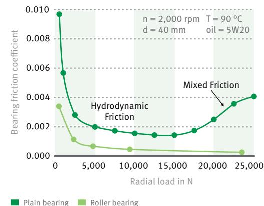
2 Comparison of friction between a cylindrical roller bearing and a plain bearing.
