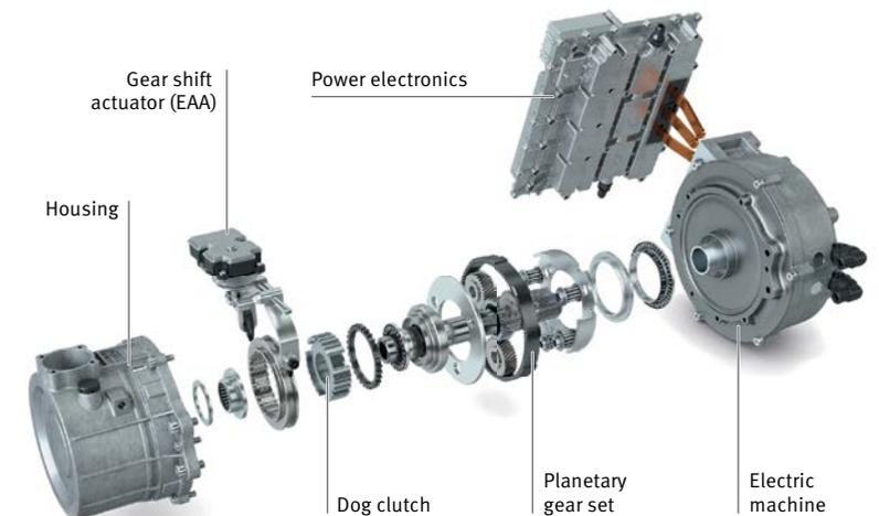
8 Construction of the single-speed (1+N) hybrid module for a 48 volt P3 hybridization (without optional multi-disk clutch for AWD)
