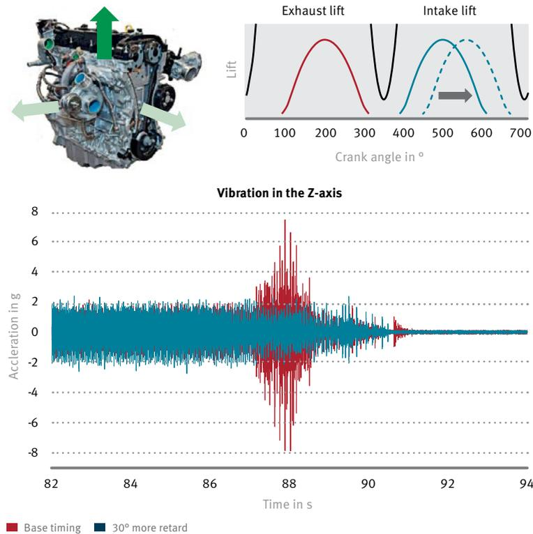
13 An intake camshaft adjustment reduces the acceleration amplitudes as the internal combustion engine enters shutdown
