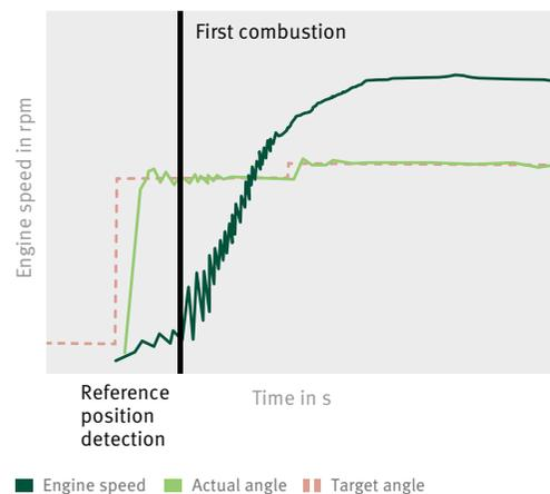
8 Timing adjustment with an electromechanical camshaft phasing unit at engine start-up
