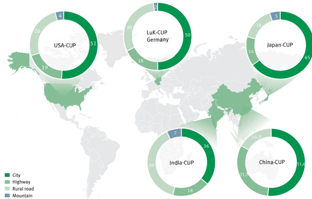
14 Driving profiles and load spectra worldwide, determined in a separate driving profile and broken down by city, freeway, highway and uphill starts (customer usage profile – CUP)
