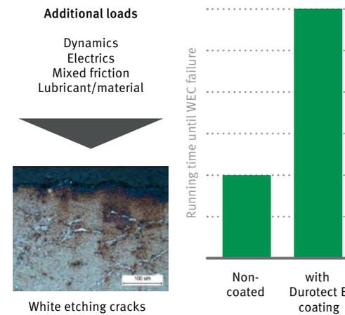
10 Increase in robustness against WEC damage with Durotect B
