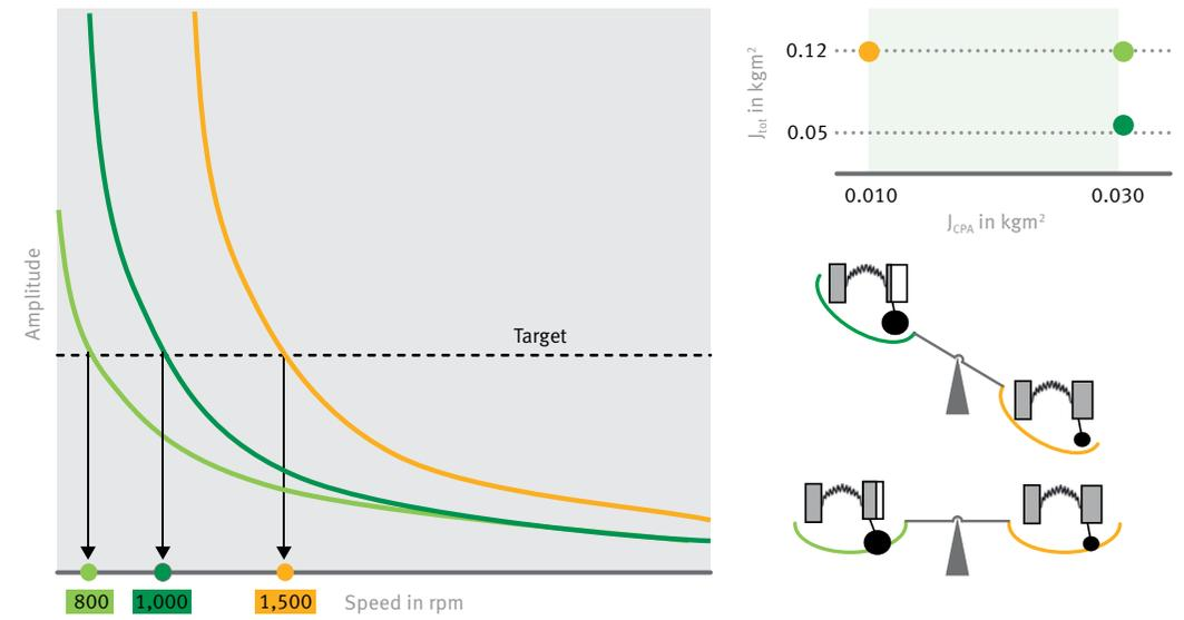
11 Theoretical potential of the CPA in the redistribution of the mass down to a reduction of the total mass of the damper system
