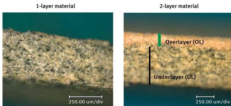
8 Schaeffler's wet friction lining as a one-layer design (left) and the new development approach with a two-layer wet running friction material (right)
