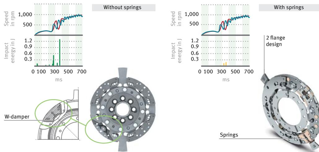
4 Design of an internal CPA with W stop damper (left) as well as tangential connecting elements on the pendulums (couple pendulum, right)
