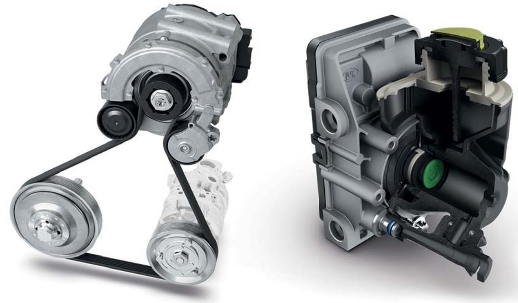
16 Schaeffler components interacting in the GTC I technology car: P0 belt drive with decoupling tensioner and crankshaft decoupling on the left; E-clutch actuator on the right
