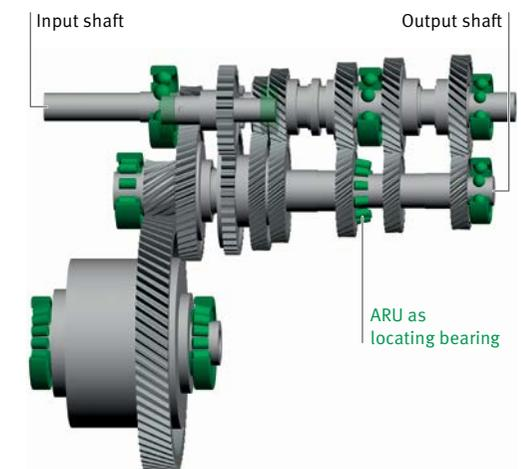
5 Mounting position of an angular roller unit (ARU) in a six-speed manual transmission on the transmission output shaft
