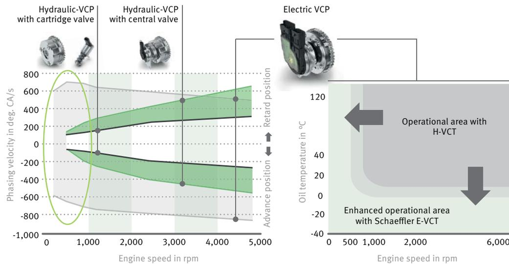
8 Electric camshaft phaser: Expansion of operating ranges (left) and higher phasing dynamics (right)
