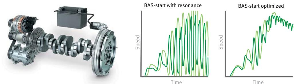
14 Vibration system of the belt drive – decoupler – crankshaft – dual-mass flywheel: rotational irregularities when starting the engine, both before (middle) and after optimization (right); green: crankshaft; bright green: belt pulley
