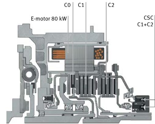
12 Triple clutch integrated inside the rotor
