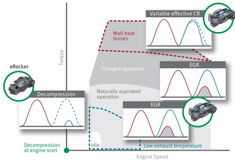
7 Switching strategies for the variable valve train in a diesel engine
