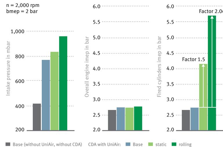
12 Measurement results: Intake manifold pressure and indicated mean effective pressure for different operating strategies
