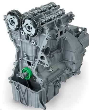
also be verified by extensive measurements. Across the entire engine performance map analyzed, the rolling bearing revealed substantial benefits over the plain bearing. This effect is especially well pronounced under conditions involving high loads and low speeds.
