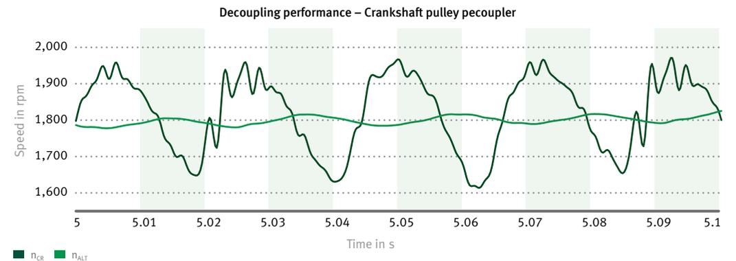
5 Decrease in engine irregularities by using a crankshaft decoupler. Graphed here are speeds over time during generator operation; the BSG speed is converted to the crankshaft
