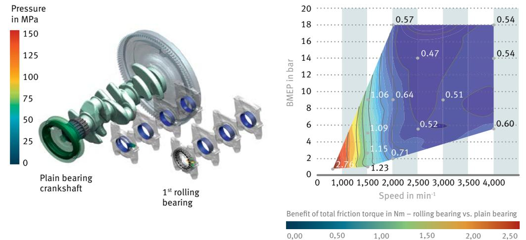
13 Friction power vs. effective medium pressure and speed in a three-cylinder engine with a displacement of 1.0 l and a P0 belt drive. Using color gradients, the diagram shows the advantage in the overall drive torque in the case of a rolling bearing arrangement in the first position of the crankshaft.
