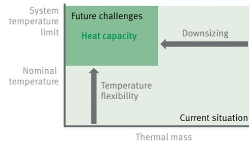
1 High heat inputs and low heat capacity will characterize the engine cooling circuit of the future.
