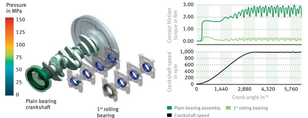
15 The start sequence of a P0 hybrid application as compared with a plain bearing and a rolling bearing assembly.
