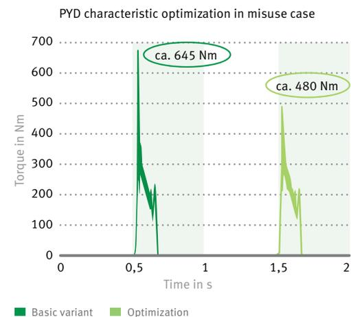
10 Torque at the interface to the crankshaft
