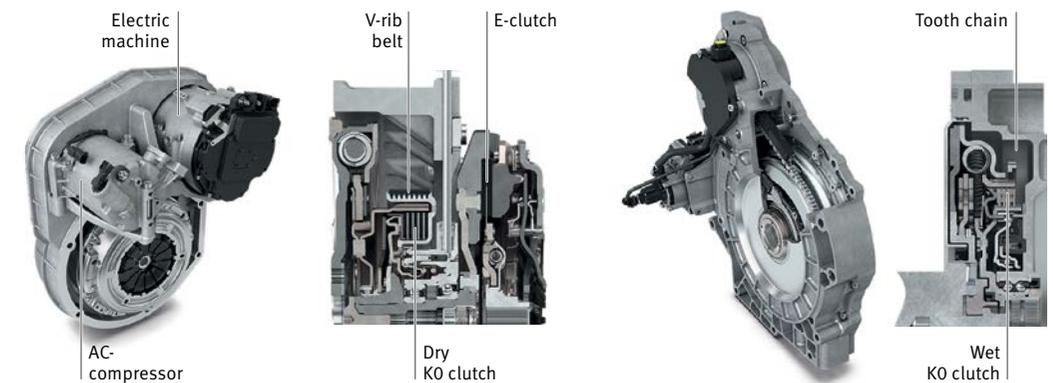
6 P2 hybrid module with belt (left) and chain (right) for parallel axis installation
