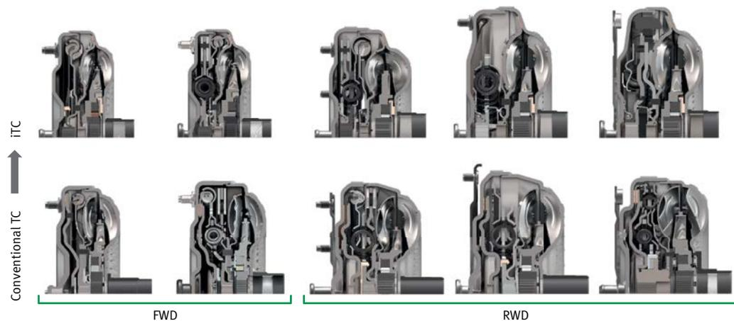
5 Integrated torque converters (iTC, top) for front-wheel (FWD, left) and rear-wheel drives (RWD, right).
