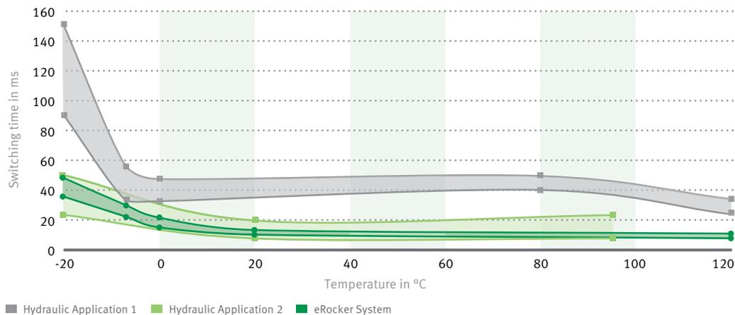
13 Switching time for interlocking SEVL systems in relation to oil temperature and internal engine constraints
