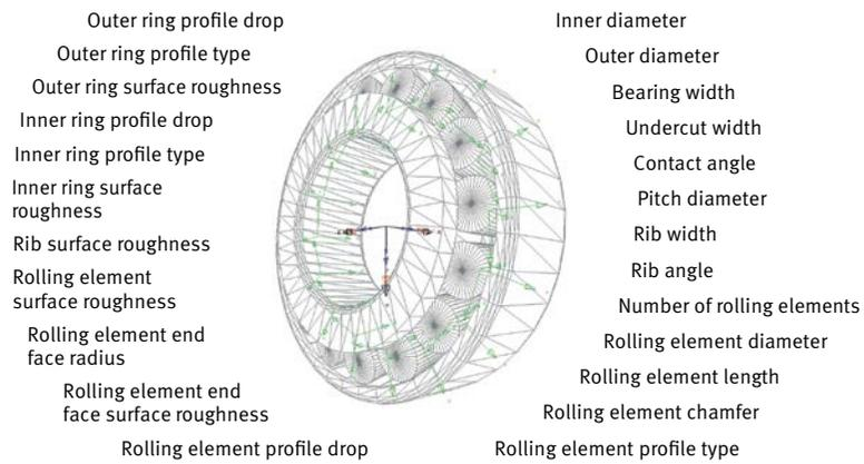
6 Variety of parameters and influencing factors in the design and optimization of transmission bearings using a tapered roller bearing as an example
