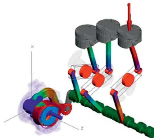
5 MBS model for quantifying the loads on the actuator
