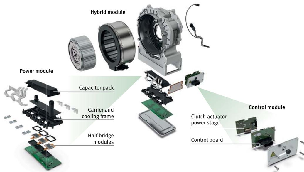
8 Modular concept for power electronics, taking a hybrid module as an example
