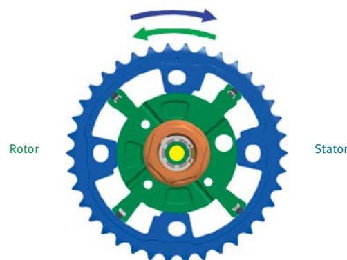
1 Design of a hydraulic camshaft phasing unit
