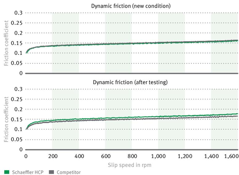
7 Benchmark results for the dynamic friction coefficient of Schaeffler's wet friction lining and a competitor product (new and after endurance test)
