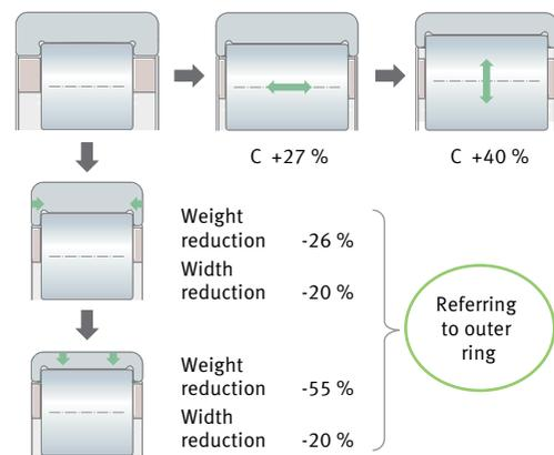
9 Increase in radial load capacity and reduction of design space requirements and weight through an improved design using an RNU308-E-XL type cylindrical roller bearing as an example
