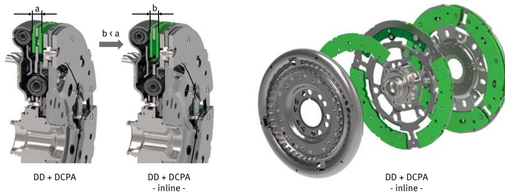
10 Design of the inline CPA using a DTD with a double CPA as an example
