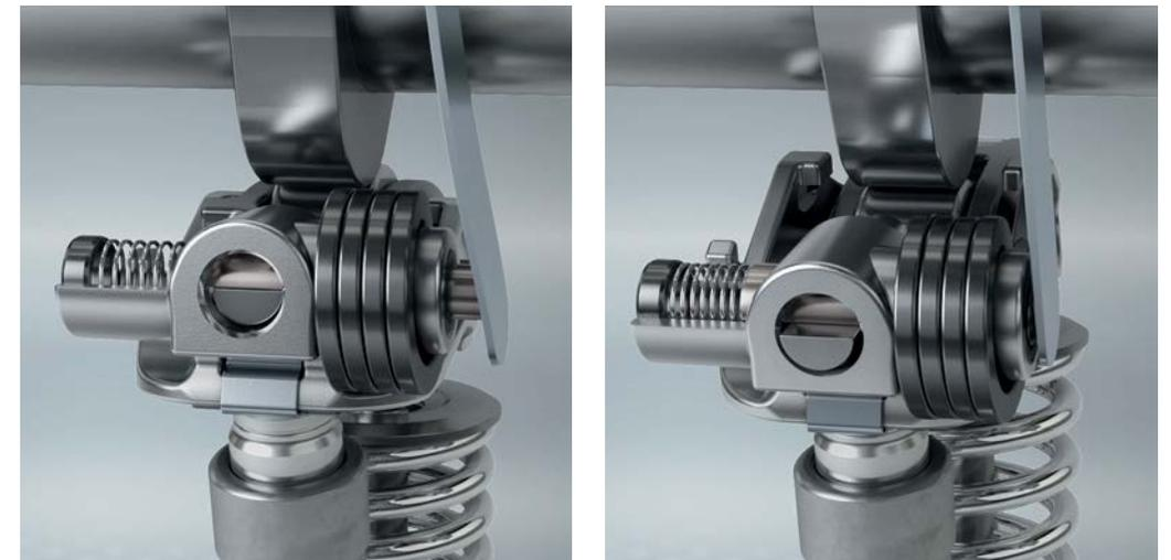
6 Actuator/slider bar motion with blocked locking pin via spring arm (left) and position after displacement (valve deactivated, right); locking mechanism partially cut away
