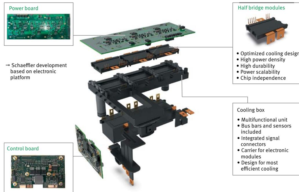
10 Power electronics setup for an electric axle drive
