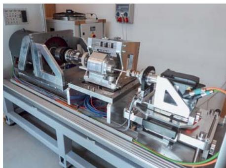
7 Example of a development sample for the gearbox for the multi-link phasing system and gearbox test stand for component testing
