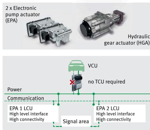
13 Actuator system for double clutch transmissions with two EPA and one HGA. A transmission control unit (TCU) is not required because the EPA performs this function.
