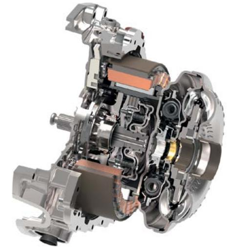
5 Hybrid module with integral converter
