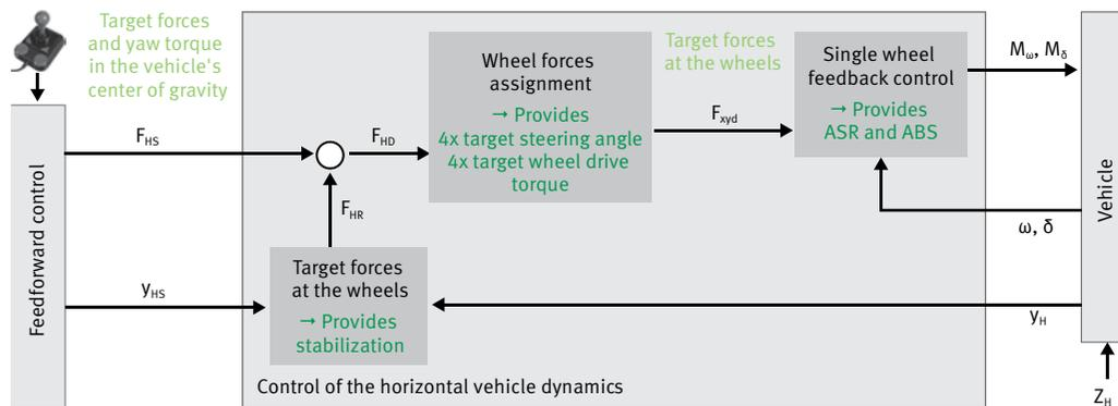
11 Signal flow in the electronic module and the individual components of the controller
