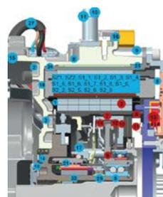
Several thermal sensors to collect the temperature behavior of the HYM components during all tests
