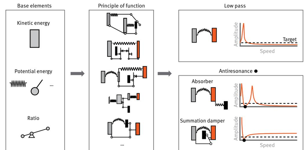
9 Various operating principles for damping vibrations
