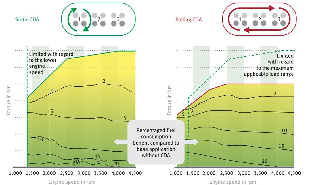
12 Comparison of operating ranges for static and rolling cylinder deactivation
