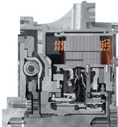
3 Cross-section through the second generation hybrid module in a dry clutch design
