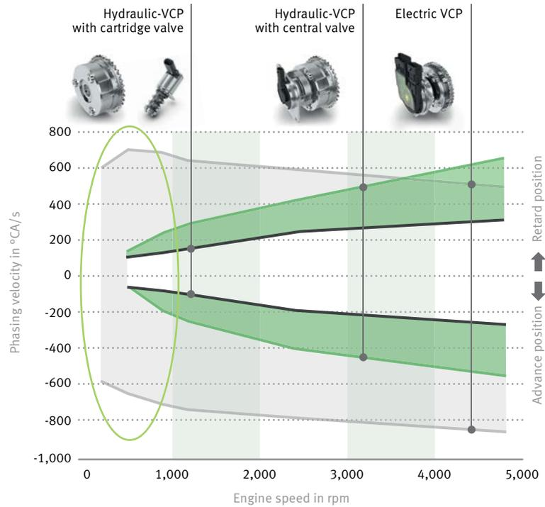
7 Phasing speed of different camshaft phasing systems in relation to the engine speed.
