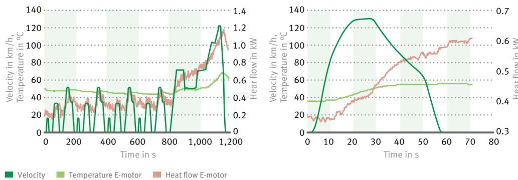
9 Model calculations for the heat entry through the electric motor in the NEDC (left) and during full-load acceleration
