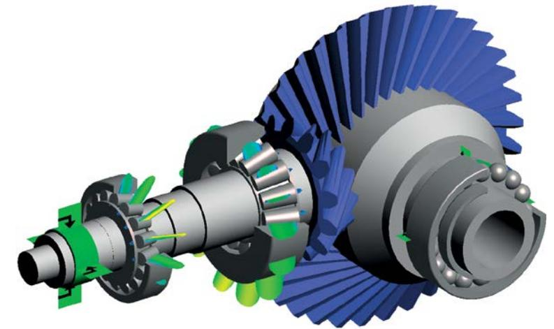
8 Model of the rear axle drive to be optimized in BEARINX
