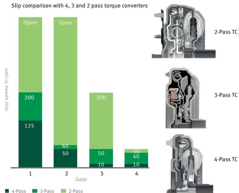
3 Comparison of the slip speeds of two-pass, three-pass and four-pass systems.
