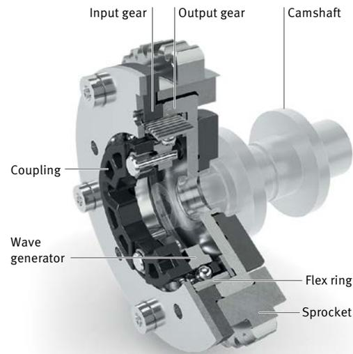
4 Design of the gear-set for the electromechanical cam phaser
