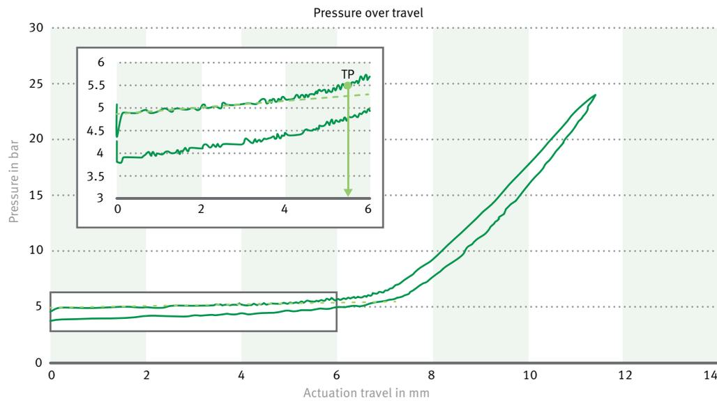
13 Determination of the touch point by means of the pressure-travel characteristic curve of a double clutch system
