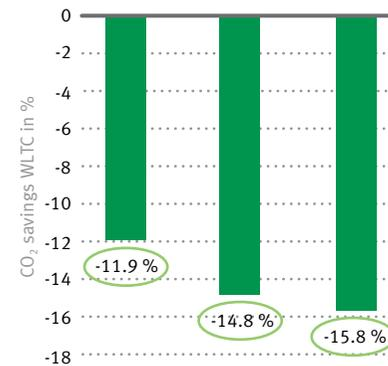
7 Simulated CO<sub>2</sub> savings by P2 hybrids when using a parallel axis and coaxial 48 volt hybrid module
