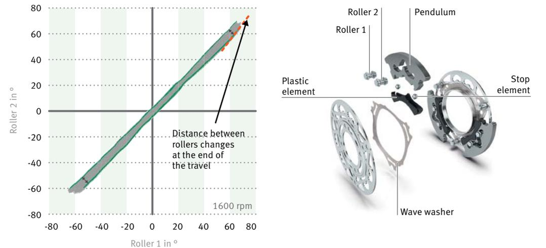
7 The distance between the rollers with multiple pendulum motions (left) and inserted friction elements for roller stabilization (right)
