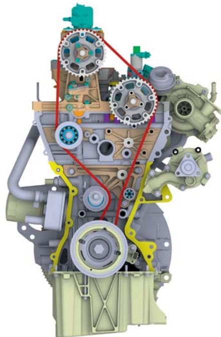
11 Prototype engine used to investigate the rolling cylinder deactivation system
