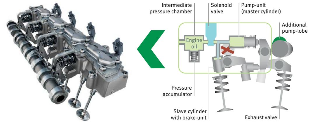
2 Design of the electrohydraulic UniAir system
