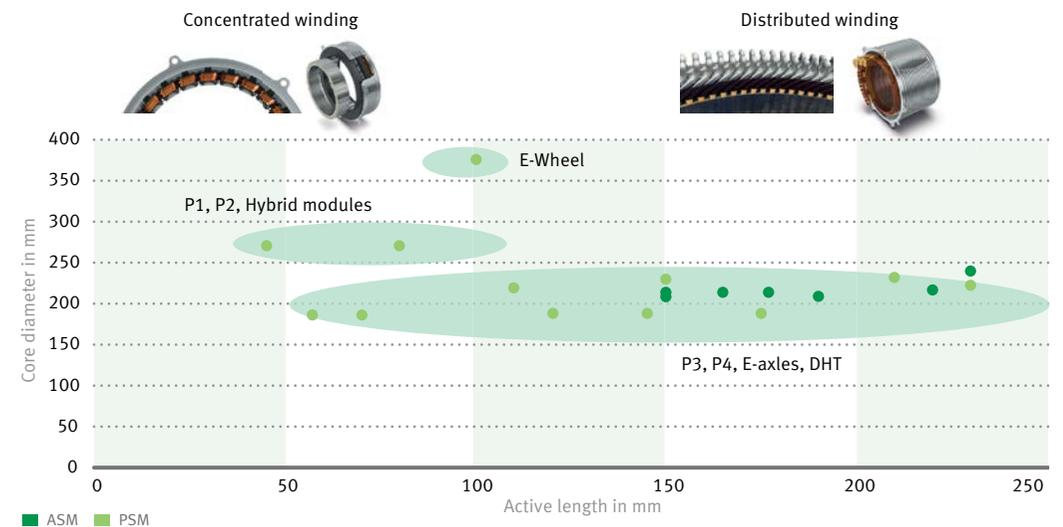
3 Application areas of concentrated and distributed winding, depending on the active length of the electric motor
