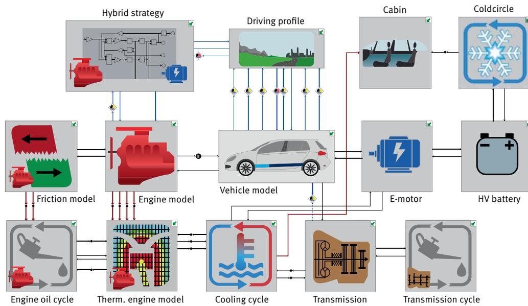
8 Simulation model for a plug-in hybrid vehicle
