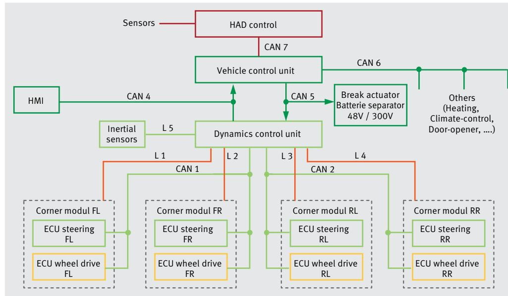
10 Signal flows for controlling the wheel modules
