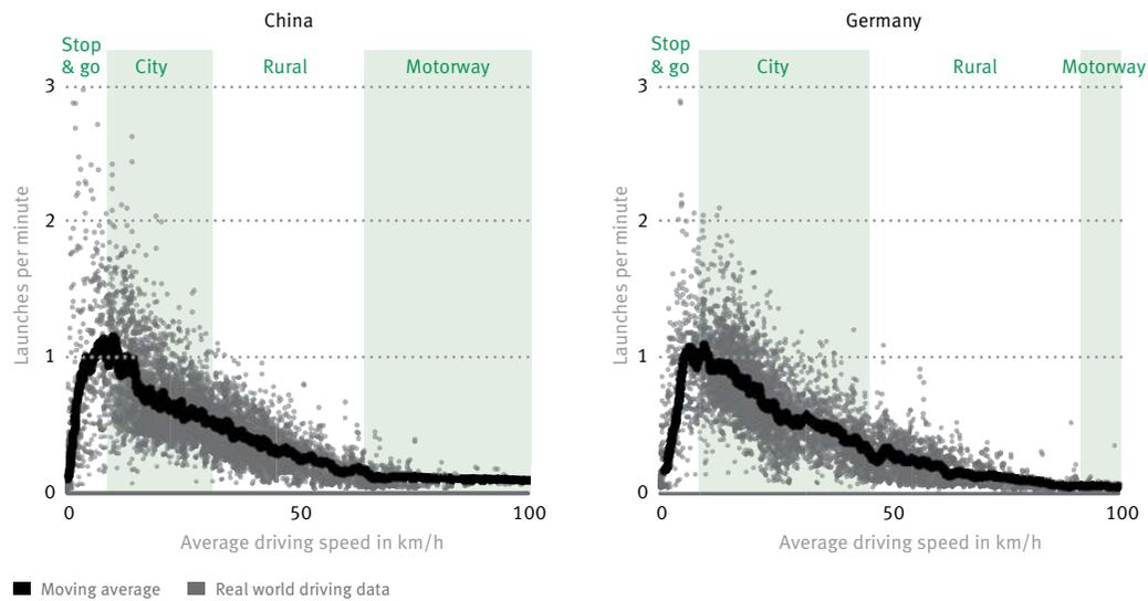
18 Analysis of real driving data on the distribution of the start frequency of individual driving ranges based on average speed
