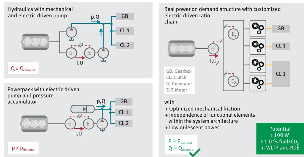
3 Comparison of real power-on-demand actuators (right) with hydraulic solutions and power packs
