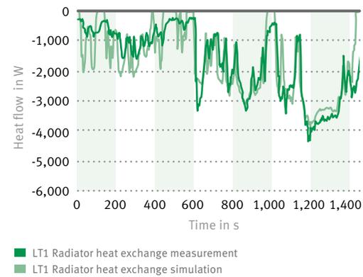
10 Measured and simulated heat exchange in the low-temperature heat exchanger of a plug-in hybrid vehicle
