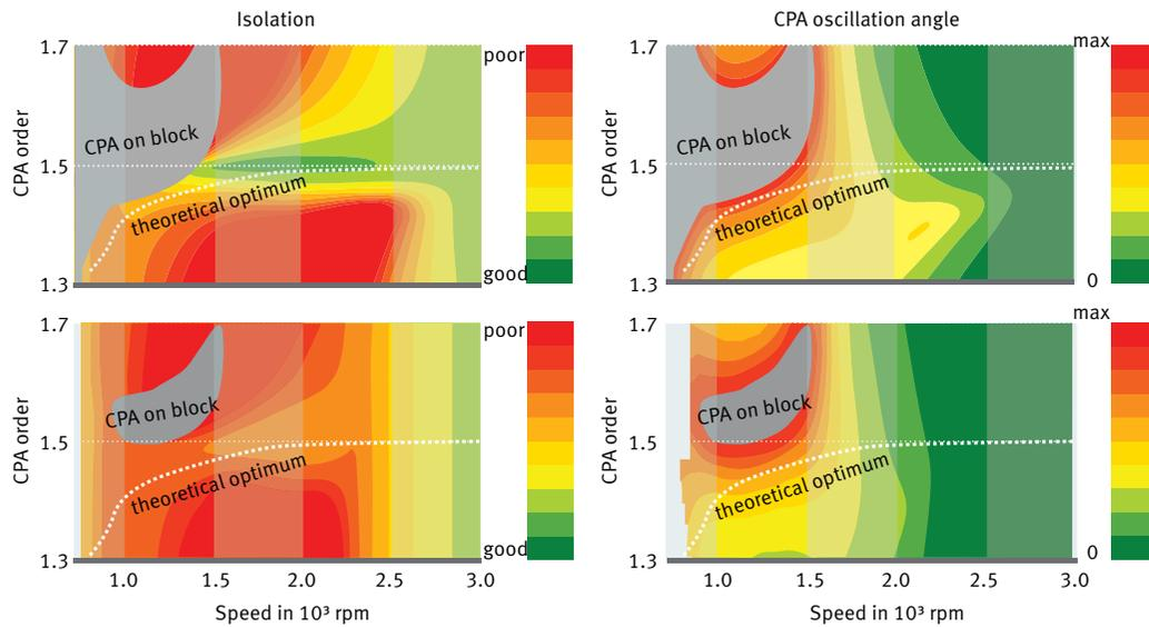
6 Basic simulation for optimization of the guide track curvature of the pendulum and the flange in combination with the roller diameter using the example of an CPA on the clutch disk without (top) and with (bottom) friction elements
