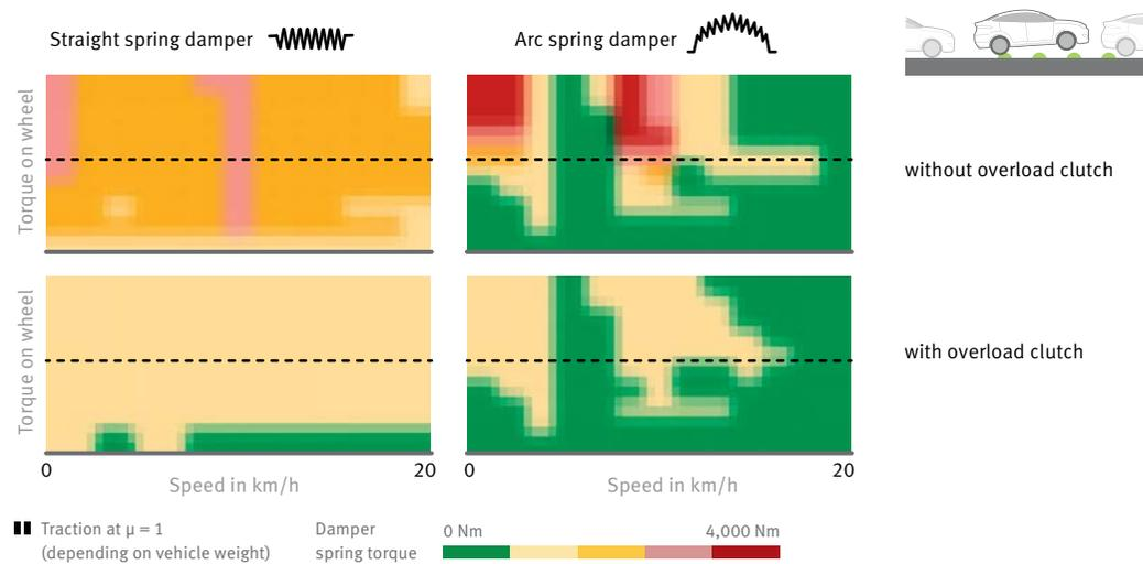
4 Simulation results for bumpy roads with driving range variations for four different damper systems
