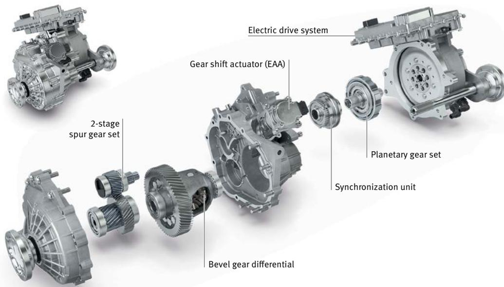
9 Construction of two-speed (2 + N) electric axle for a 48 volt P4 hybridization
