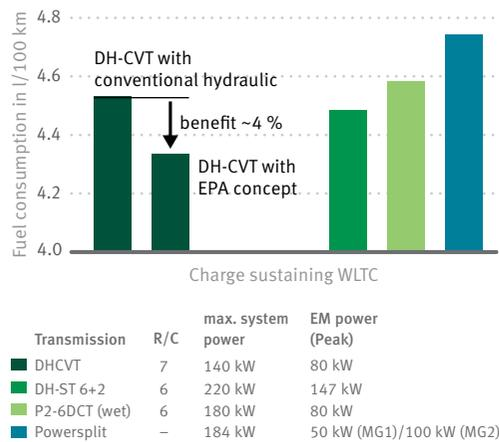
12 Comparison of the fuel efficiency of various hybrid drives in charge sustaining mode
