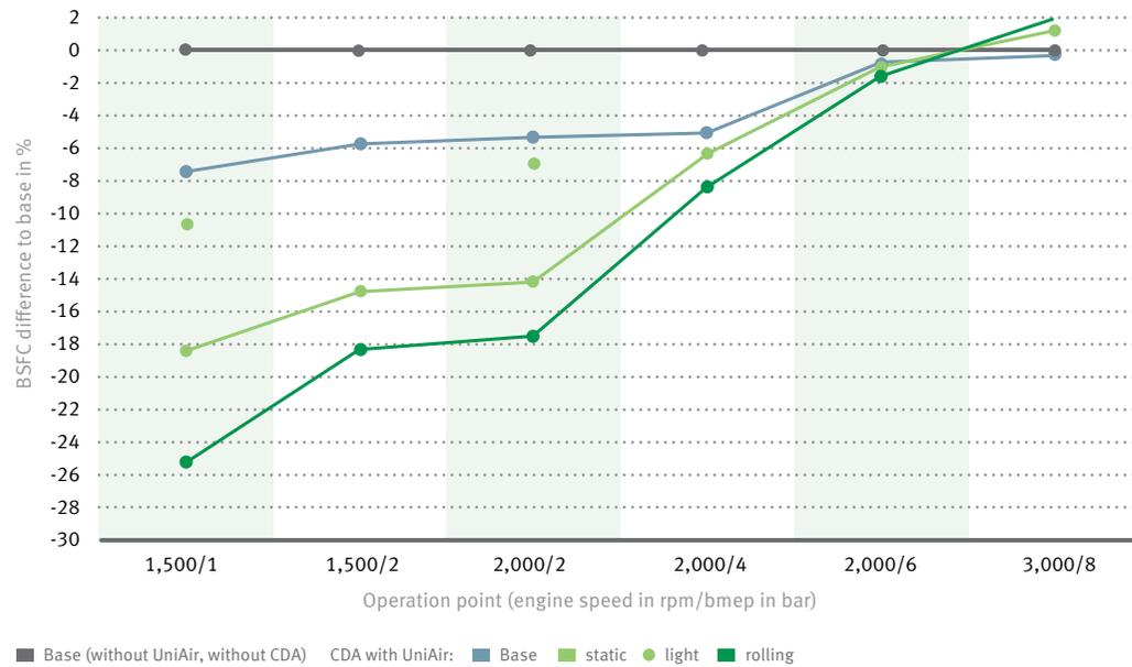
11 Impact of EIVC and cylinder deactivation on specific fuel consumption
