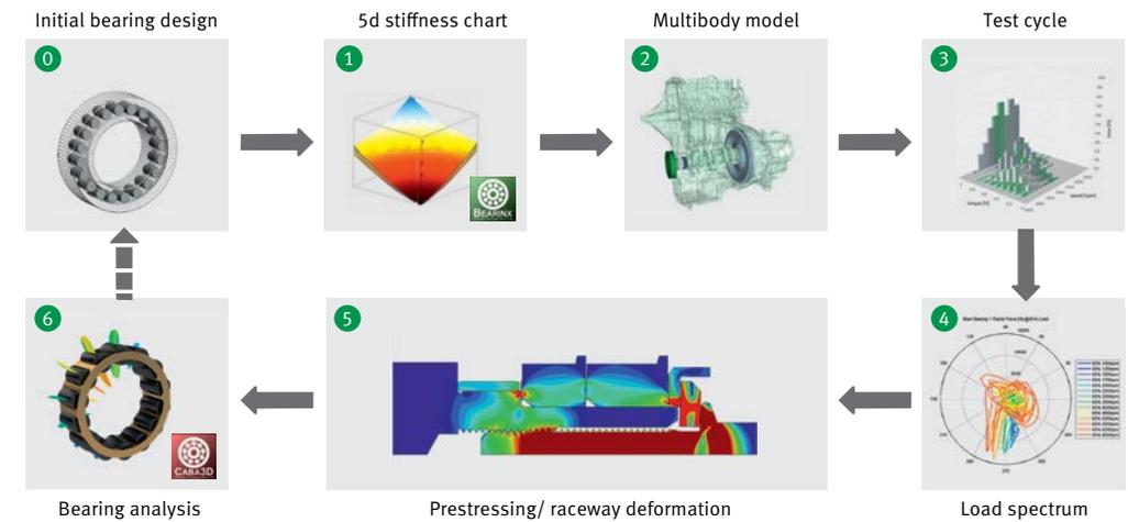
4 Self-contained development process for designing crankshaft bearings.
