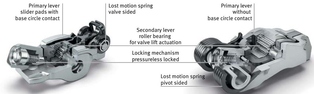
2 Switchable roller finger followers on an early generation (left) and on the current generation (right) for gasoline engines
