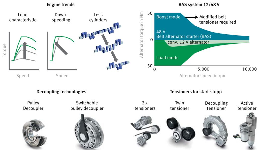
6 Tensioning systems and decouplers for P0 systems
