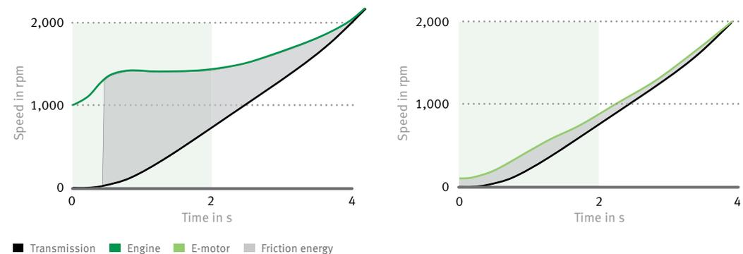
3 Clutch slip during vehicle launch with a combustion engine (left) and an electric motor (right)
