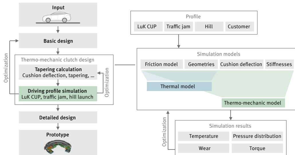
14 Schematic diagram of the optimized thermal clutch design
