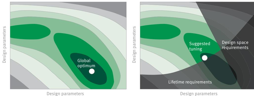
7 Comparison of the function of a classic optimization algorithm (left) and a real-life optimization based on development requirements (right)
