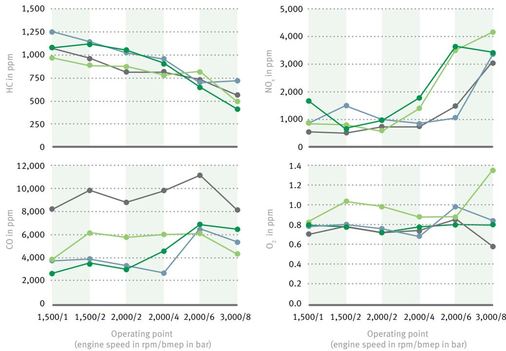
13 Measurement results of gaseous untreated emissions and O<sub>2</sub> concentration levels
