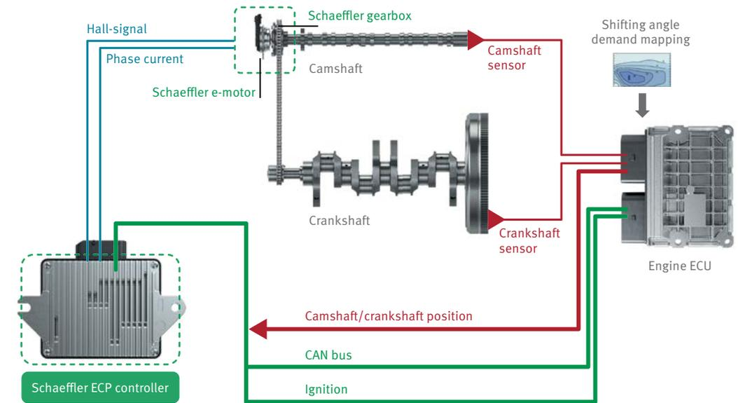
5 Topology of the electromechanical cam phaser
