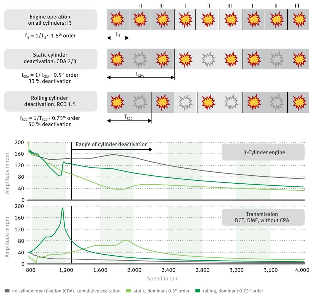
1 Deactivation level and torsional vibration excitation of different deactivation strategies for three-cylinder engines
