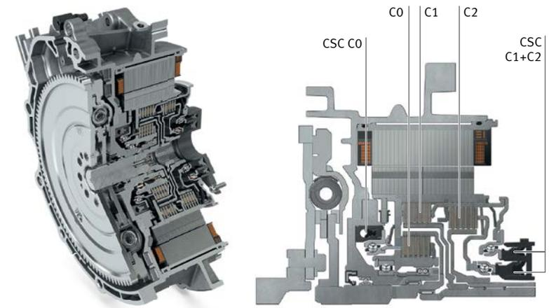
6 P2 hybrid module with a rotor-integrated, wet triple clutch system
