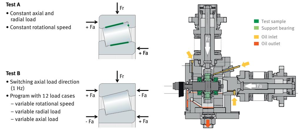
8 General design of the test stand used to validate the rating life calculations for the new ARU bearing design
