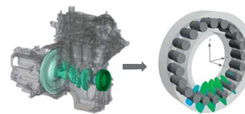
4 Three-cylinder engine with a rolling bearing at the first main bearing position
