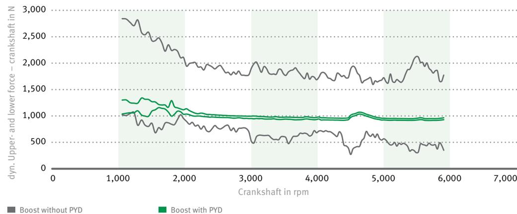
12 Reduction in the bearing forces on the crankshaft pulley by using a crankshaft decoupler
