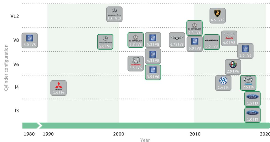
1 Product launch of gasoline engines with cylinder deactivation
