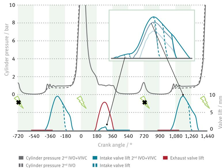
7 Strategies for controlling the residual gas and intake valve lift with the UniAir system for rolling cylinder deactivation
