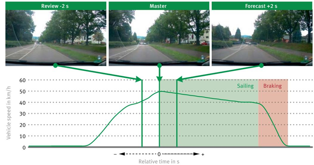
5 Field test on coasting mode: Video material synchronization with measured data
