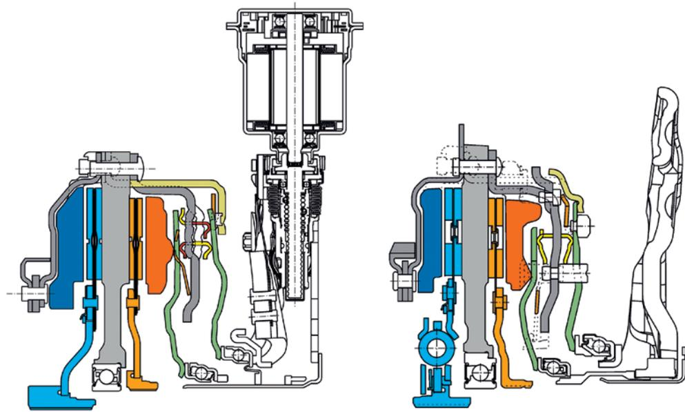
4 Half section of two double clutches with wear adjuster
