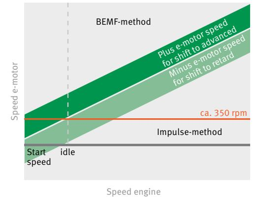
15 The BEMF and pulse method together cover the entire operating speed range of the actuator
