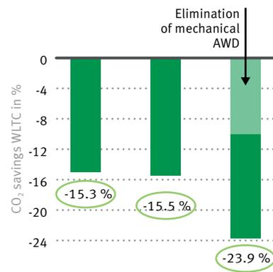
10 Simulated CO<sub>2</sub> savings on a P3 hybrid using a single-speed hybrid module on the transmission output and a P4 hybrid (based on FWD and AWD) with a two-speed electric axle
