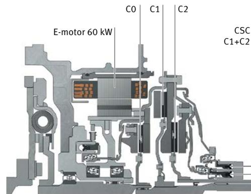
11 Radially nested dry triple clutch
