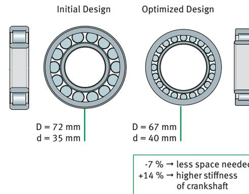
11 Optimally designed rolling bearing for the first crankshaft main bearing in the 1.0-liter three-cylinder engine.
