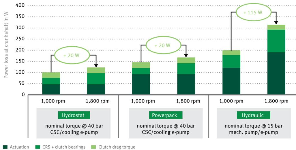
16 Power losses compared to “Hydraulic”, “Power pack” and “Hydrostatic” systems at an average speed of 1,000 rpm and 1,800 rpm in relation to the crankshaft
