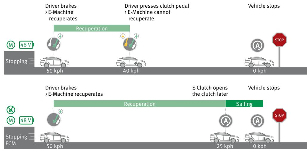
10 Stop from 50 kph without and with an automated clutch
