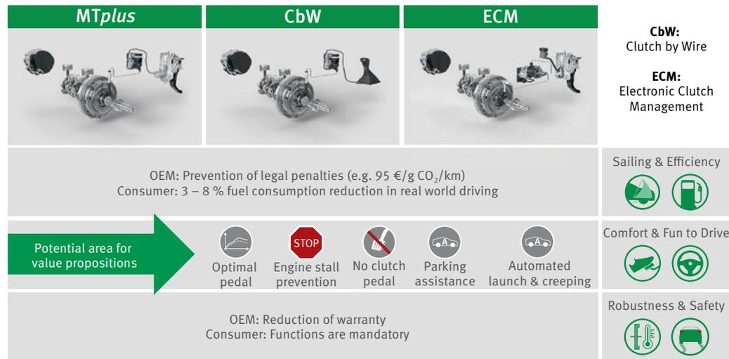
10 Variants for clutch automation: MTplus, clutch-by-wire (CbW) and electronic clutch management (ECM)
