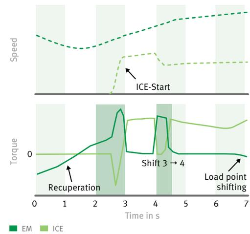
11 Internal combustion engine gear selection and start-up process
