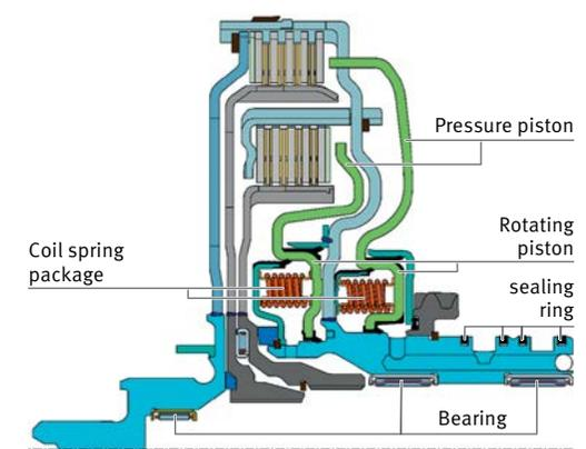
3 Half section of a wet double clutch with rotary feedthroughs and rotating cylinders
