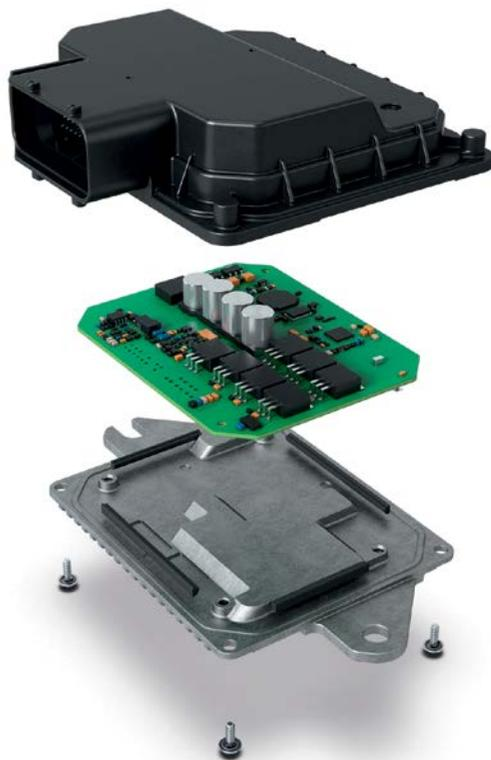
10 Combination of a new printed circuit board and a proven housing concept
