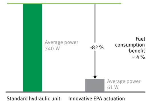
5 Comparison of the of the output requirements of a standard hydraulic unit with EPA actuation technology
