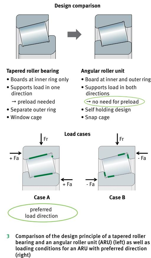
Figure 3 shows Schaeffler's approach with a new locating bearing – the “angular roller unit” (ARU). It has a higher load capacity than a deep groove ball bearing but operates with less friction under axial loads than a cylindrical roller bearing. The ARU can support axial forces in both directions as a self-retaining single bearing. However, it should be mounted in the preferred direction so that the higher axial forces can be transmitted via the raceways, similar to tapered roller bearings.
