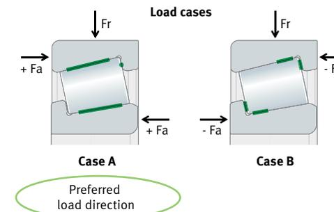
4 Comparison of the design principle of a tapered roller bearing and an angular roller unit (ARU) (left) as well as loading conditions for an ARU with preferred direction (right)
