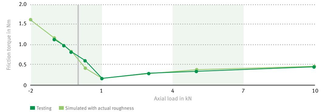
7 Comparison of the simulated friction torque and the friction torque measured on the test stand for the new ARU bearing design
