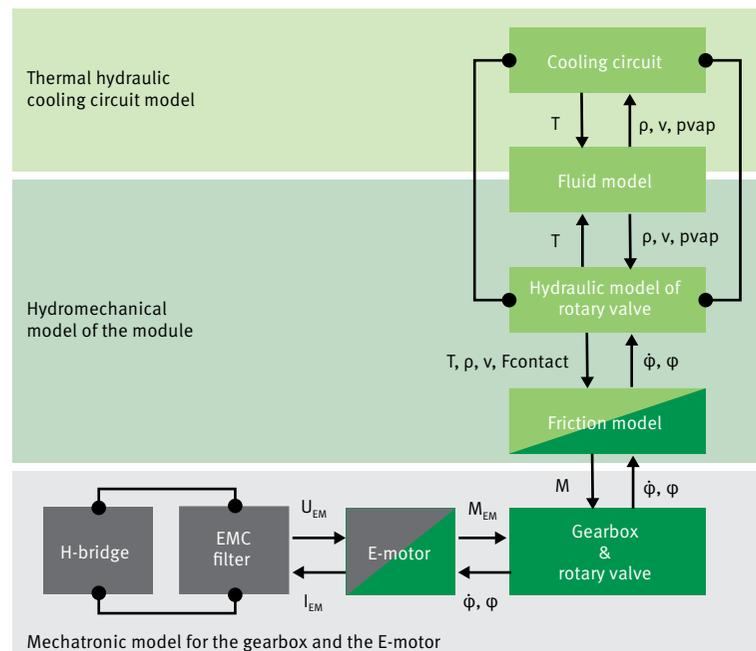
11 Structure of a physical model for designing thermal management
