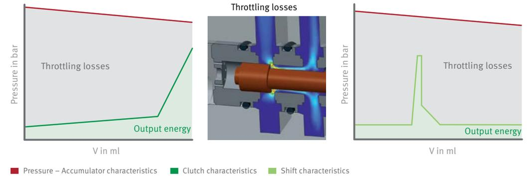
2 Throttling losses on pressure reduction valves of power packs
