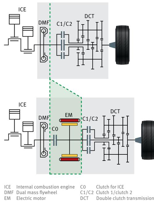
1 Schematic diagram of P2 hybridization in connection with a double clutch transmission
