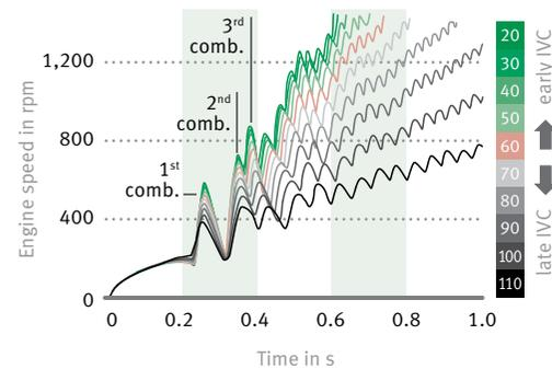
11 Engine speed ramp-up when starting at different phase adjustment angles
