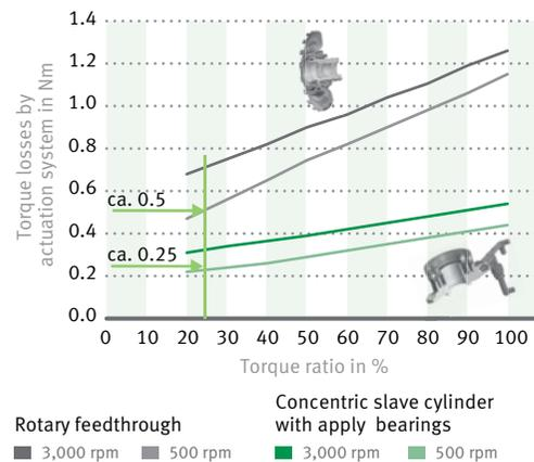
17 Drag loss measurements of engagement bearings and rotary feedthrough
