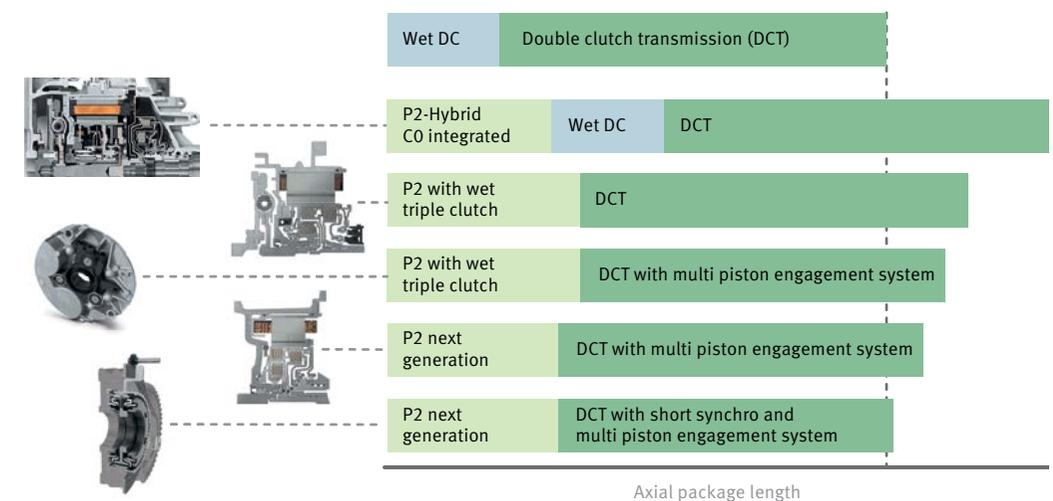
18 Measures for reducing the overall transmission length of P2 hybrid double clutch transmissions
