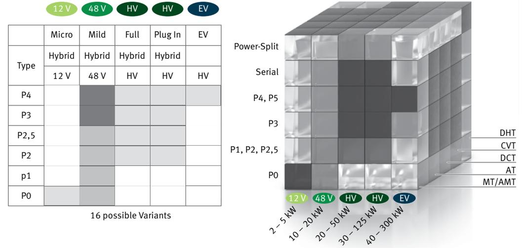
4 Combination of architecture, topology, and transmission options in a hybrid powertrain
