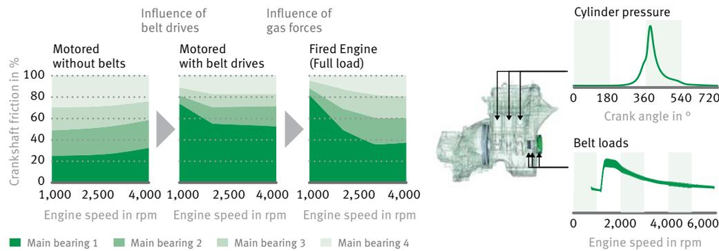
9 Friction percentages of the four crankshaft main bearings and virtual reciprocal effects.
