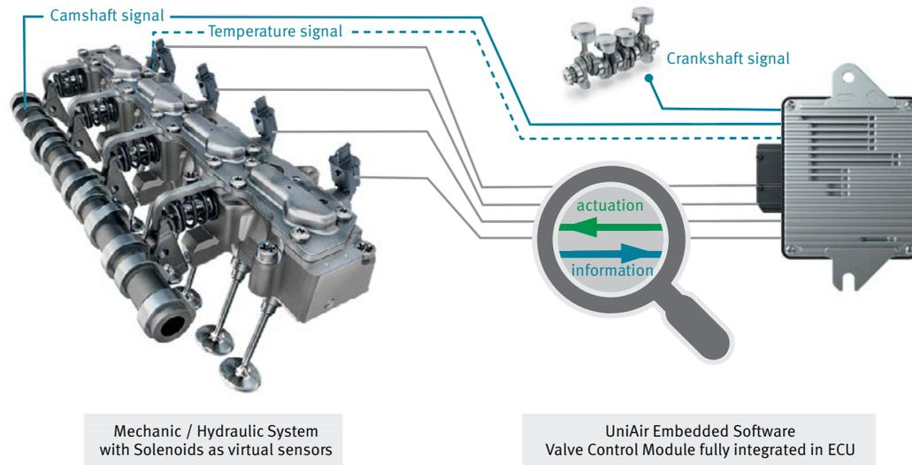
3 Interlinking of actuator technology and engine control unit
