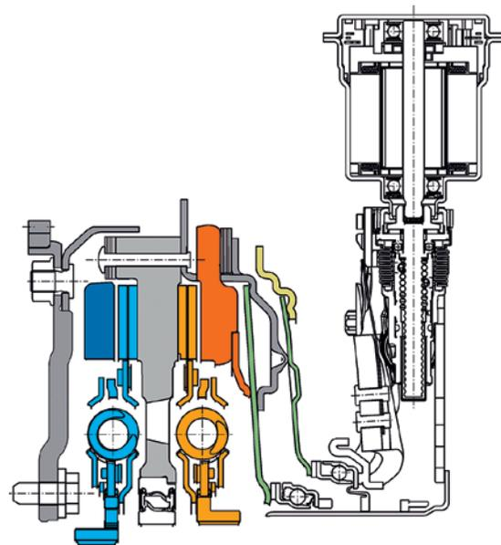
5 Half section of a dry double clutch without wear adjustment
