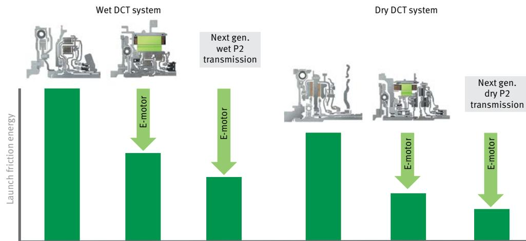
5 Energy needed for vehicle launch with various stages of electrification of wet and dry double clutch transmissions
