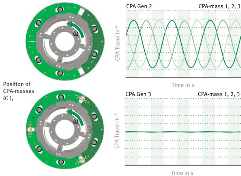
12 Effect of gravity on the pendulum motion in a 1<sup>st</sup> order CPA
