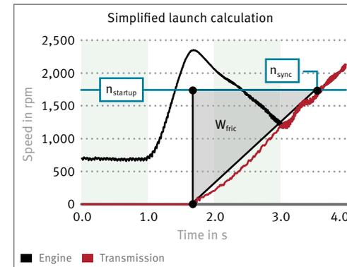
12 Clutch design based on simplified calculation values
