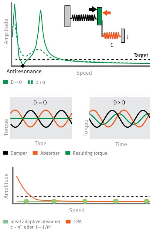
10 Implementation of the anti-resonance principle using the example of a damper
