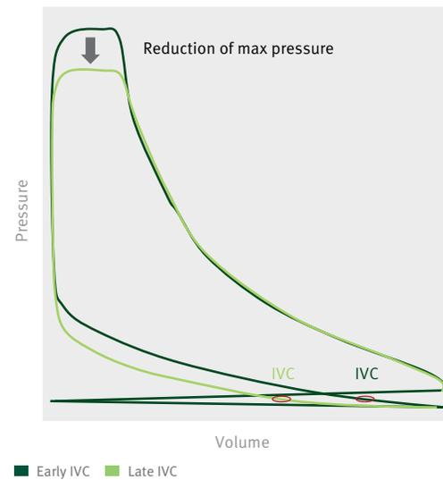
10 The charge cycle as depicted in the schematic PV diagram: When the intake valves execute a delayed close, part of the charge is ejected during compression such that less air is compressed
