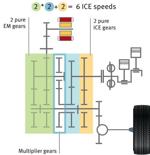
9 Transmission schematic for a hybrid transmission with six combustion engine and two electric gears
