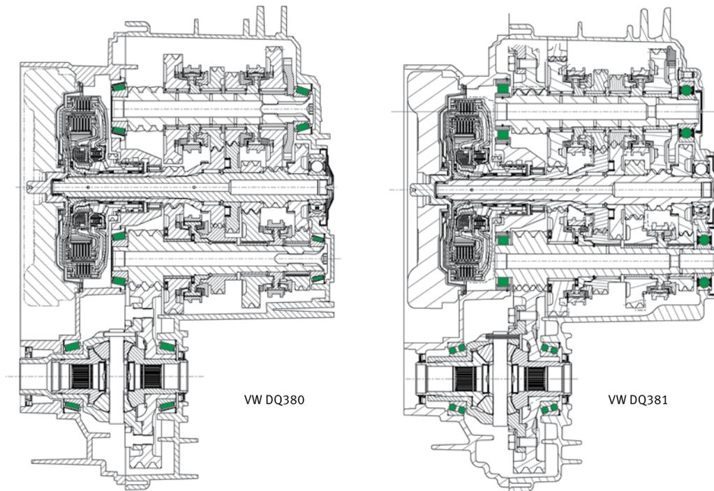
2 Adjusted tapered roller bearing supports (left) versus locating/non-locating bearing supports (right)
