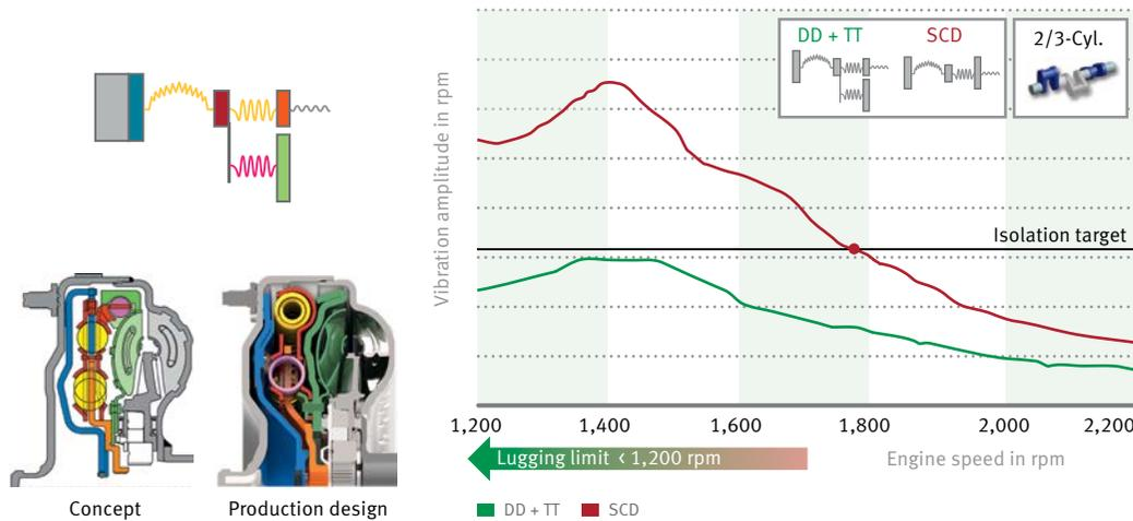
14 Isolation comparison of torsion dampers with and without turbine tilger
