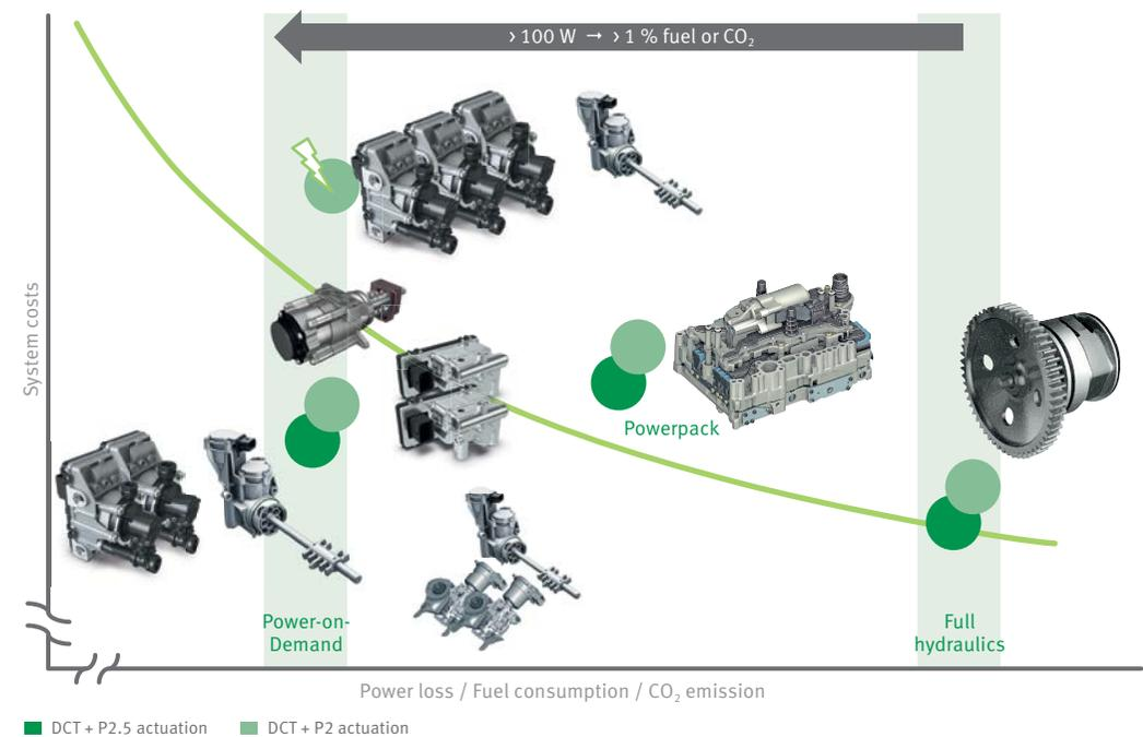
10 Efficiency gains for various actuator systems in relation to system costs for P2.5 and P2 double clutch transmissions
