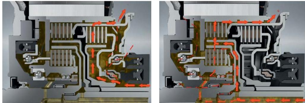
7 Oil flow inside of the rotor for the sub-clutches and the bearing positions
