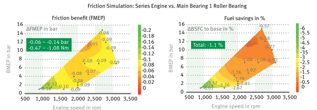
12 The reduced friction attributed to the first crankshaft bearing fitted as a rolling bearing averages out to 1.1 % less fuel consumption in the WLTC.
