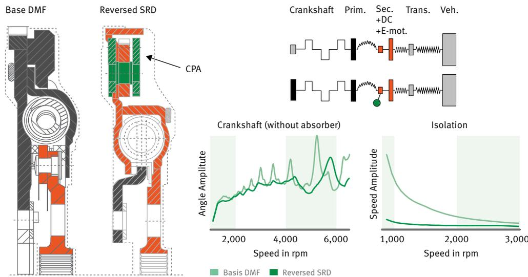
8 Reversed small radial damper (RSRD) with CPA and flywheel on front end of the crankshaft
