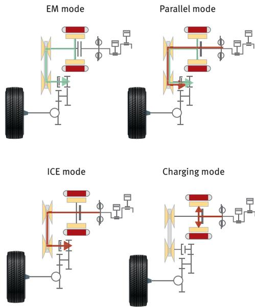
3 Operating modes of the DH CVT with electric reverse gear
