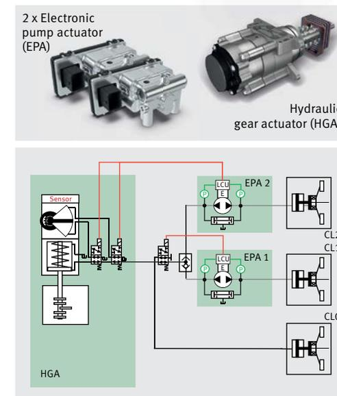
7 Actuator system for double clutch transmissions with two EPA and one HGA
