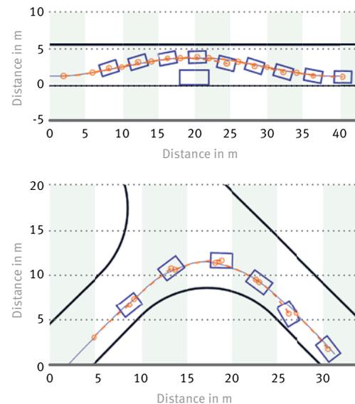
12 Vehicle behavior during emergency braking due to total system failure
