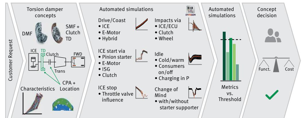
2 Optimization process for the design of modern torsional vibration dampers
