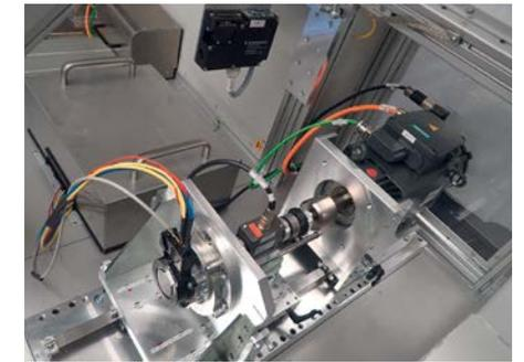
8 VCR BLDC motor prototype and test stand for component testing
