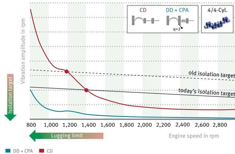
8 Isolation comparison of torsion dampers with and without a CPA
