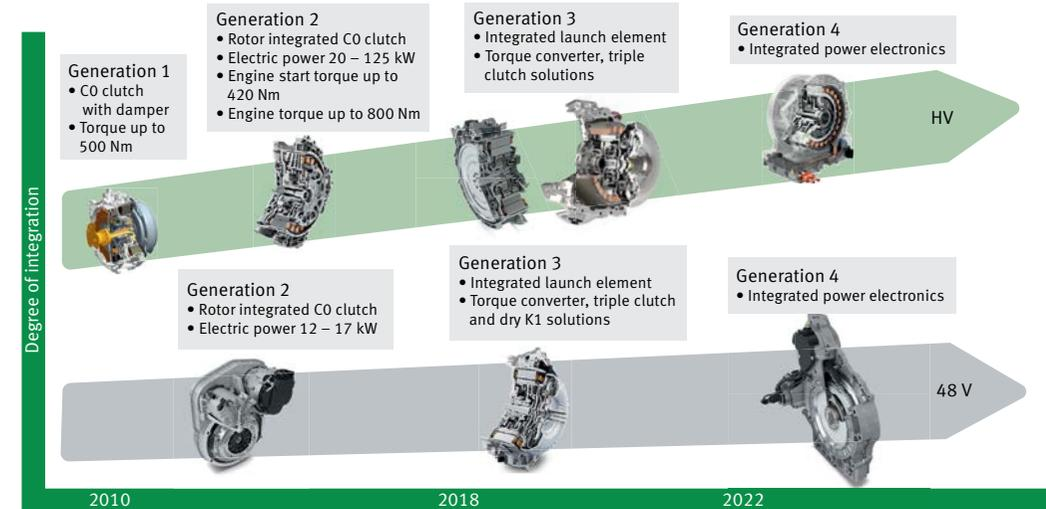
10 Evolutionary phases for the Schaeffler modular system for P2 hybrid module
