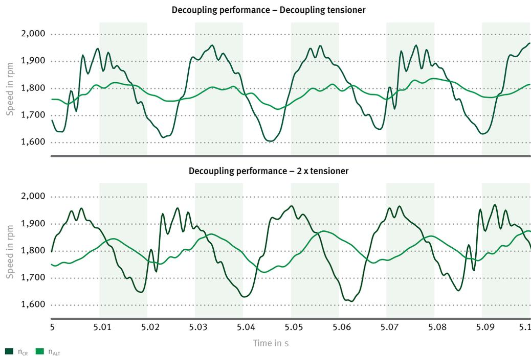
3 Decoupling function of a P0 system, based on two individual tensioners (above), compared to a P0 system with a decoupling tensioner. Graphed here are speeds over time during generator operation; the BSG speed is converted to the crankshaft
