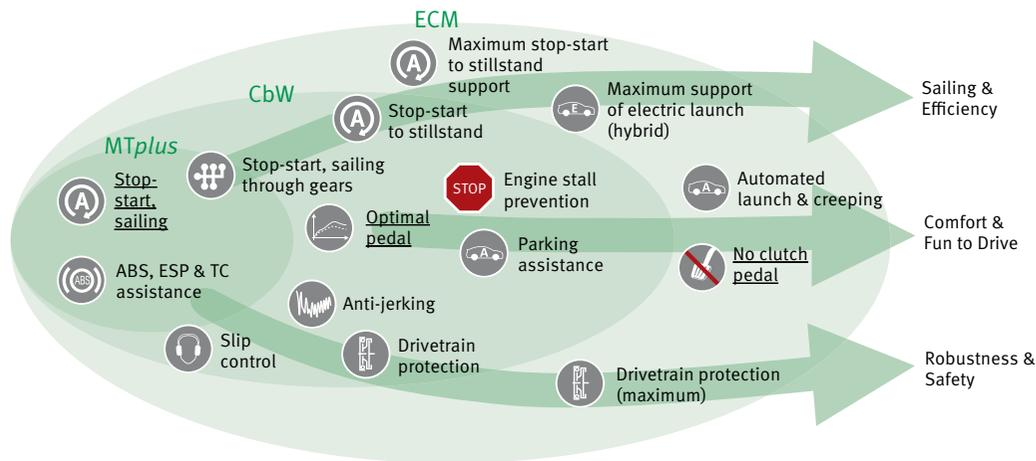
4 Functions of the automated clutch in the MTplus, CbW and ECM variant
