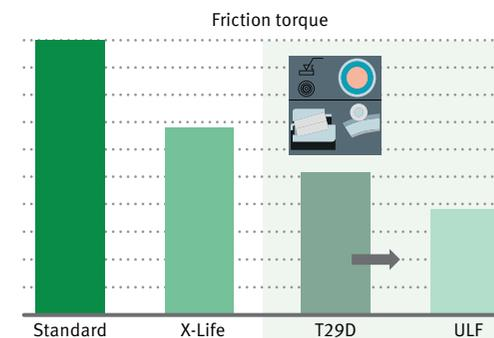
1 Comparison of ultra low friction tapered roller bearings
