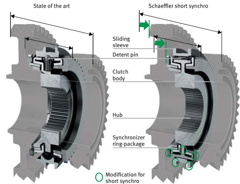
16 Optimizing installation space by using shorter synchronization units, taking the Schaeffler Short Synchro as an example
