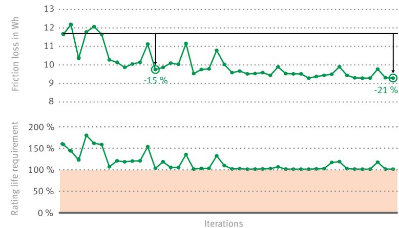
9 Curve of the determined friction energy and service life evaluation based on optimization Both values are calculated using different design cycles that represent the respective target requirements
