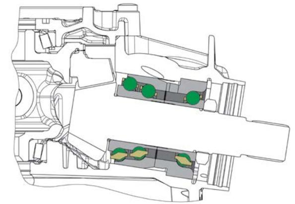
13 Integration of bearing systems using a bearing cartridge for a hypoid drive as an example
