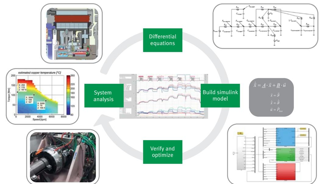
6 Continuous development of a thermal model for tractive motors
