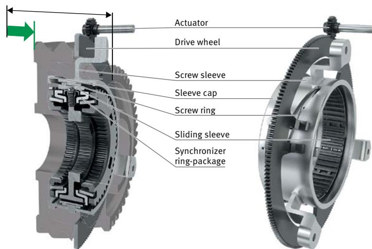
17 Synchronization unit with a rotary actuation under the gearwheels (Schaeffler Ultra Short Synchro)
