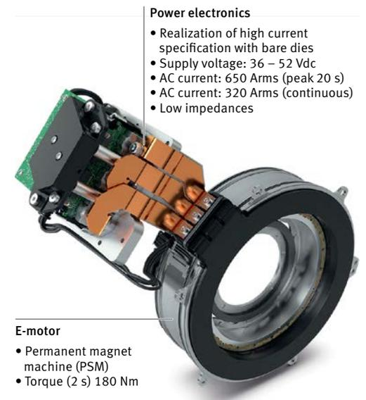
11 Integration of the power electronics in a P2 hybrid module at the 48-volt level
