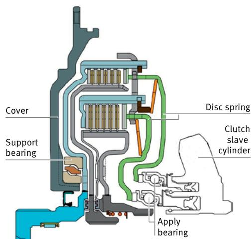
1 Half section of a wet double clutch with actuation bearings
