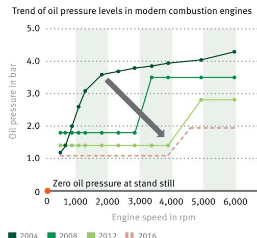
2 Oil pressure of different generations of an engine family from 2004 (dark green) to 2016 (light red)
