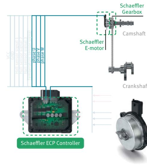
14 Simplified electromechanical camshaft phasing unit concept without engine-integrated sensor system
