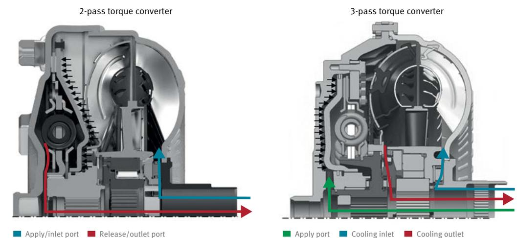
1 Comparison of a two-pass and a three-pass converter
