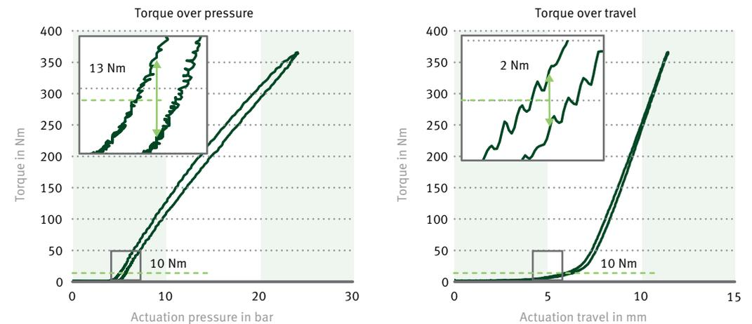
12 Torque characteristics of leakage-free systems with regard to controllability of the touch point
