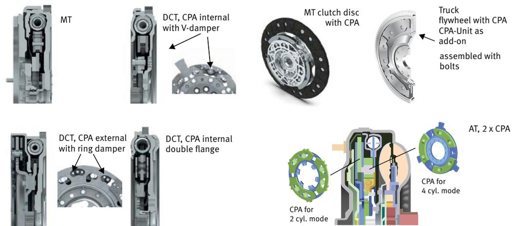
2 Applications for the centrifugal pendulum-type absorber in the DMF (left) and other applications (right) on the clutch disk, in the single mass flywheel and as a double CPA in an automatic transmission converter
