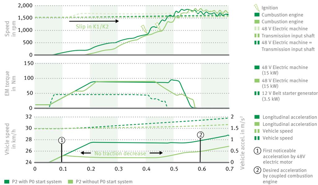
12 Simulation of a restart from electric driving with a 48 V P2 hybrid with and without additional starter system
