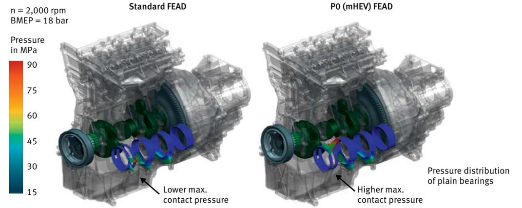
14 The load exerted on the first crankshaft main bearing can be very high, particularly on a P0 hybrid, which means that a rolling bearing mount can measurably reduce fuel consumption.
