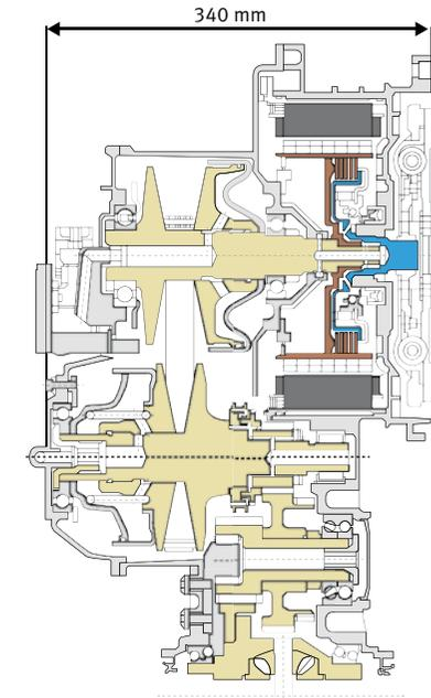
4 Cross-section and construction of the DH CVT
