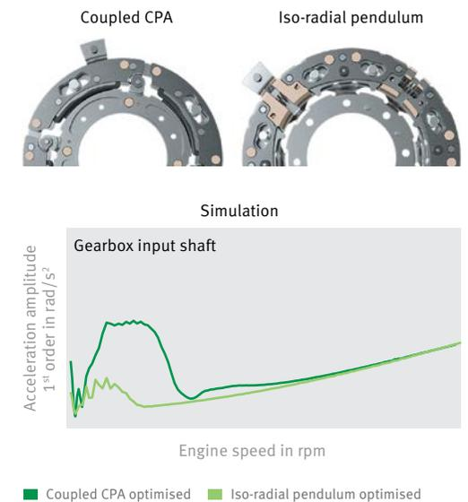
5 Couple pendulum and iso-radial pendulum (top) with a diagram of vibration amplitudes in relation to the speed (bottom)
