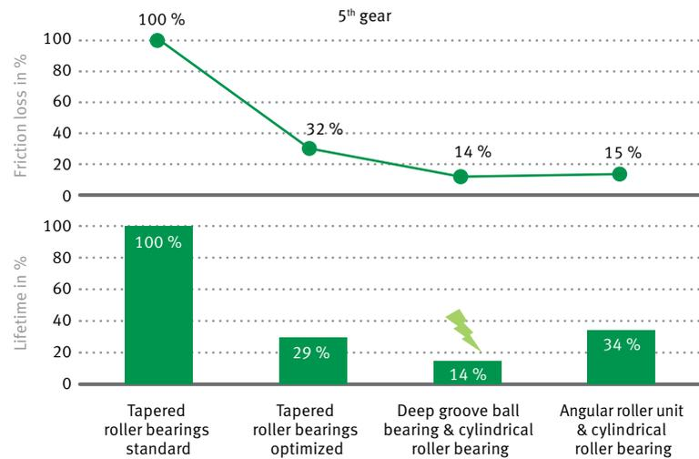
6 Simulation of friction (top) and rating life (bottom) for the 5<sup>th</sup> gear of a manual transmission
