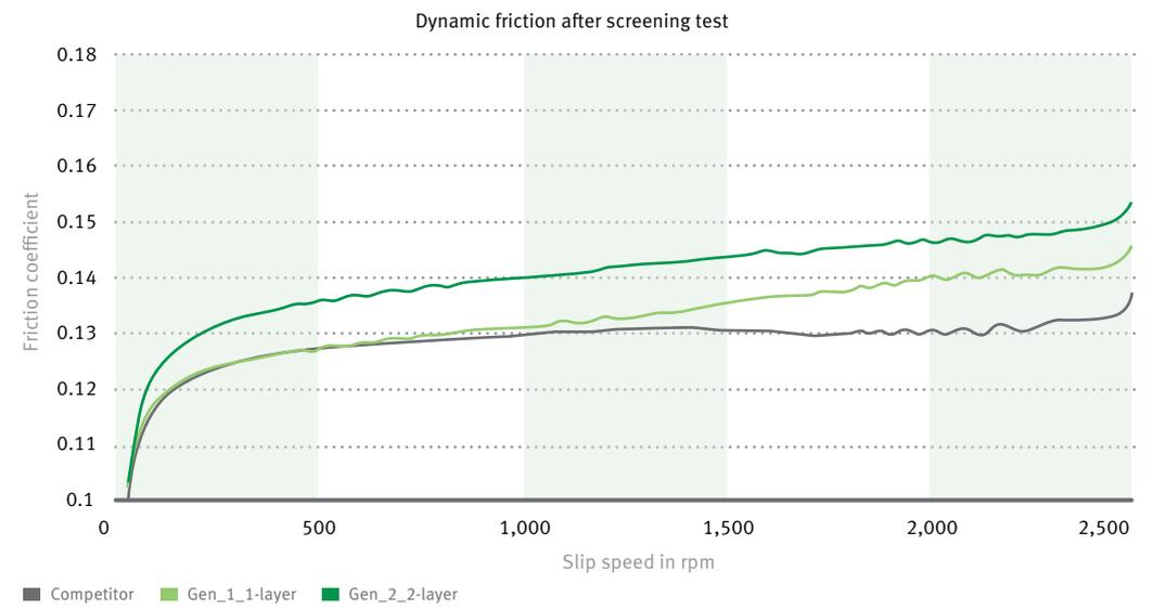
9 Comparison of dynamic friction coefficients of the one-layer and two-layer Schaeffler friction lining after 15,000 uphill starts at full load.
