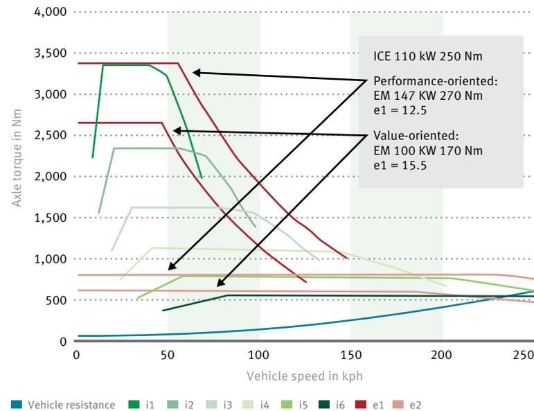
10 Axle torque as a function of the driving speed for two variants of the electric motor (147 and 100 kW) as well as two different ratio stages in the electric gears
