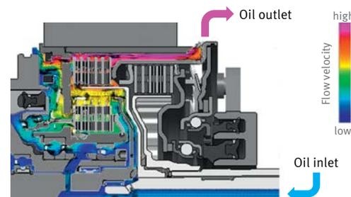
8 Flow simulation for a P2 hybrid module with an integrated wet triple clutch
