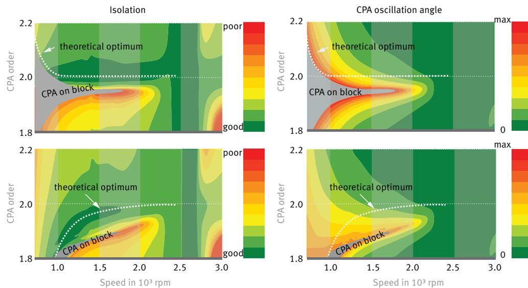
3 Basic simulation for optimization of the guide track curvature of the pendulum and the flange in combination with the roller diameter using the example of an CPA without (top) and with (bottom) spring elements between the pendulums (couple pendulum).
