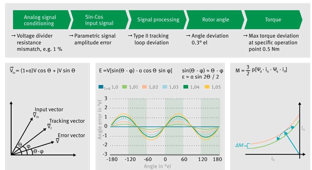
14 Propagation of torque generation inaccuracies in a typical e-machine
