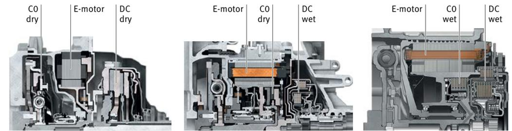
2 Implemented series solutions for P2 hybridization of double clutch transmissions
