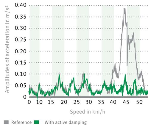
13 Vibration reduction in a wheel-hub drive through targeted torque variation in the e-machine
