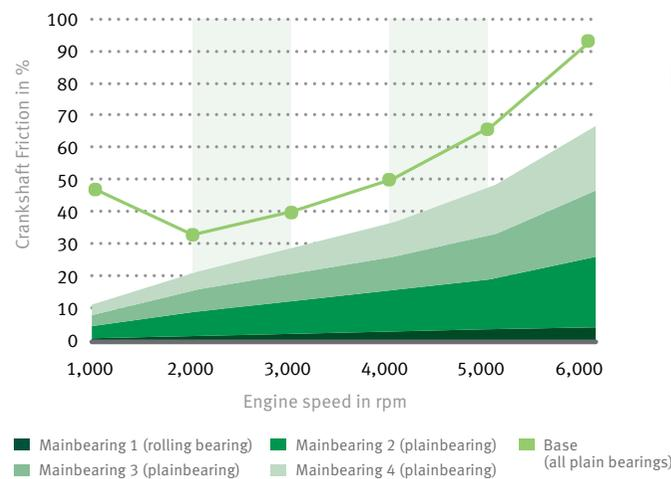
10 Potential for reducing friction using rolling bearings.
