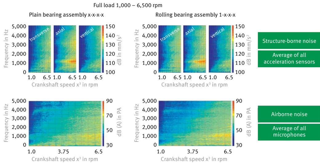
13 The subjective analyses revealed that there was no perceptible difference in NVH performance between the engine when fitted with rolling and with plain bearings.
