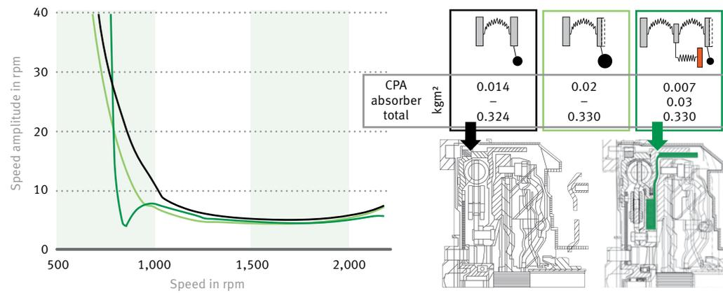
13 Placing a damper on an intermediate flange to utilize anti-resonance
