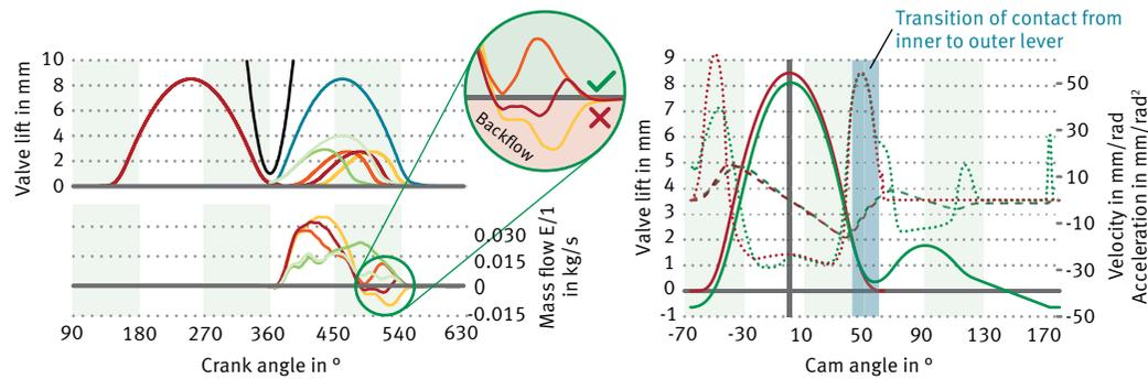
10 Intake backflow (left) and transfer of contact from main to secondary lift (right)
