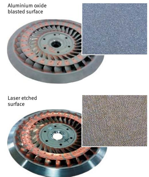
7 RepARATION of adhesive surface by laser etching
