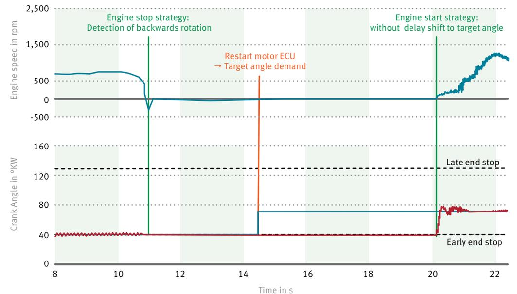
9 Adjusting the camshaft at engine start-up
