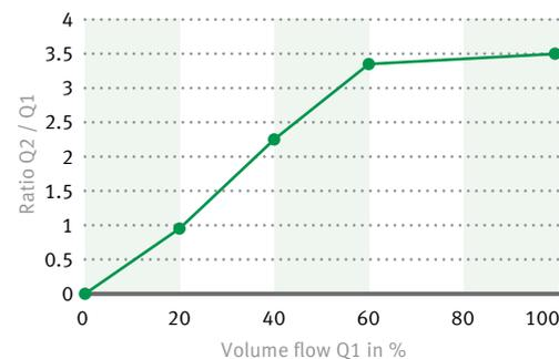
19 Ejector pump including measurement of the amplification factor of the volume flow
