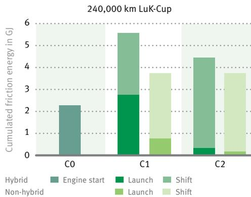
4 Friction energy of the clutches for double clutch transmissions, with and without P2 hybridization
