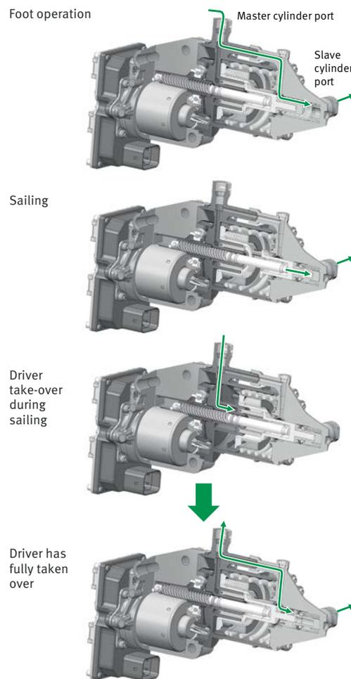
2 Operating conditions of the actuator: Clutch actuation by driver and pedal, actuation by actuator only when coasting and return to actuation by the driver
