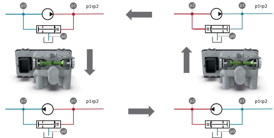
12 Operating principle of the two-pressure valve in the EPA
