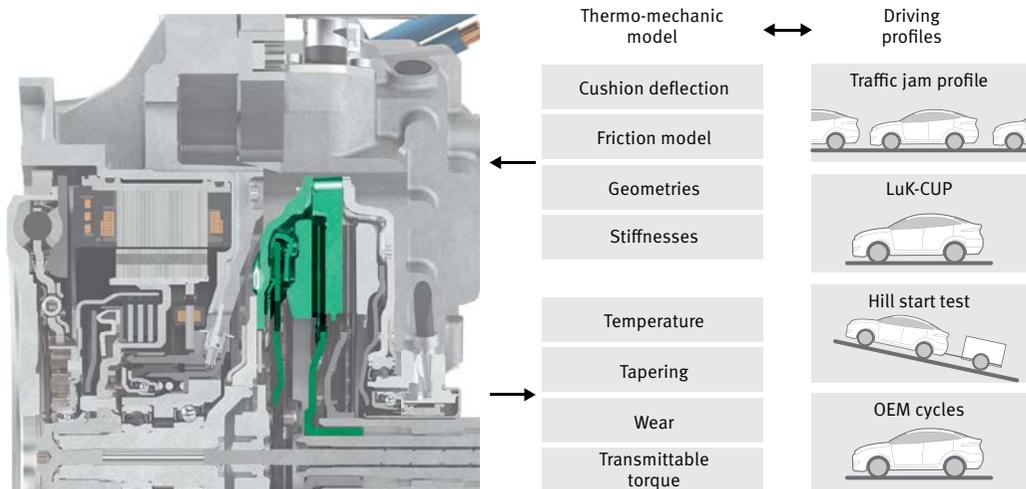
16 Development and safeguarding of complex clutch systems by including thermal-mechanical effects
