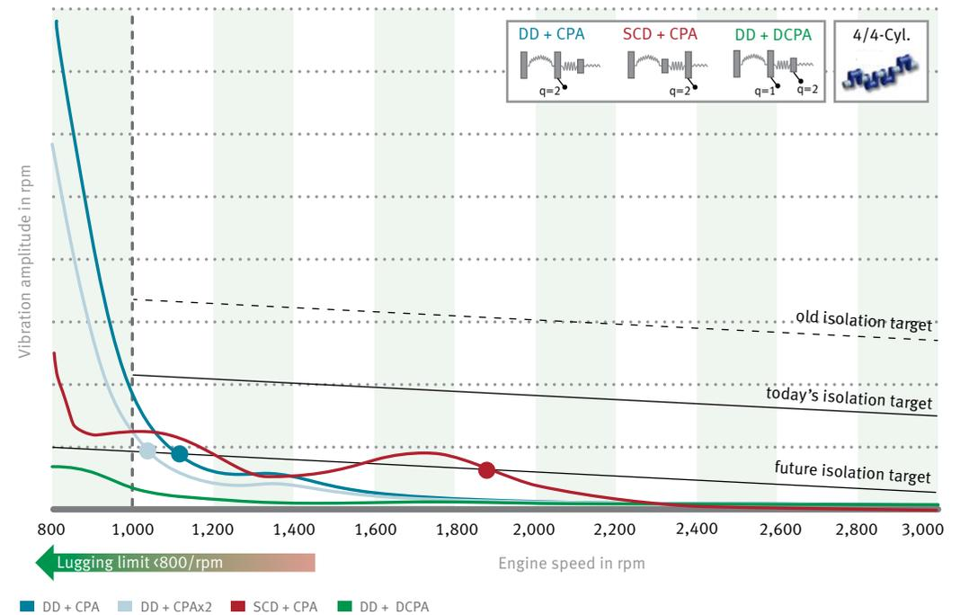
9 Isolation comparison of torsion dampers with CPA and double CPA
