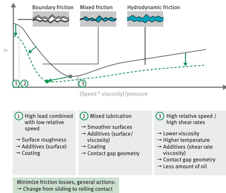
1 Stribeck curve with static friction, mixed friction and viscous friction.
