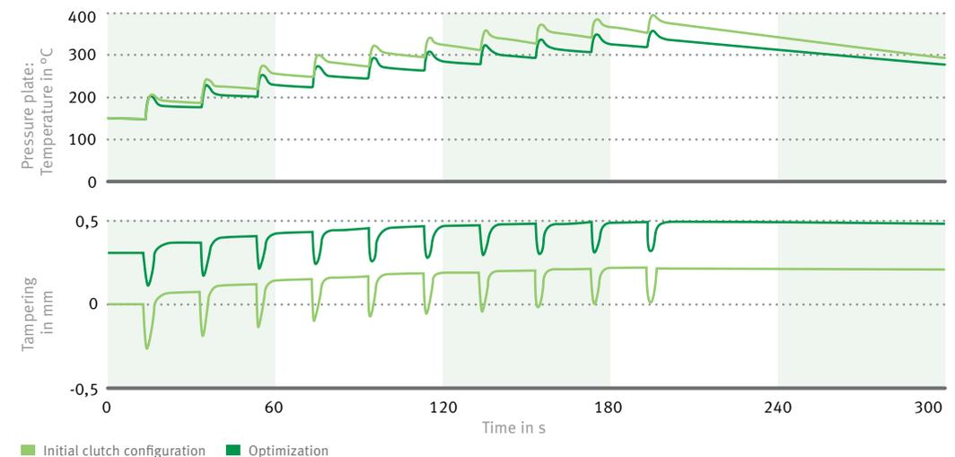
15 Excerpt from uphill start simulation with the thermal-mechanical model
