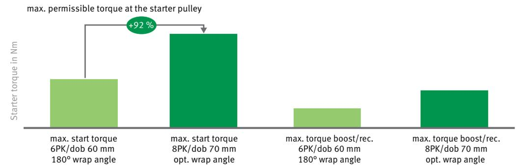
7 Torque limits of the e-machine due to the maximum admissible belt forces, depending on the belt width, BSG diameter, and wrap angle.
