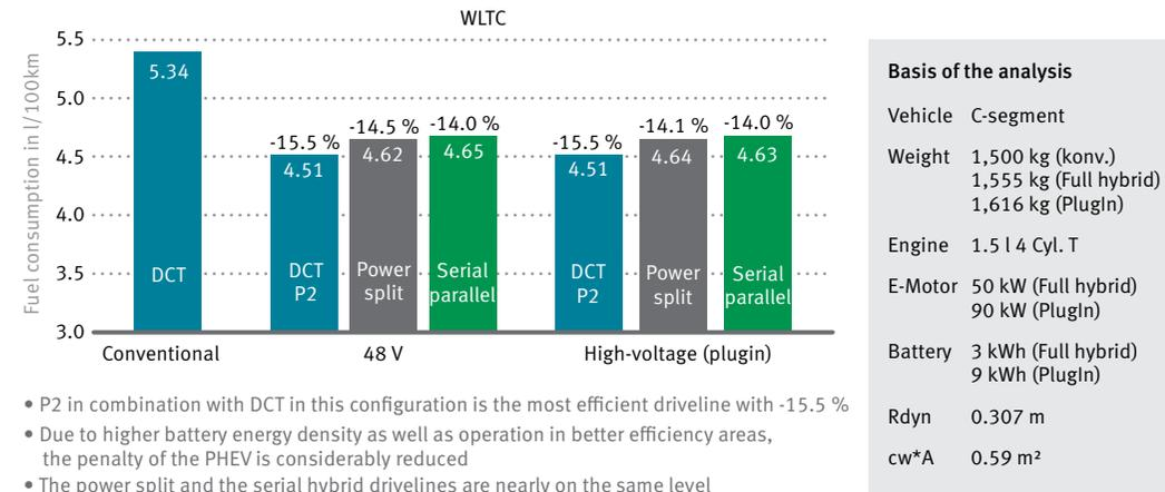
2 Simulated fuel consumption for various high-voltage hybrid systems in the WLTC
