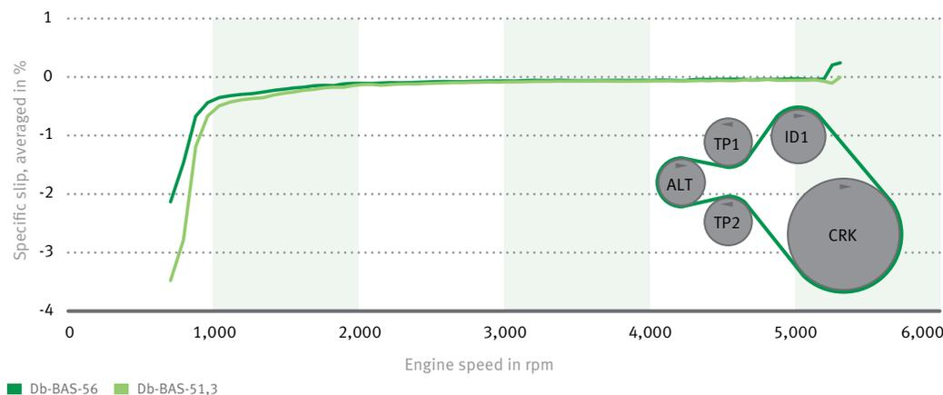
6 Simulation of a P0 48V system during boost operation: Average belt slippage at the belt pulley on the generator side for two pulleys 51.3 mm (light-green characteristic curve) and 56.0 mm (green characteristic curve) in diameter.
