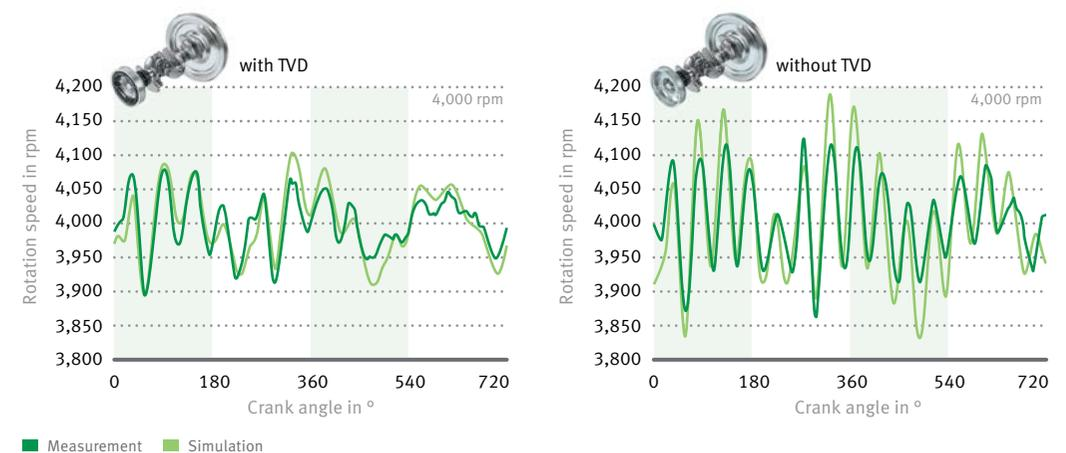
6 The measurements and engine model calculations showed a high level of congruence both with and without the vibration damper.
