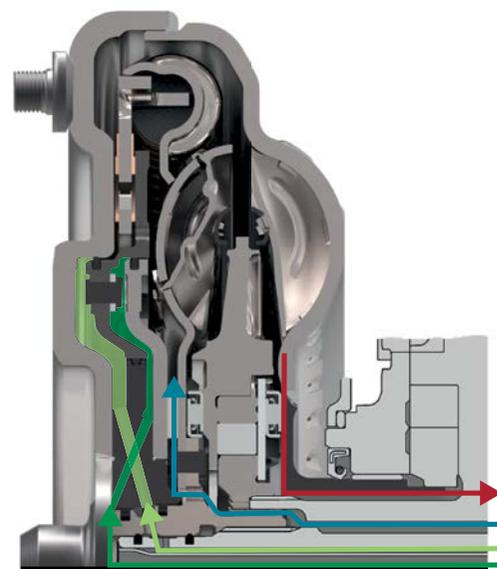
2 Design of the four-pass torque converter
