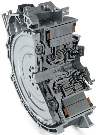
6 Cross-section through the complete oil-cooled hybrid module with integral triple clutch
