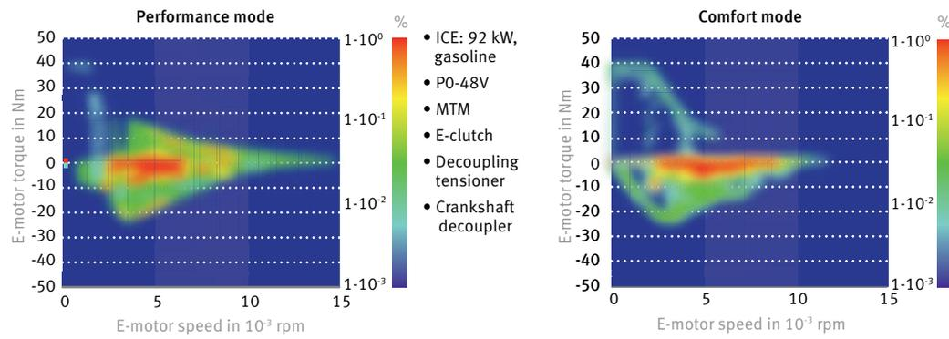
17 Time-weighted occurrence of various loads in the P0 drive over the electric motor speed for two operating strategies: histogram analysis in sport mode on the left and in comfort mode on the right
