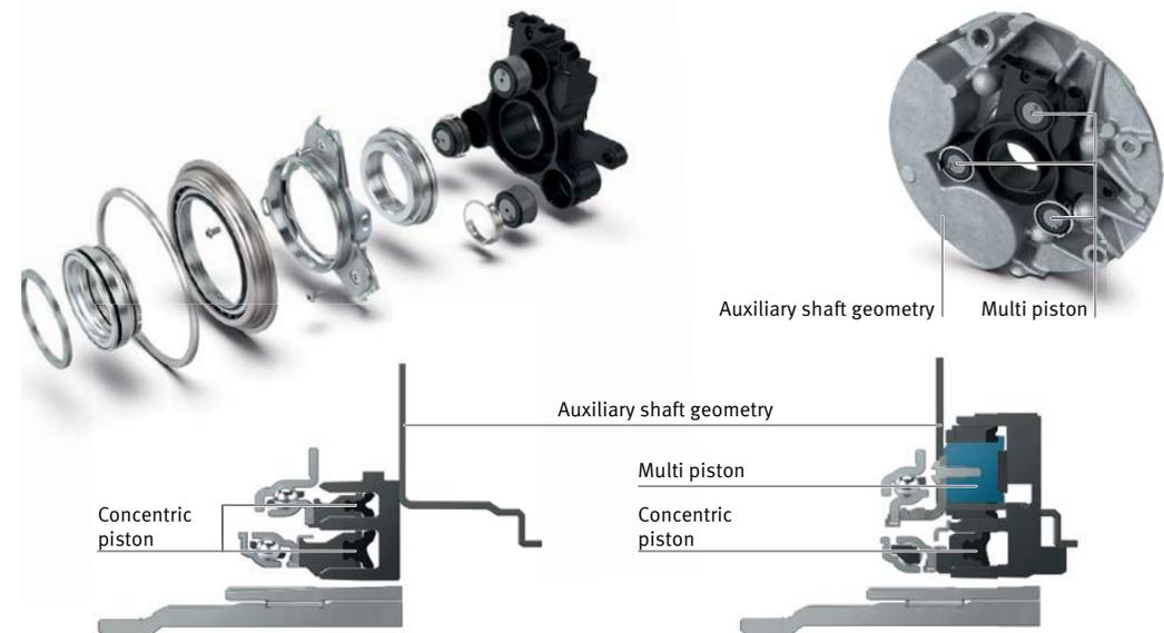
13 Further development of the double actuator system for C1 and C2 (3-piston actuator system)
