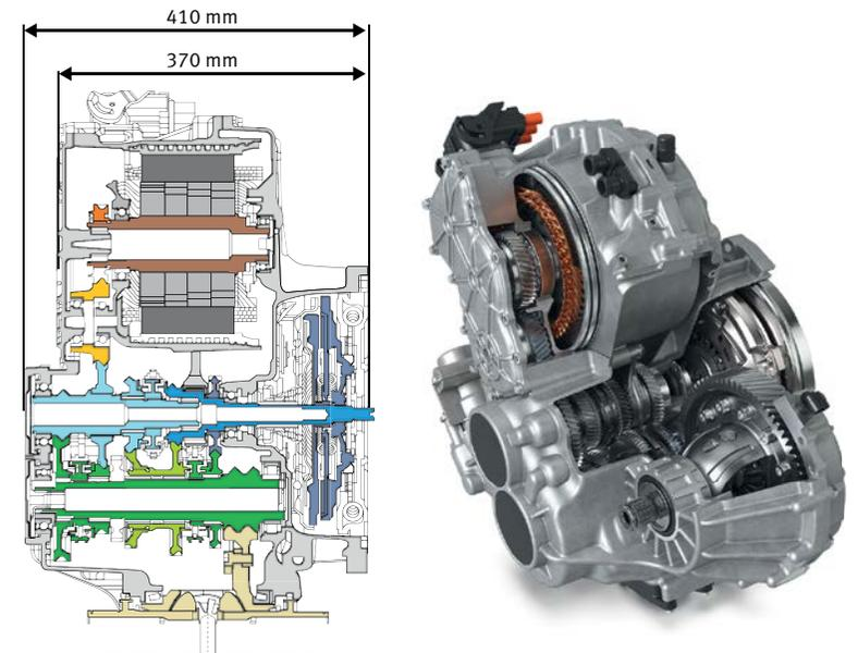
8 Cross-section and design of the DH ST 6+2 with six combustion engine and two electric gears
