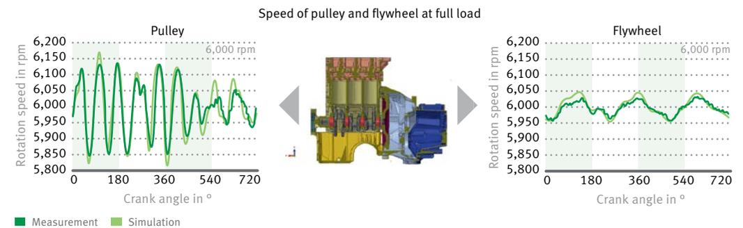
5 The comparison between the physical engine and the engine model reveals close conformity with the crank angle resolved speed.
