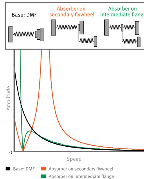
12 Operating principle of the damper on the intermediate flange: Achievement of an anti-resonance without interfering resonance in a higher speed range
