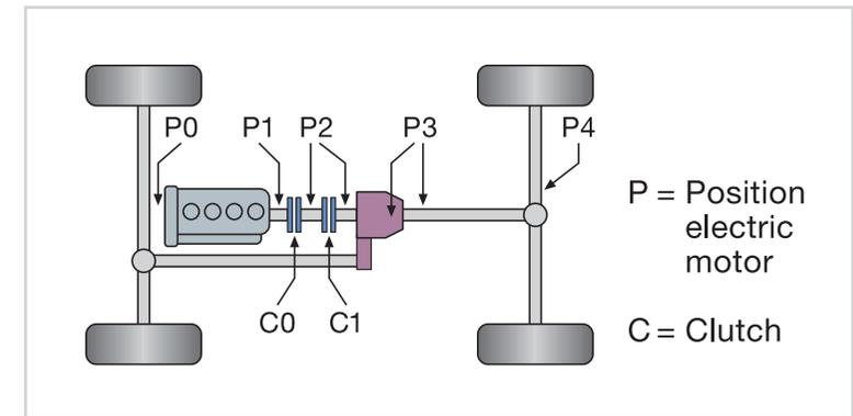
Figure 11 Possible installation positions of electric motors
