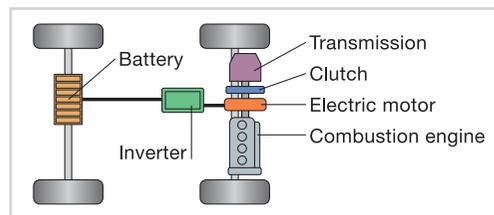
Figure 1 Principle mild hybrid
