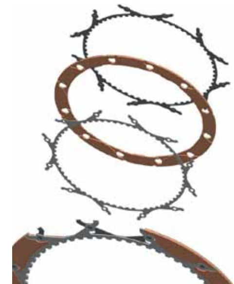
Figure 11 Composite friction Disk construction
