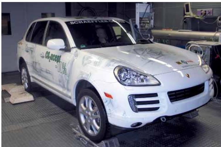
Figure 18 Measurements taken with the vehicle on the rolling test stand
