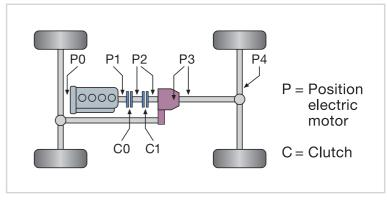
Figure 11 Possible installation positions of electric motors
