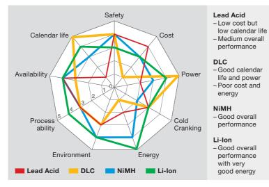
Figure 6 Comparison of different battery systems for automotive application
