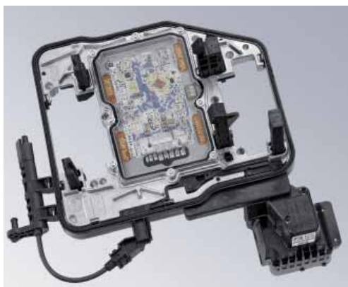
Figure 11 Electromechanical transmission control system
