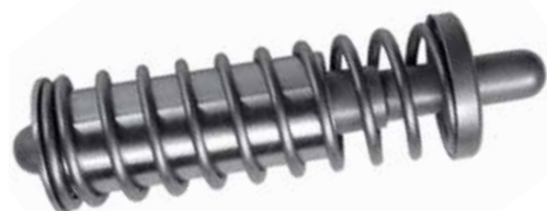
Figure 1 First hydraulic chain tensioner
