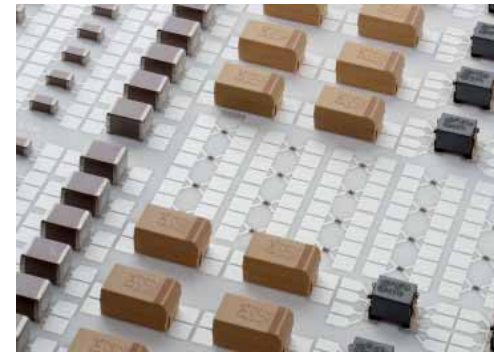
Figure 8 Test substrate for conductive adhesive interconnections of new component shapes for use in transmission controls (detail)
