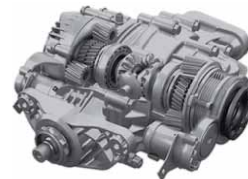
Figure 1 Rear axle differential of the BMW X6
