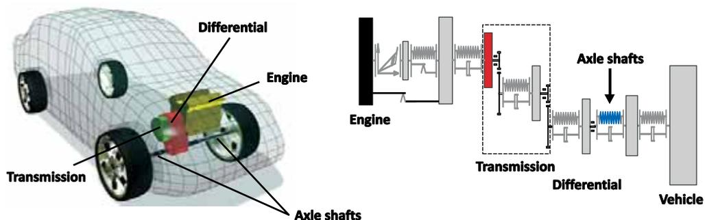
Figure 10 Taking the entire drive train into consideration to reduce torsional vibrations
