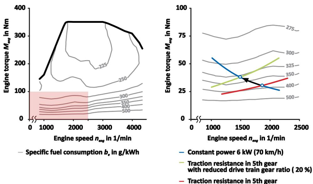
Figure 4 Consumption characteristic map for a 2.0-liter diesel engine – potential consumption reduction due to lowering engine speeds (downspeeding)
