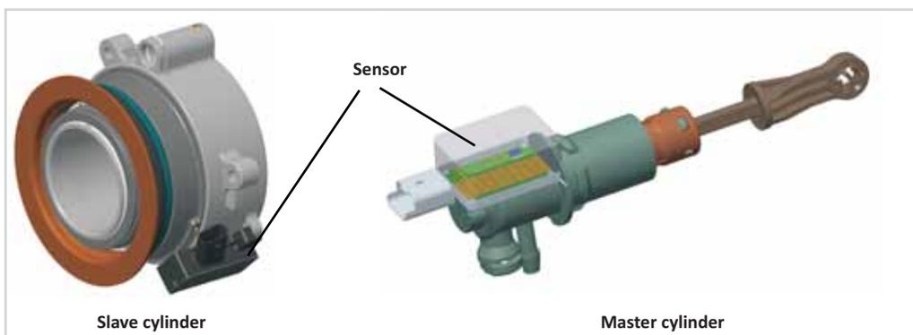
Figure 16 Travel sensors in the release system – not only for stop-start systems
