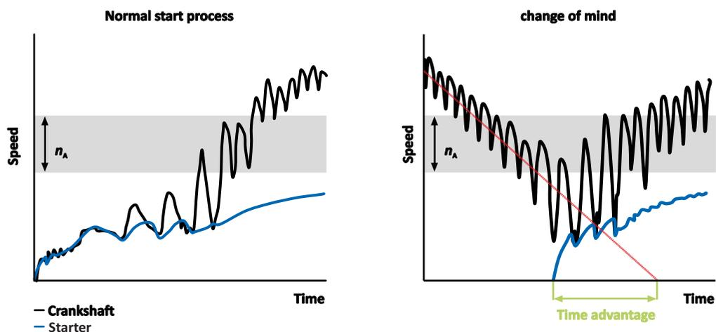
Figure 17 Normal start and restart of a still-running engine (change-of-mind)
