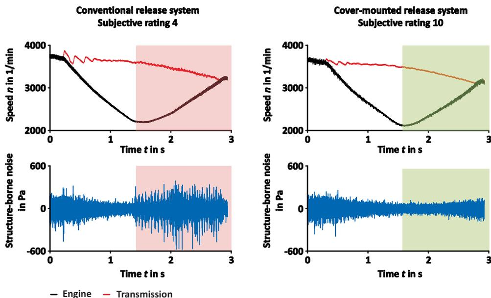
Figure 22 Rattling noise in the slip phase – effectiveness of the cover-mounted release system (CMR)
