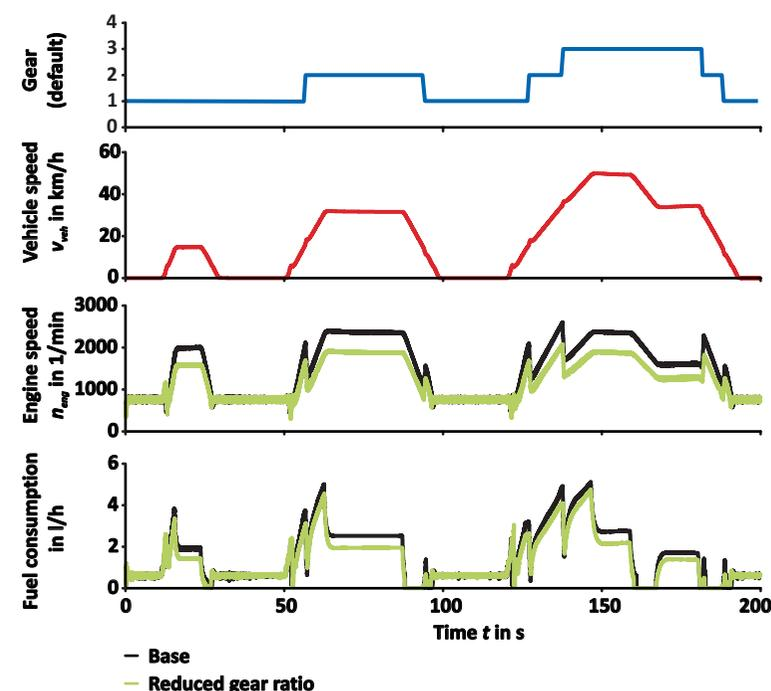
Figure 5 Effects of downspeeding in the NEDC – consumption simulation (city cycle)
