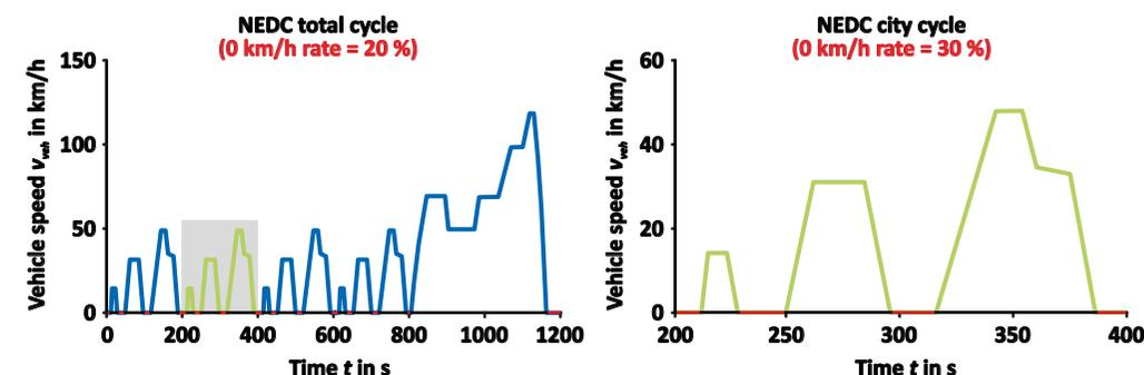
Figure 15 Consumption reduction potential of a stop-start system in NEDC
