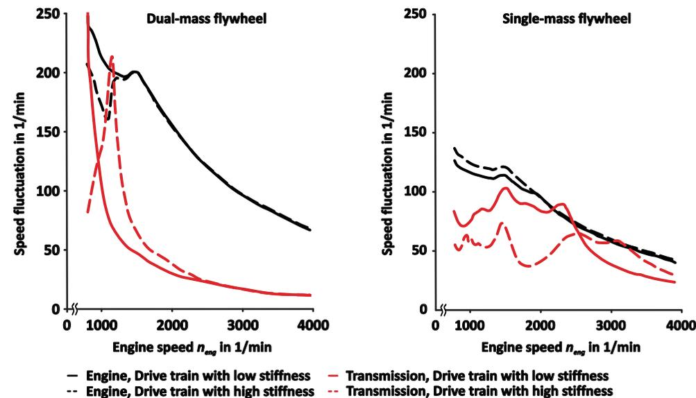
Figure 11 Performance limits of torsional vibration dampers in the entire drive train
