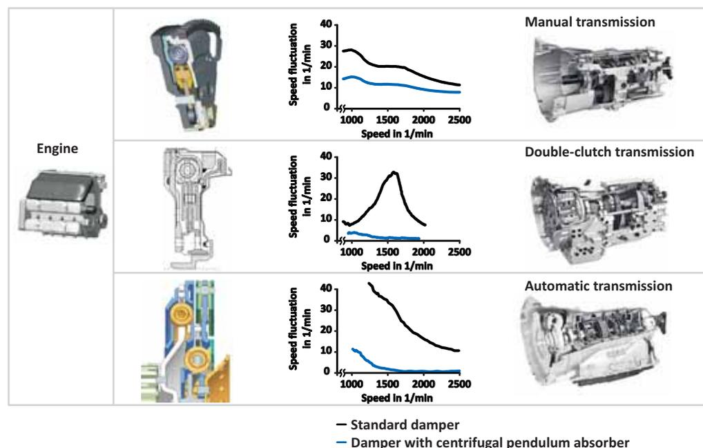
Figure 7 LuK CPA – the standard for torsional vibration isolation in all transmission types
