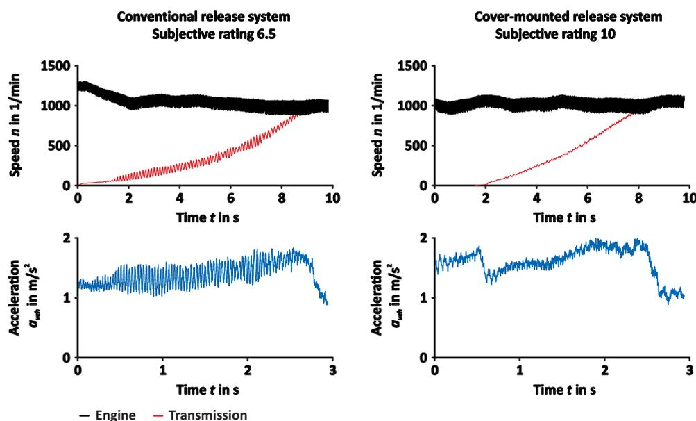
Figure 23 Crankshaft-excited slip – effectiveness of a cover-mounted release system (CMR)
