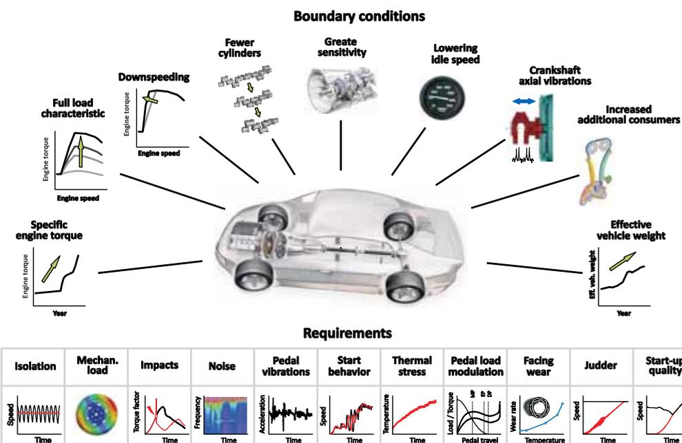
Figure 21 Tightened boundary conditions and requirements for a clutch system
