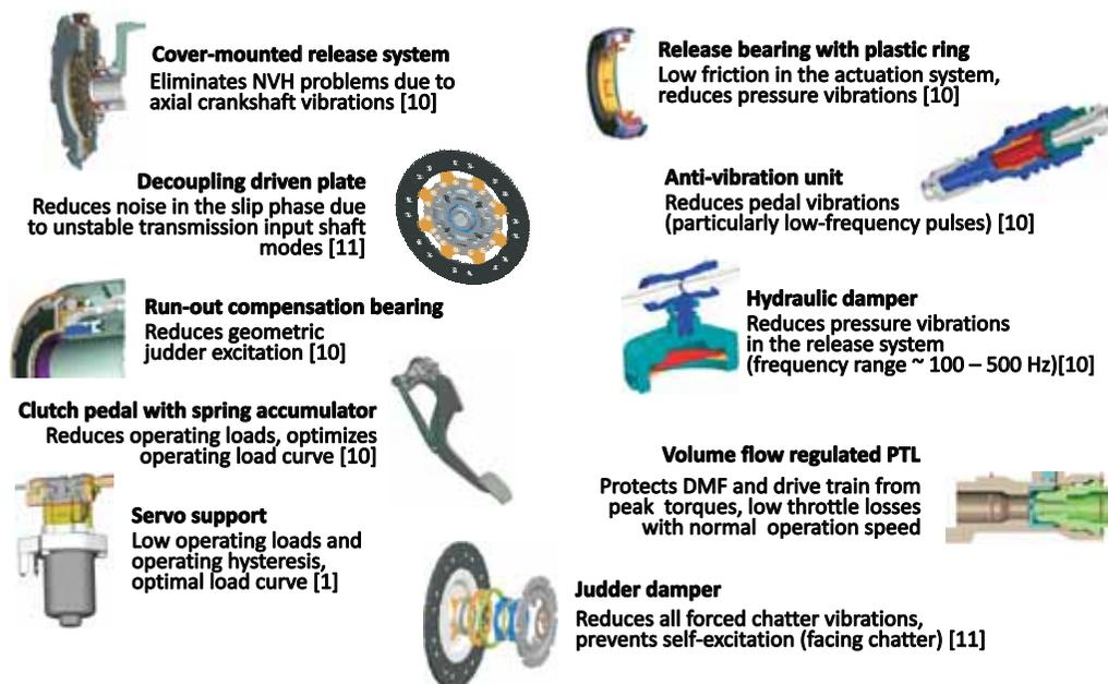
Figure 26 Examples of efficient products to optimize the system behavior in the slip phase
