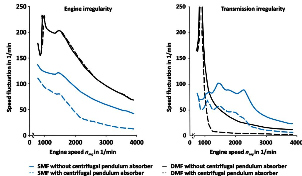
Figure 12 Isolation potential of alternative damper types for 3-cylinder engines
