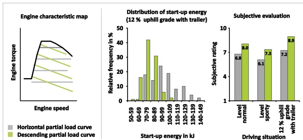
Figure 20 Effect of engine characteristic map on start-up stability – driving test with 10 testers
