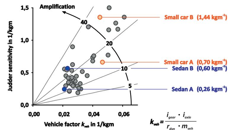
Figure 24 Benchmark slip sensitivity of automobiles in 1st gear
