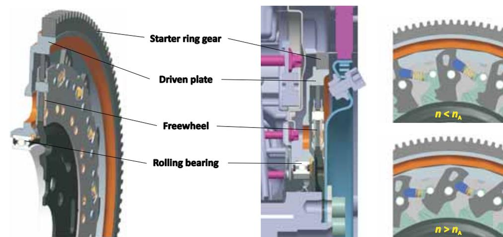
Figure 19 LuK freewheel concept for PES (permanently engaged starter)
