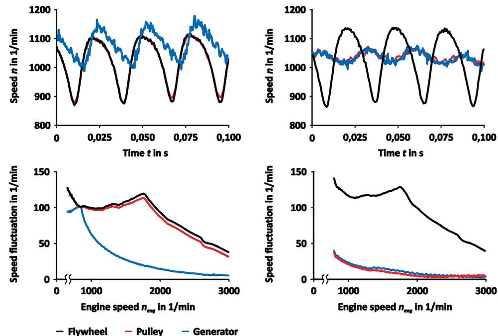
Figure 14 LuK belt pulley decoupler (right) – compared with a conventional generator freewheel (left)
