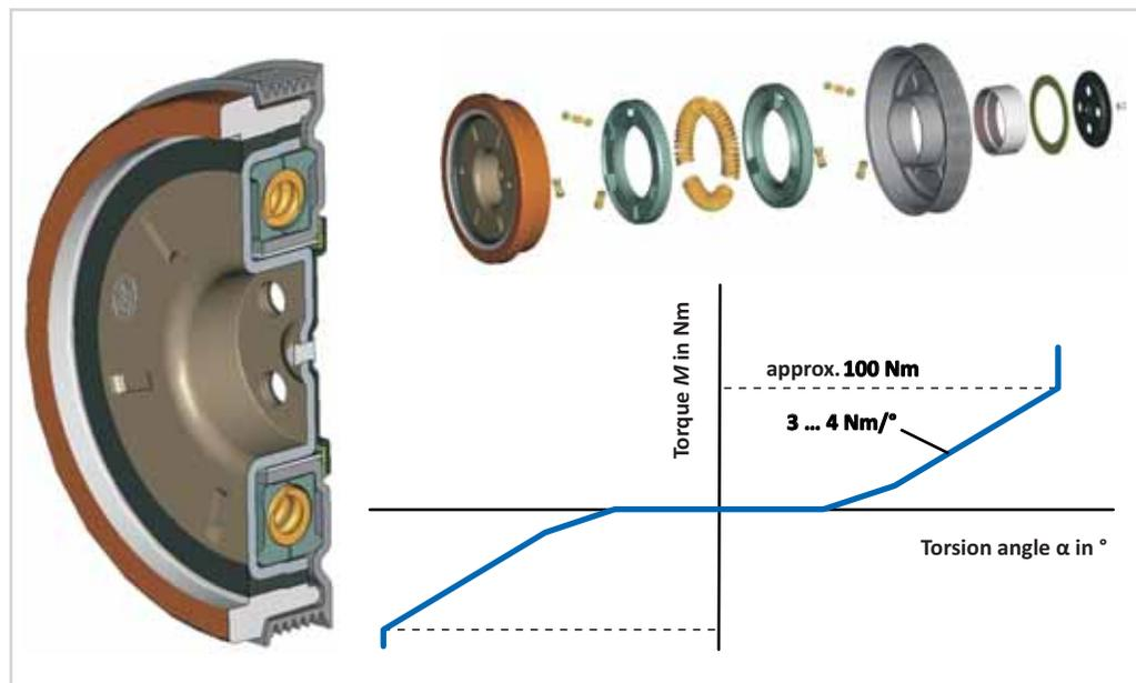
Figure 13 LuK belt pulley decoupler (BPD) – the DMF for the power take-off
