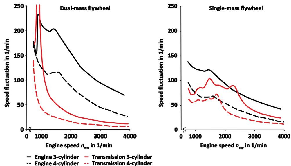
Figure 9 Increasing requirements when reducing the number of cylinders – Example: 3 cylinders instead of 4, with the same maximum engine torque
