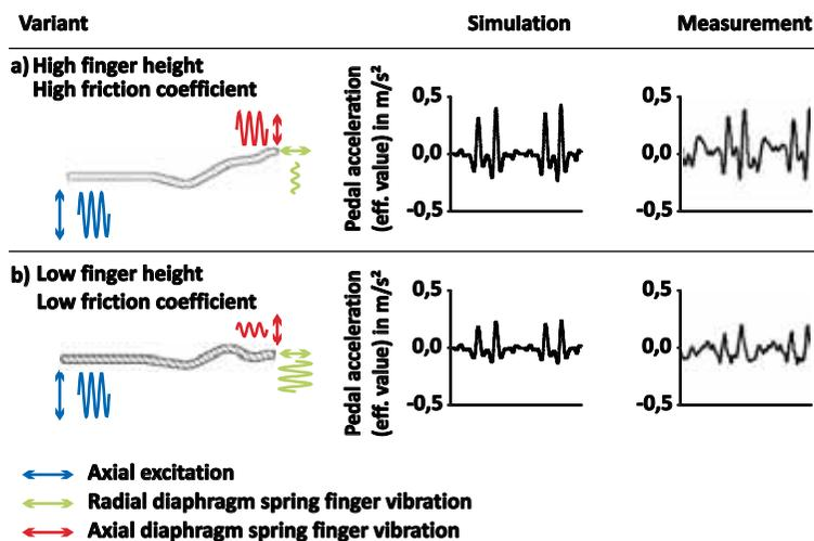
Figure 25 Pedal vibrations – detail optimization at the contact point between diaphragm spring finger and release bearing
