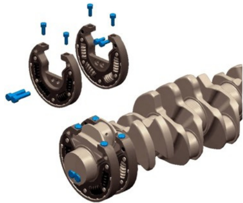
Fig. 14: Securing Two Dampers to the Crankshaft
