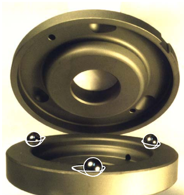
Figure 9: Circular ramp arrangement
