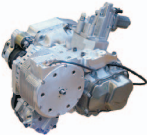
Figure 28 Prototype transmission with electric motor flange mounted on side
