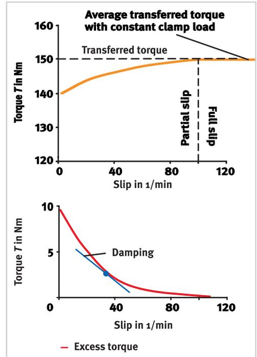
Figure 11 Slip-dependent excess torque and the resulting damping
