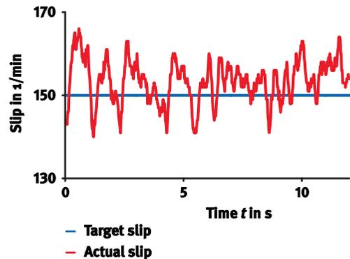
Figure 13 Measurement of the real limit cycle in the vehicle
