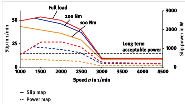
Figure 18 Slip map and mean introduced power
