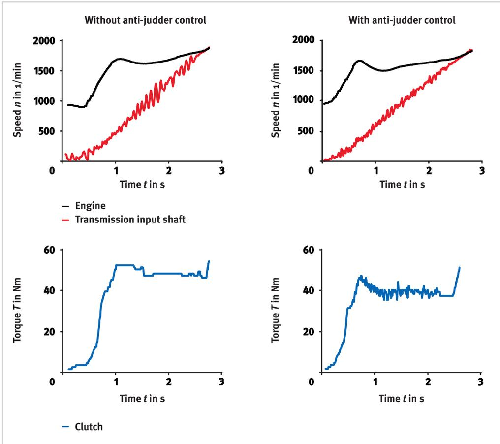
Figure 10 Feed-back anti-judder control under geometrical stimulation
