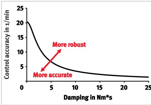
Figure 14 Achievable control accuracy for real systems
