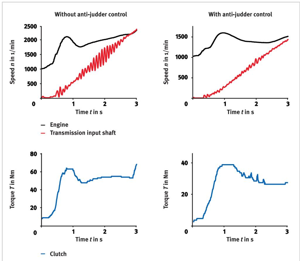
Figure 9 Feed-forward anti-judder control of self-induced judder
