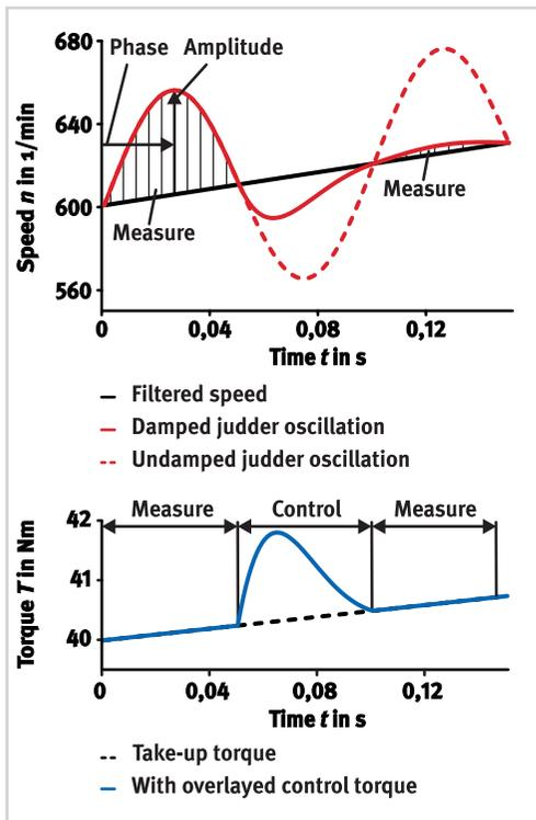
Figure 7 Feed-forward control system for judder reduction
