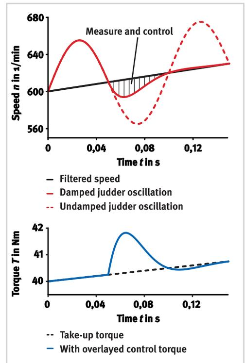
Figure 6 Feed-back control system for judder reduction
