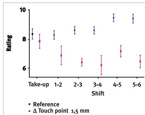
Figure 3 Rating with manipulated touch point and deactivated adaptation in comparison with original state
