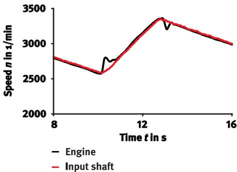
Figure 17 Vehicle measurement of slip control with load reversal
