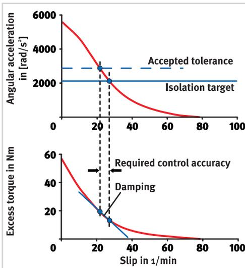
Figure 15 Isolation tolerance and damping for an operating point
