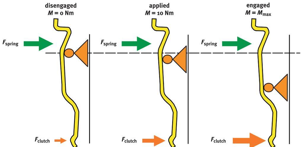
Figure 5 Lever actuator – engagement by displacement of support point
