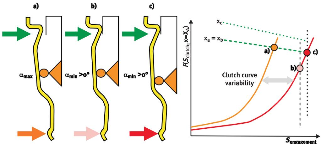
Figure 7 Lever actuator – robustness to tolerances
