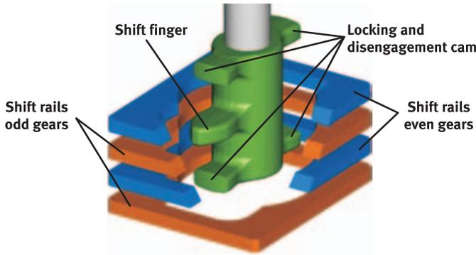
Figure 11 Integration of shift/select shaft with shift finger unit and shift rails
