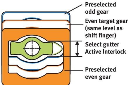
Figure 12 Active Interlock – select gate with engaged gears
