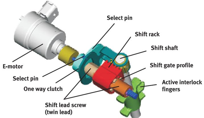
Figure 17 Kinematics of single motor transmission actuator
