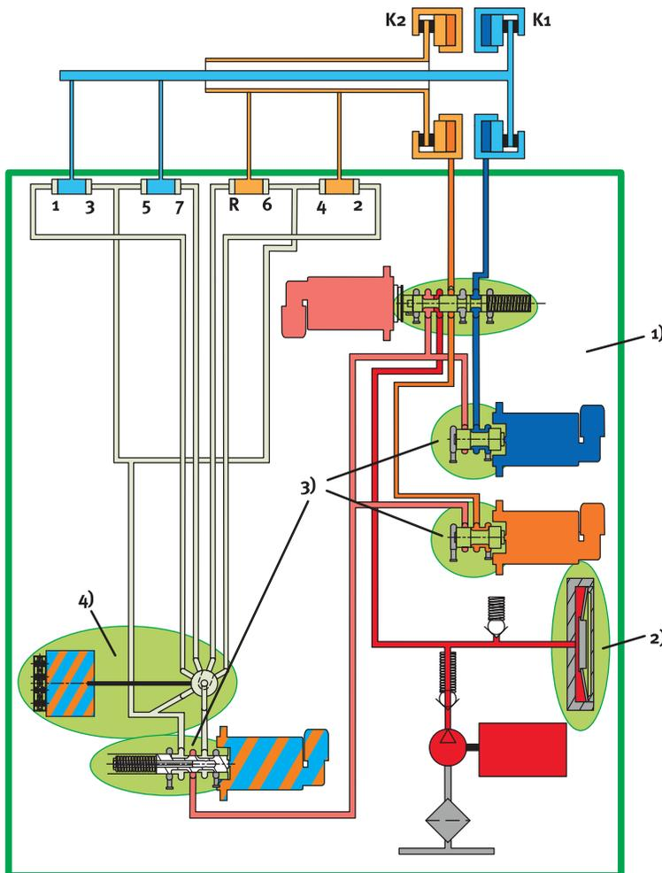
Figure 19 Hydraulic layout of power pack for double clutch transmission
