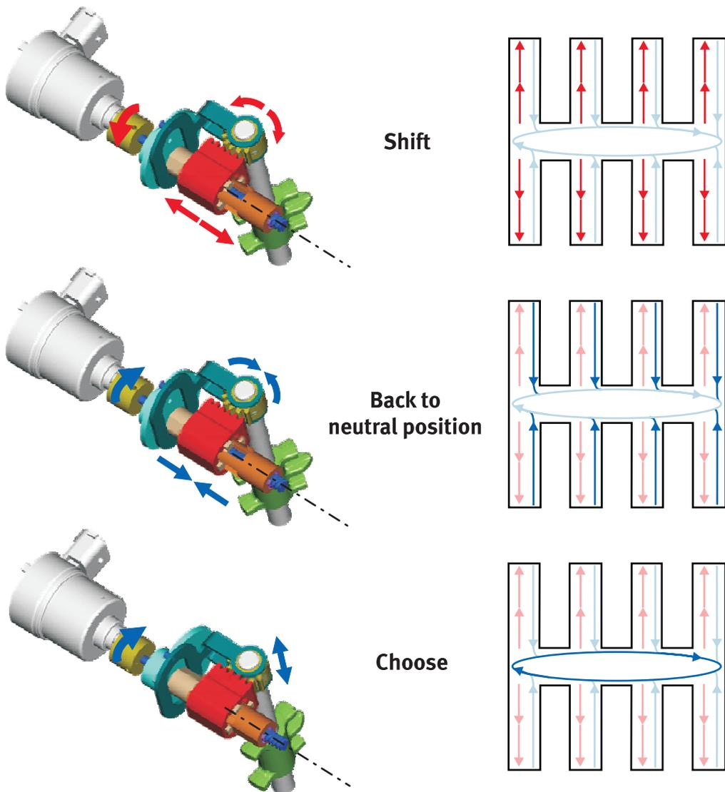
Figure 18 Single motor transmission actuator: function
