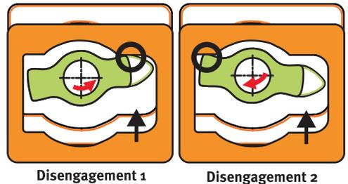
Figure 13 Active Interlock – disengagement of engaged gears
