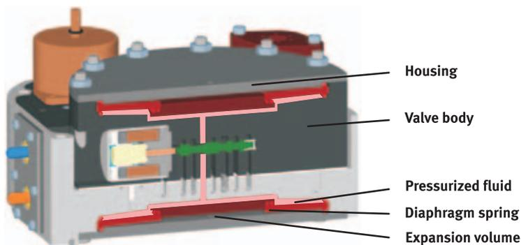
Figure 21 Power Pack with diaphragm spring accumulator
