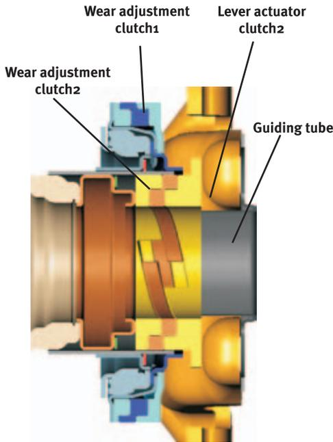
Figure 25 Double clutch engagement system with wear adjusters
