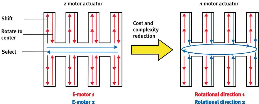
Figure 16 Single motor transmission actuator: basic concept
