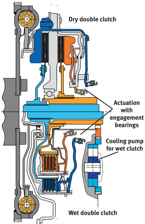
Figure 1 Modular clutch concept for actuation by means of clutch engagement bearing
