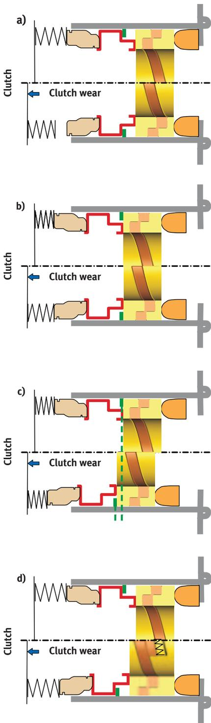
Figure 24 Wear adjustment in the clutch engagement system – function
