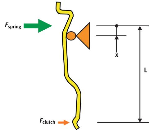
Figure 4 Lever principle
