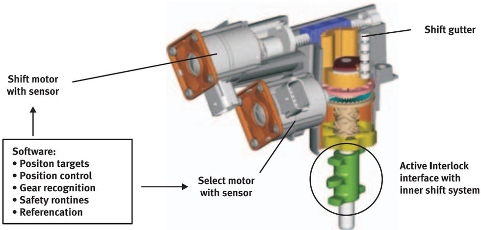
Figure 14 Transmission actuator with shift and select motors
