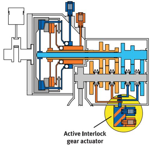
Figure 10 Active Interlock – one actuator for both sub-transmissions
