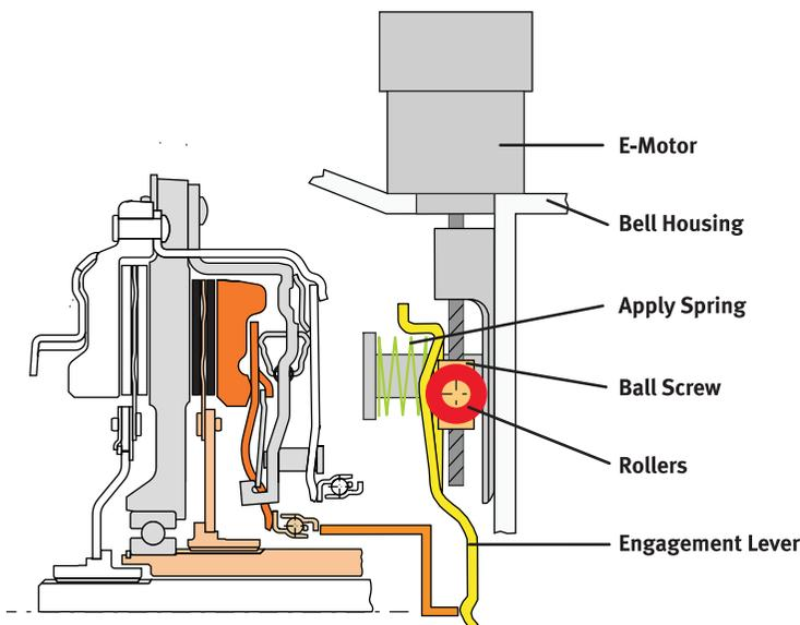
Figure 3 Lever actuator for clutch actuation – principle
