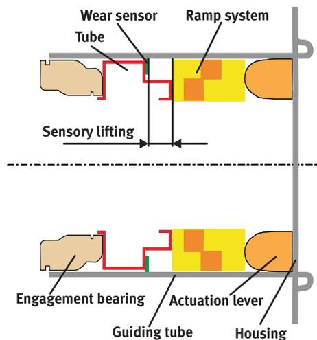
Figure 23 Wear adjustment in the clutch engagement system – schematic
