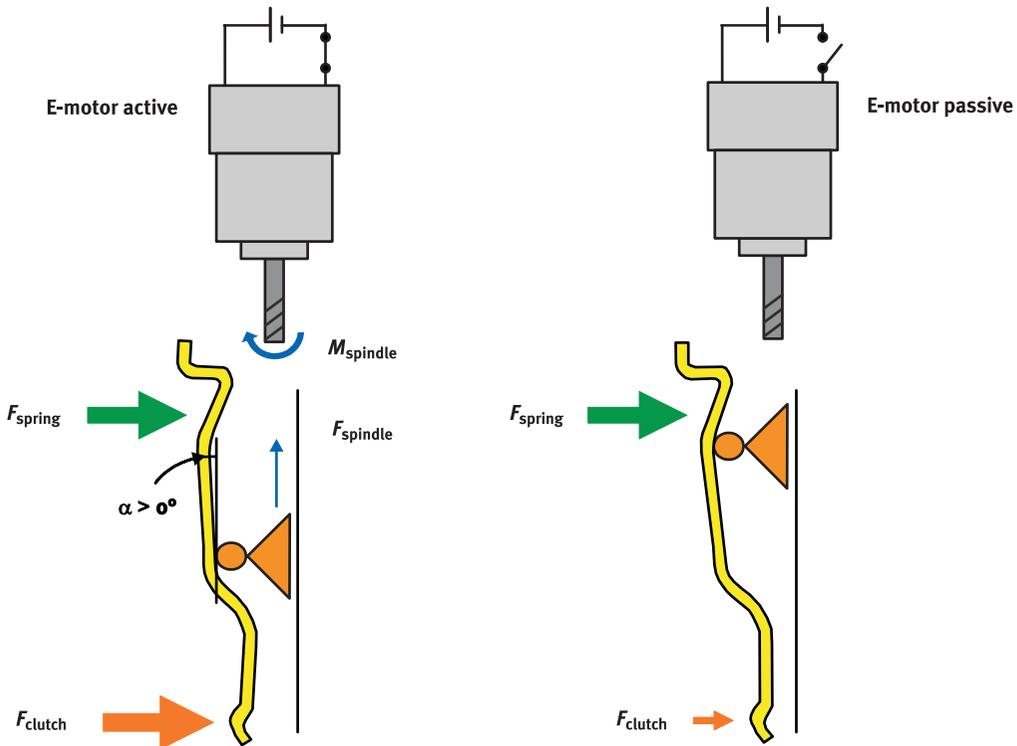
Figure 6 Passive opening under loss of power
