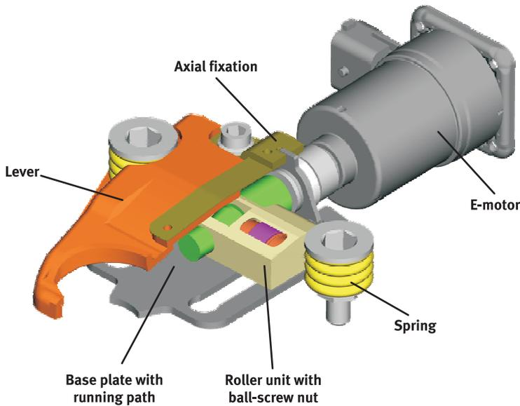
Figure 8 Model of lever actuator
