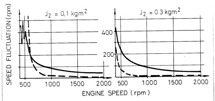
J2 = TRANSMISSION INERTIA + ADDITIONAL INERTIA
