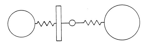
ADDITIONAL INERTIA ON TRANSMISSION INPUT SHAFT
