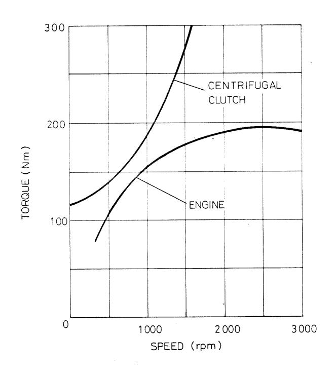
TORQUE CURVE OF ENGINE AND CENTRIFUGAL CLUTCH
