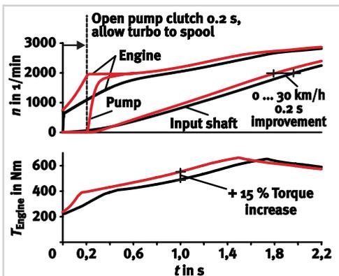
Figure 33 Simulation of improved acceleration from slipping impeller clutch
