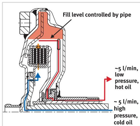
Figure 35 Cooling Circuit 1
