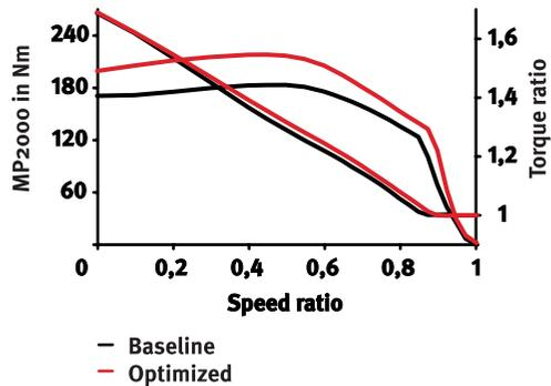
Figure 16 TC characteristic with diffuser stator
