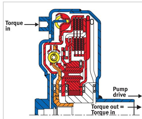
Figure 40 Fully Locked Mode
