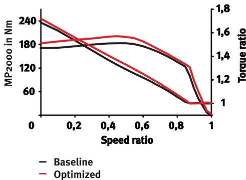
Figure 14 TC characteristic with increased radius
