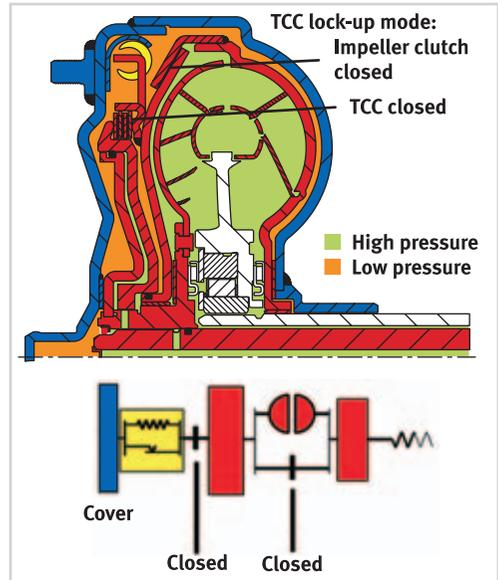
Figure 29 Pressurizing the closed piston engages the torque converter clutch
