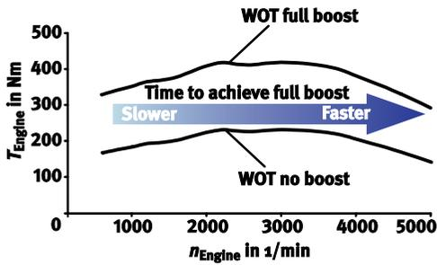
Figure 32 Engine output torque variation due to turbocharger lag
