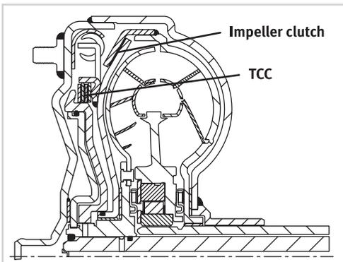
Figure 26 Three-Pass Multi-Function Torque Converter with 273 mm torus
