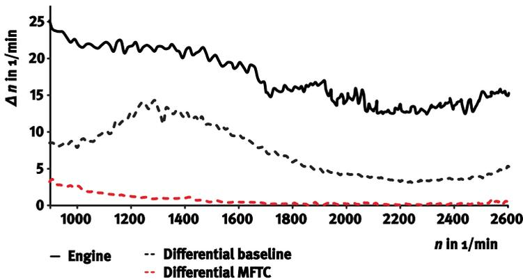
Figure 31 Measurement of torsional vibration isolation improvement with MFTC
