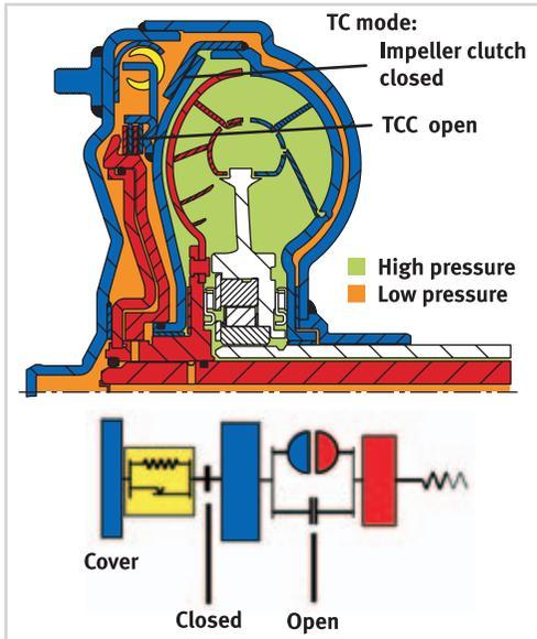
Figure 28 Engaged impeller clutch provides conventional torque converter operation
