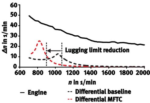
Figure 30 Simulation of torsional vibration isolation improvement with MFTC
