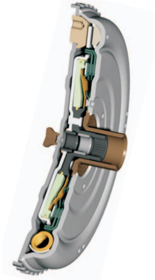
Figure 24 Hybrid damper with lockout feature to eliminate start-stop resonance
