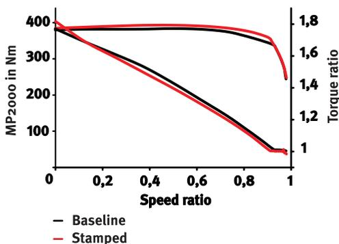
Figure 3 Measured TC characteristic
