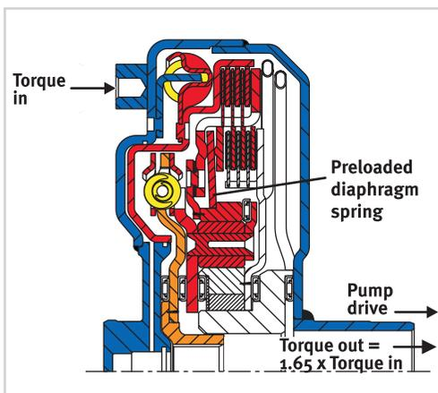
Figure 39 Torque Multiplication Mode
