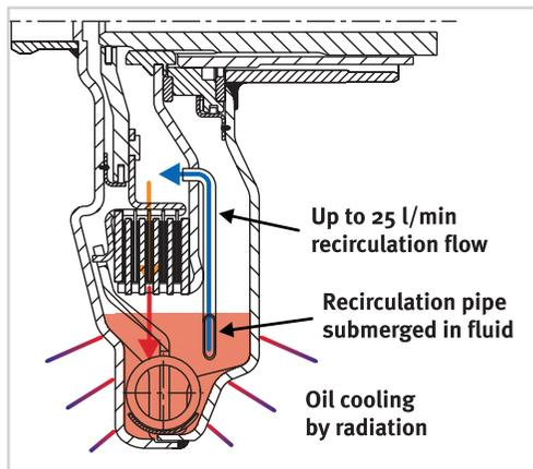
Figure 36 Cooling Circuit 2
