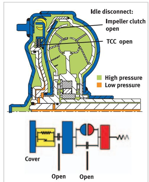
Figure 27 Disengaged impeller and torque converter clutches at idle to save fuel
