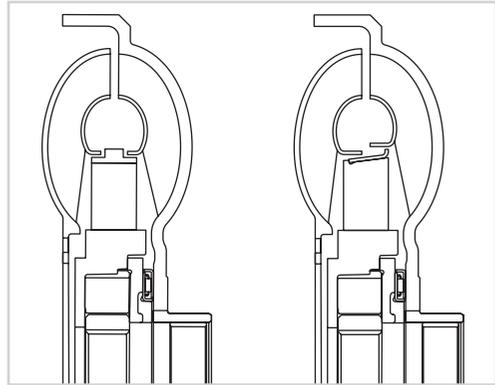
Figure 15 Diffuser style stator
