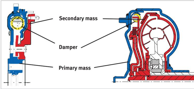
Figure 25 Inertia distribution of a Dual-Mass Flywheel (left) and Multi-Function Torque Converter (right) when the TCC is locked
