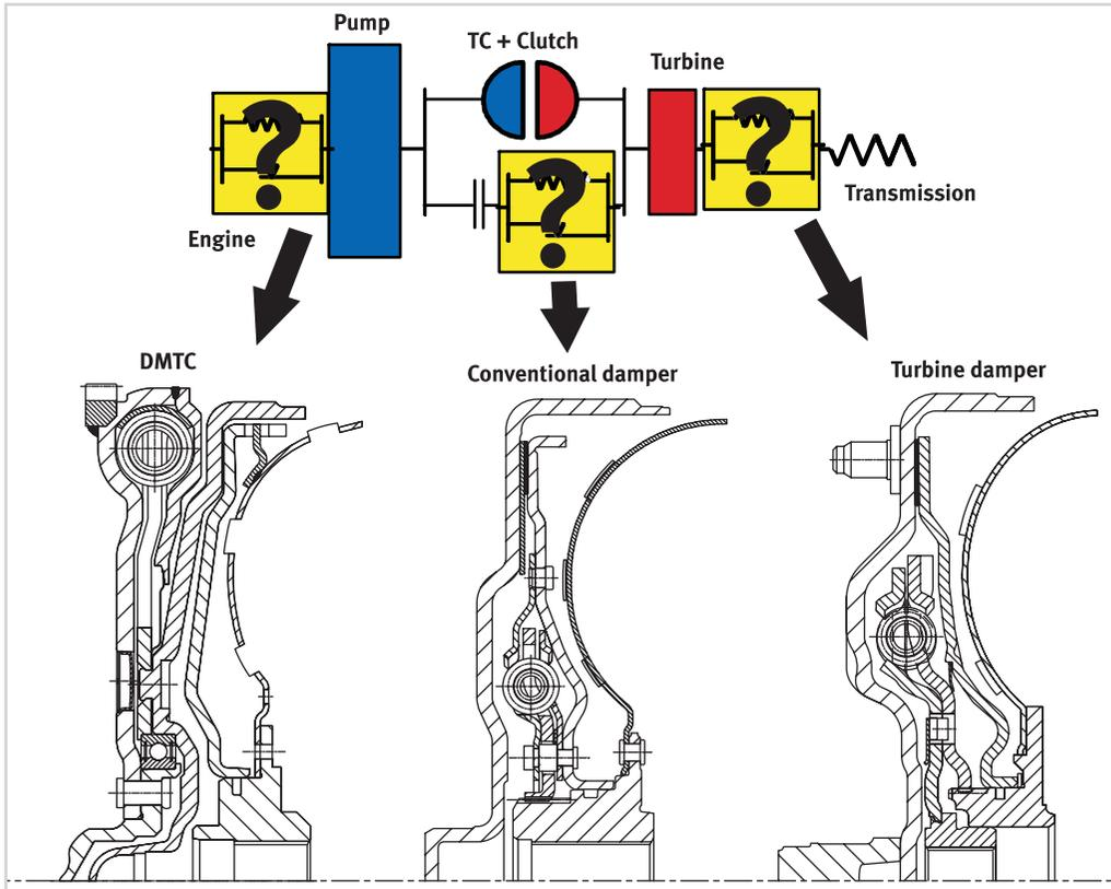
Figure 20 Representative dampers for each position.
