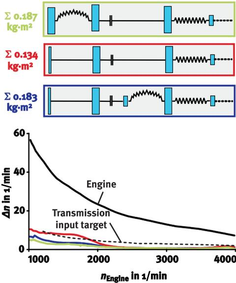
Figure 23 Drivetrain response versus target for advanced damper concepts
