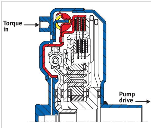
Figure 38 Idle Disconnect Mode
