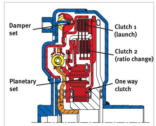
Figure 37 The Mechanical Torque Converter
