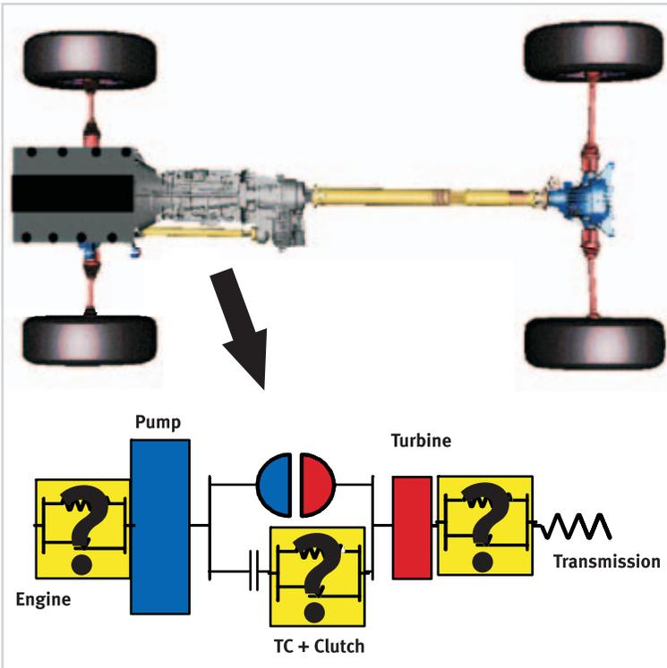
Figure 19 Possible Damper positions for a traditional planetary automatic transmission
