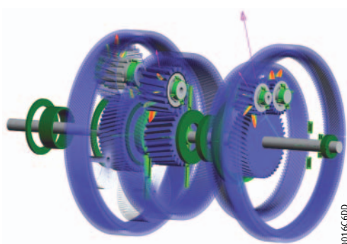
Figure 1: Planetary gear sets in an automatic gearbox
