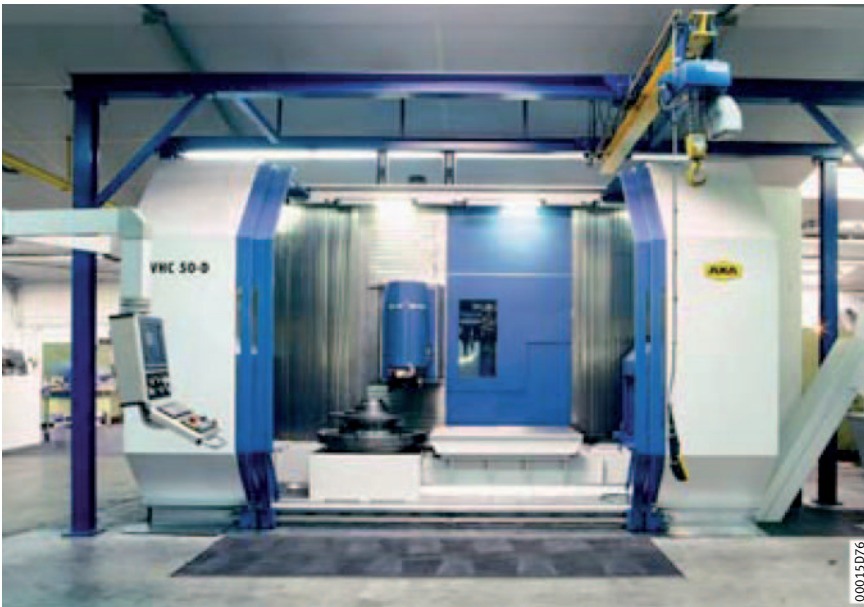
Figure 8 - Turning/milling centre, type VHC50-D from AXA Maschinenbau GmbH
