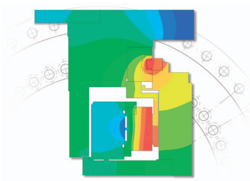
Figure 3: Temperature calculation (simulation) for a direct drive rotary table axis
