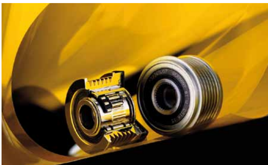
The overrunning alternator pulley supports belt-driven starter generators, which with 48 volts are powerful enough to provide kinetic energy recovery and drive the wheels for short periods in addition to the starting and alternator functions.
