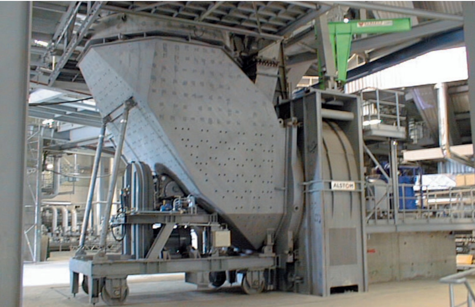
Beater wheel mill N 535.43V built by ALSTOM Power Stuttgart, Germany
