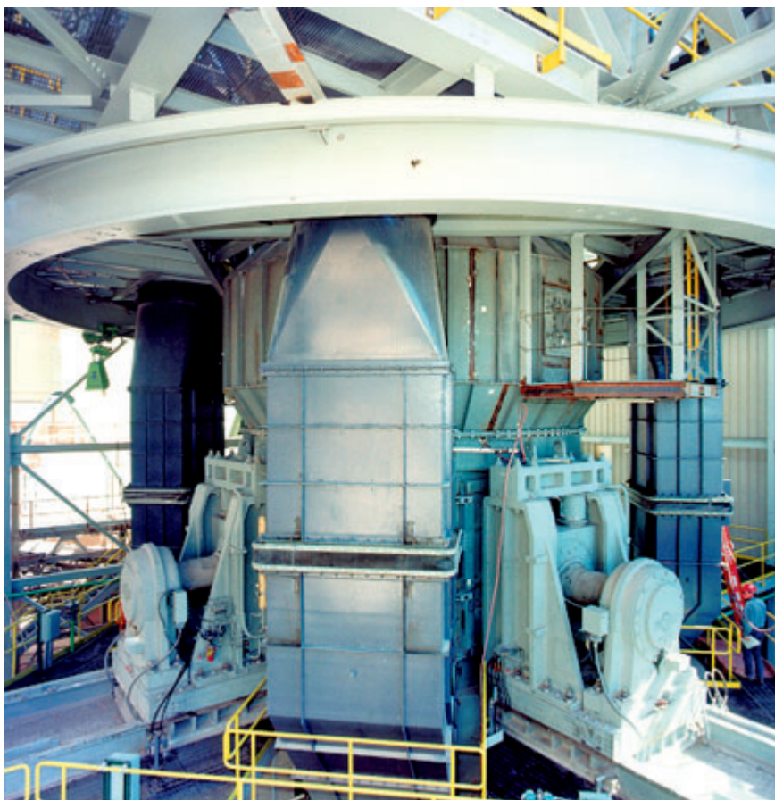
QUADROPOL roller mill with special spherical roller bearings
