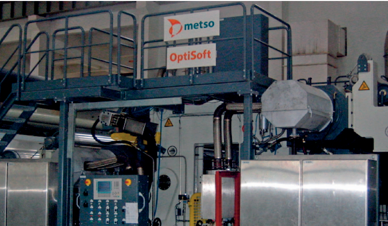
Soft nip calender Manufacturer: Metso Paper, Finland; Operator: Shandong Sun Paper Co. Ltd., Yanzhou City/China
