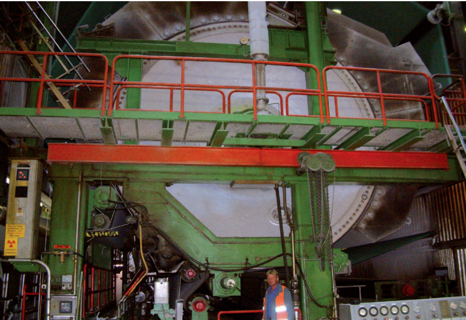
Lenzing paper mill, Austria M.G. cylinder in the dryer section of a paper machine
