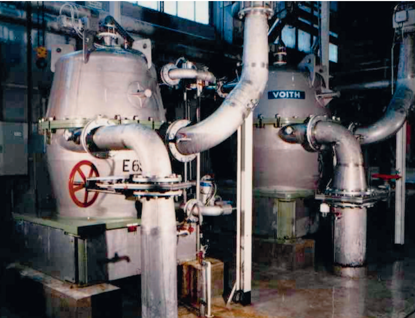
"Spectro Screen 23D" pressure screen, Voith Paper, Germany
