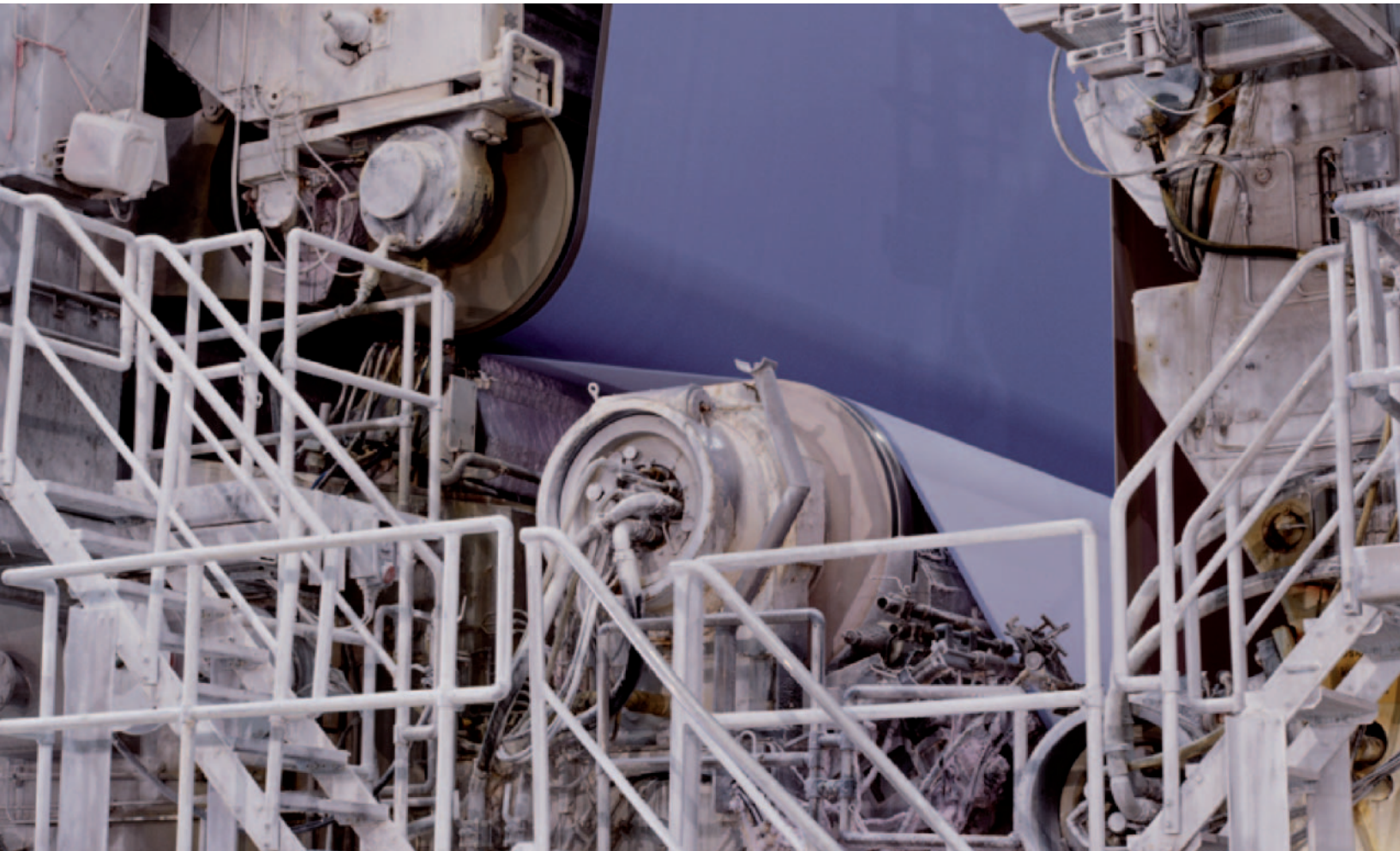
Spreader rolls in paper machine. Operator: UPM-Kymmene, Jämsänkoski/Finland
