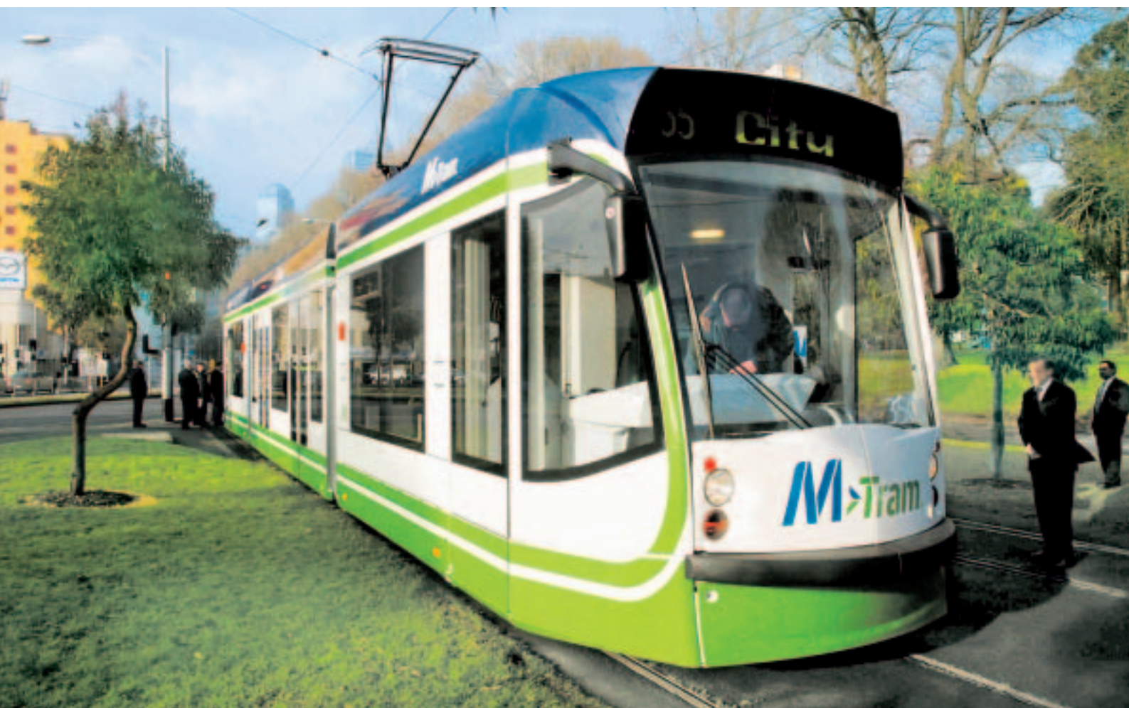
Combino® five-section, articulated low-floor tramcar built by Siemens AG, Transportation Systems – Light Rail, Germany
