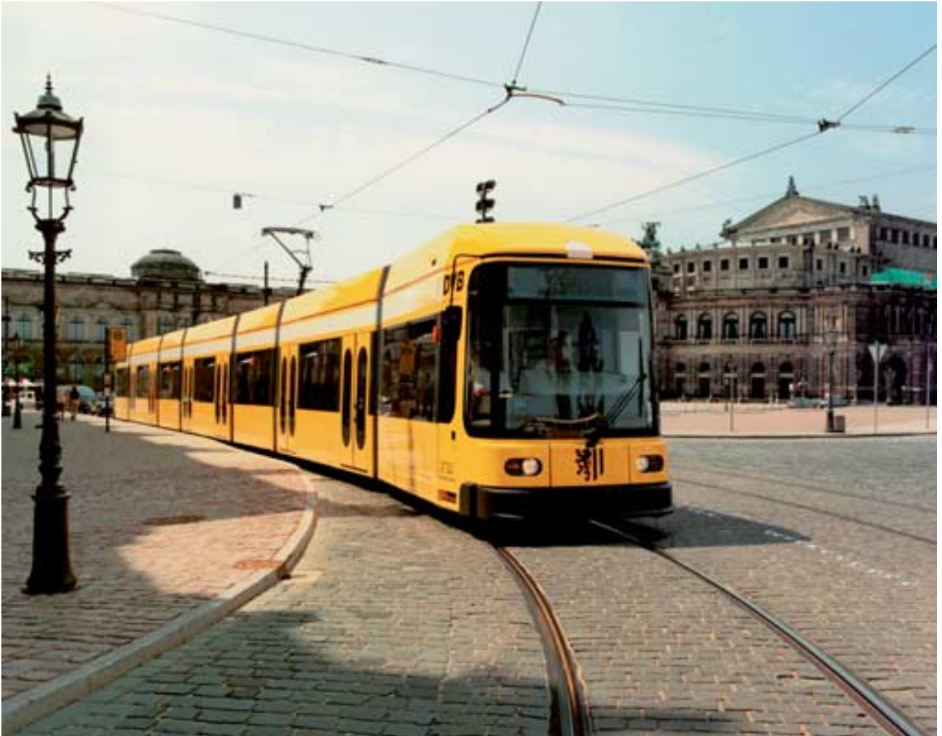
Dresden NGT8DD tramway car developed and built by Siemens AG Transportation Systems
