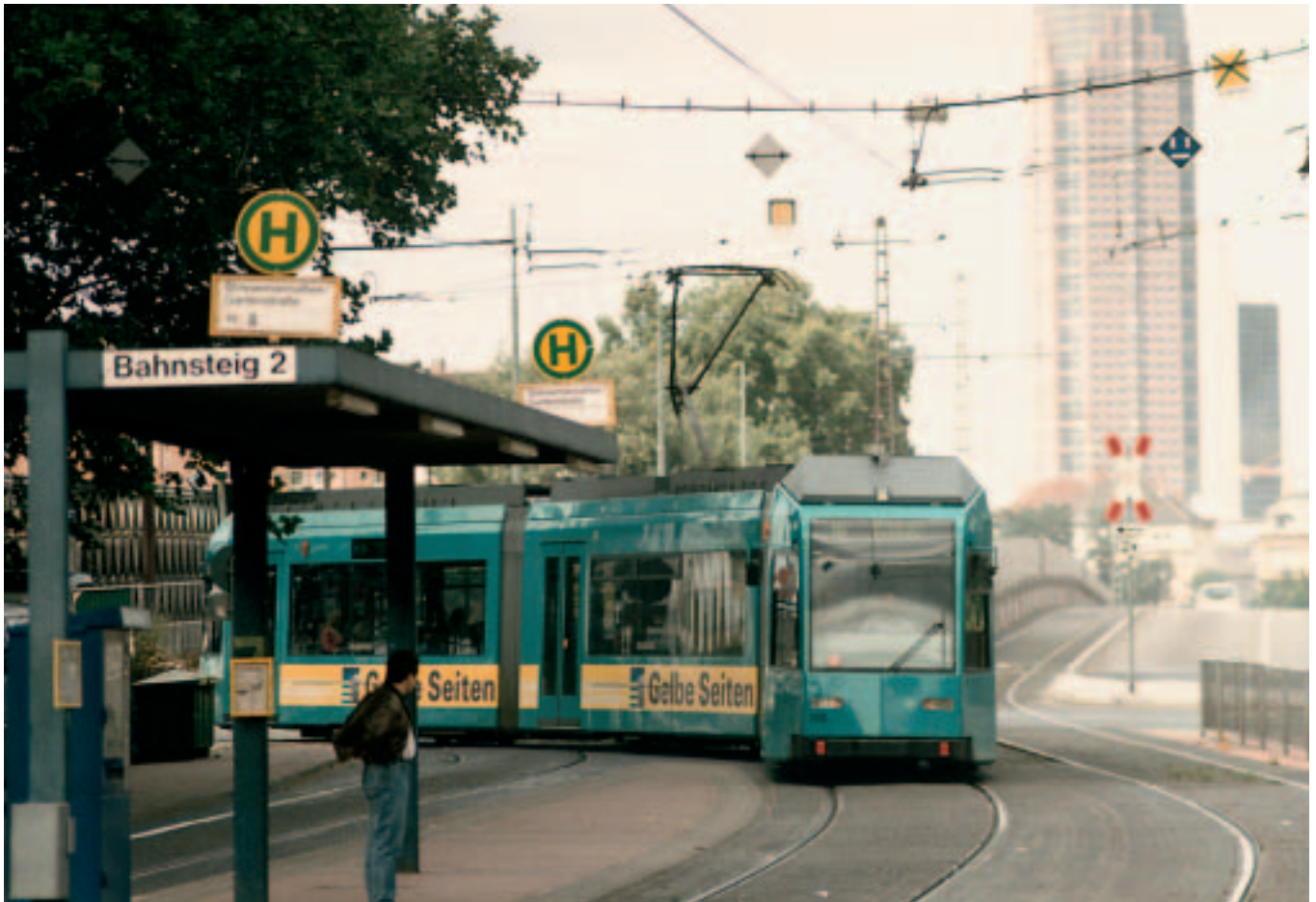
Low-floor tram with wheel hub drives.
