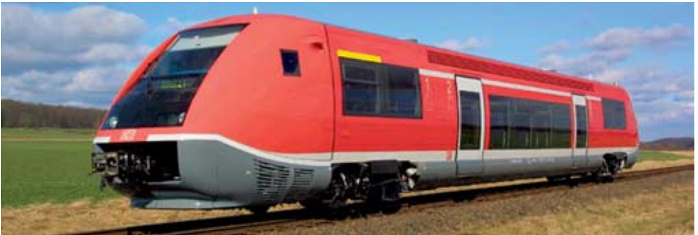
VT641: Diesel rail car for the German Railways DB Diesel rail cars developed and built by ALSTOM GmbH
