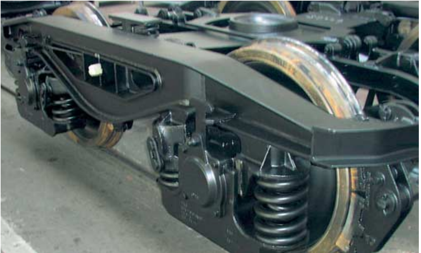
FAG wheelset bearing - ASB130Z.176181 - for Y25-type bogies in freight cars up to 25 t axle load.
