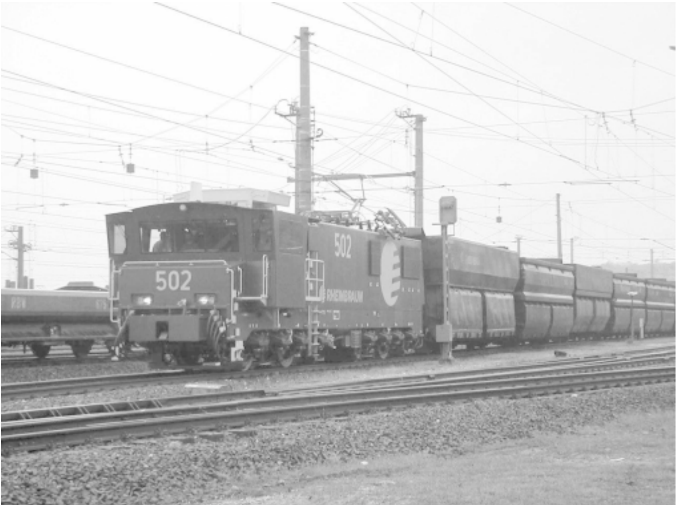
Heavy-freight locomotive of series EL2000: developed by ADtranz in cooperation with Rheinbraun AG
