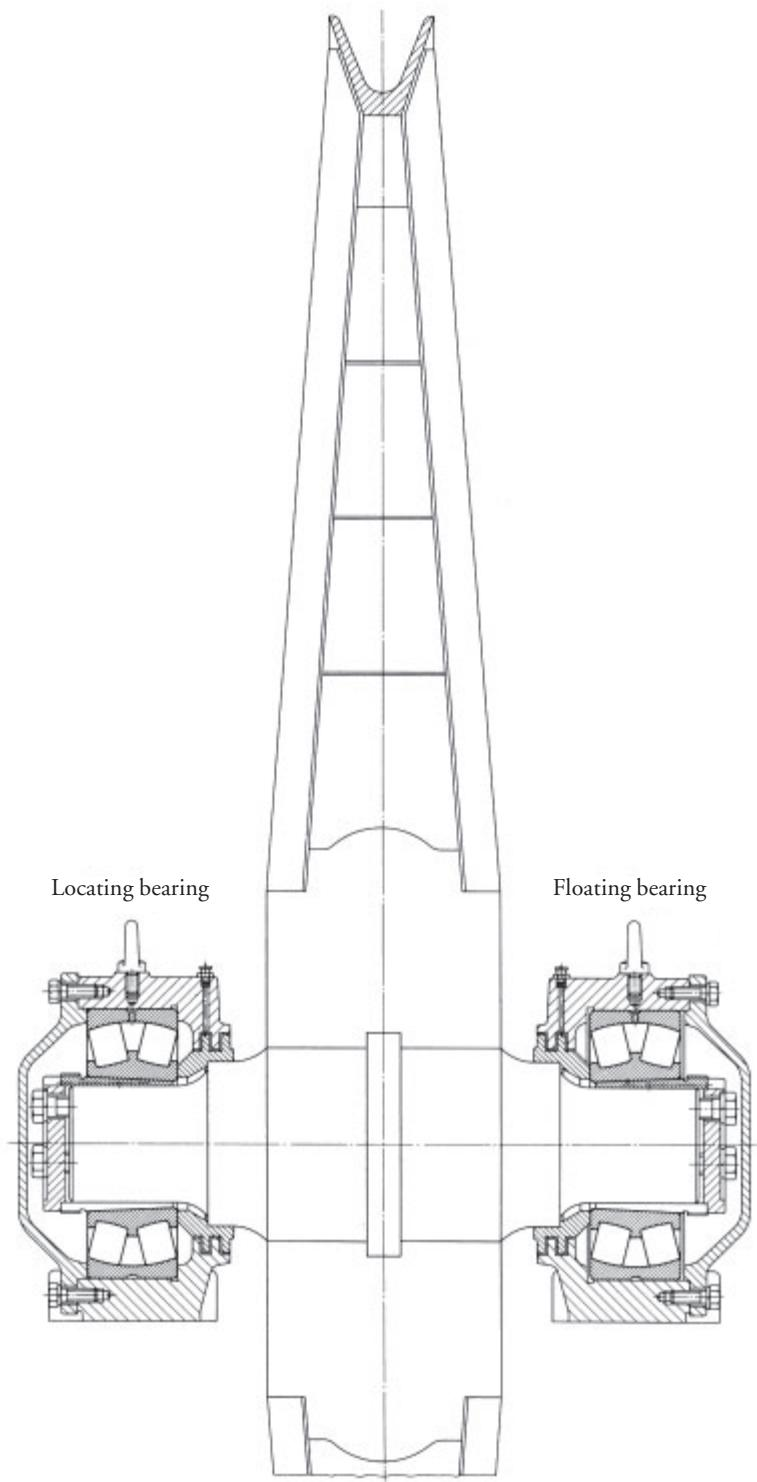
75: Rope sheave (underground mining)
