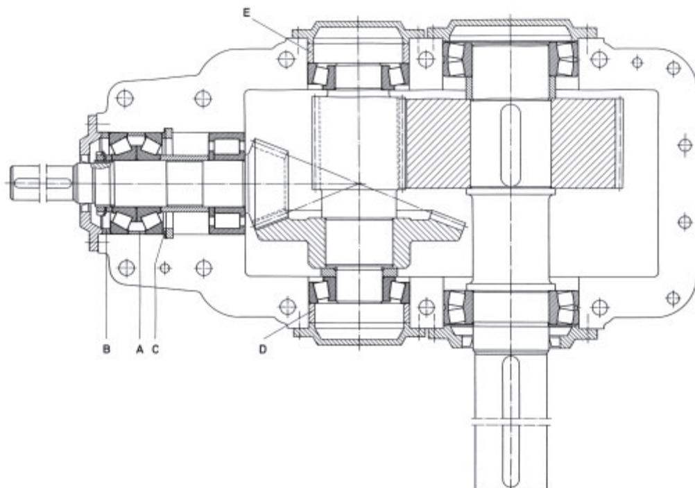
29: Bevel gear-spur gear transmission
