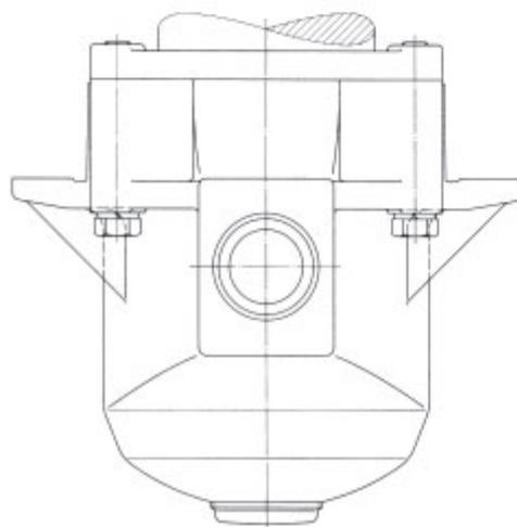
44: UIC axle boxes with spherical roller bearings
