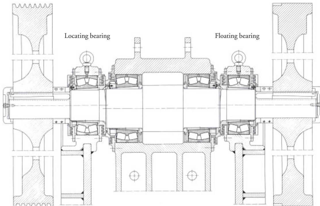
92: Bearing mounting of a double-toggle jaw crusher
