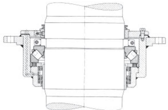
59: Rudder carrier bearing FAG RS9284W.1.....
