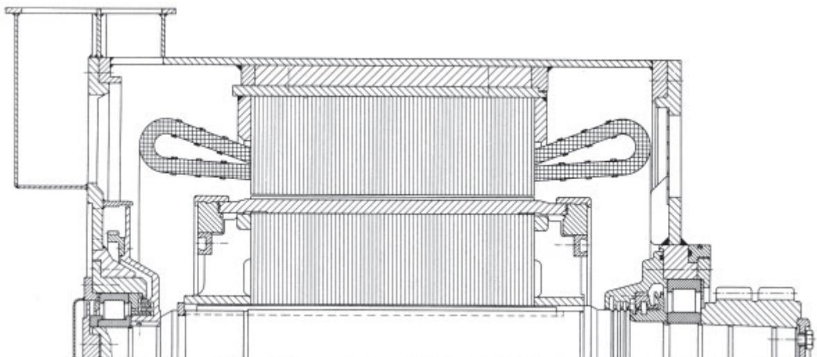
1: Traction motor for electric standard-gauge locomotive
