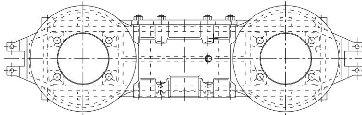
47: Axle box roller bearings of the Channel tunnel's freight engine, class 92
