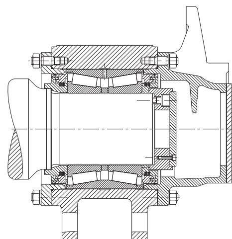
46: Axle box roller bearings of the ICE driving unit
