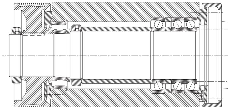
11: CNC-lathe main spindle
