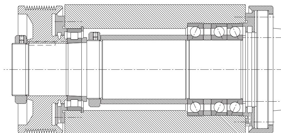
11: CNC-lathe main spindle
