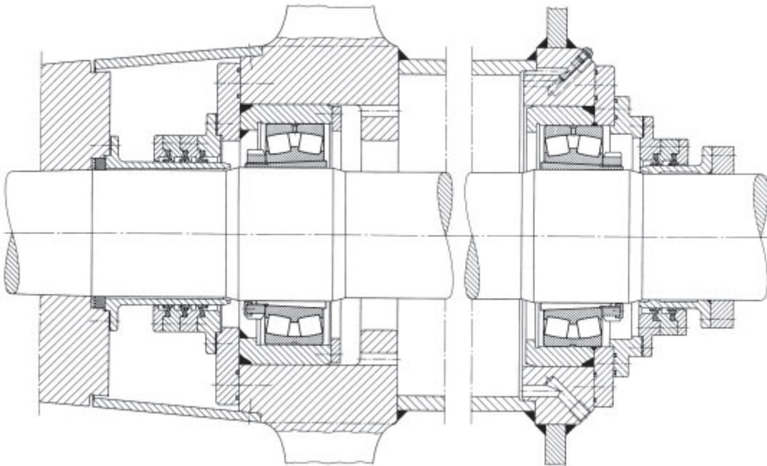
62: Stern tube or tail shaft bearing arrangement
