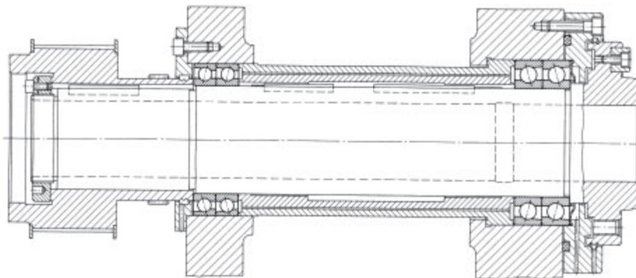
10: NC-lathe main spindle
