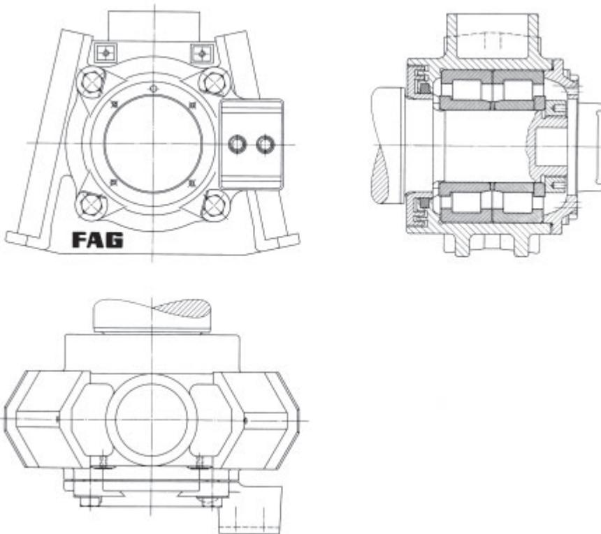
48: Axle box roller bearings for an underground train
