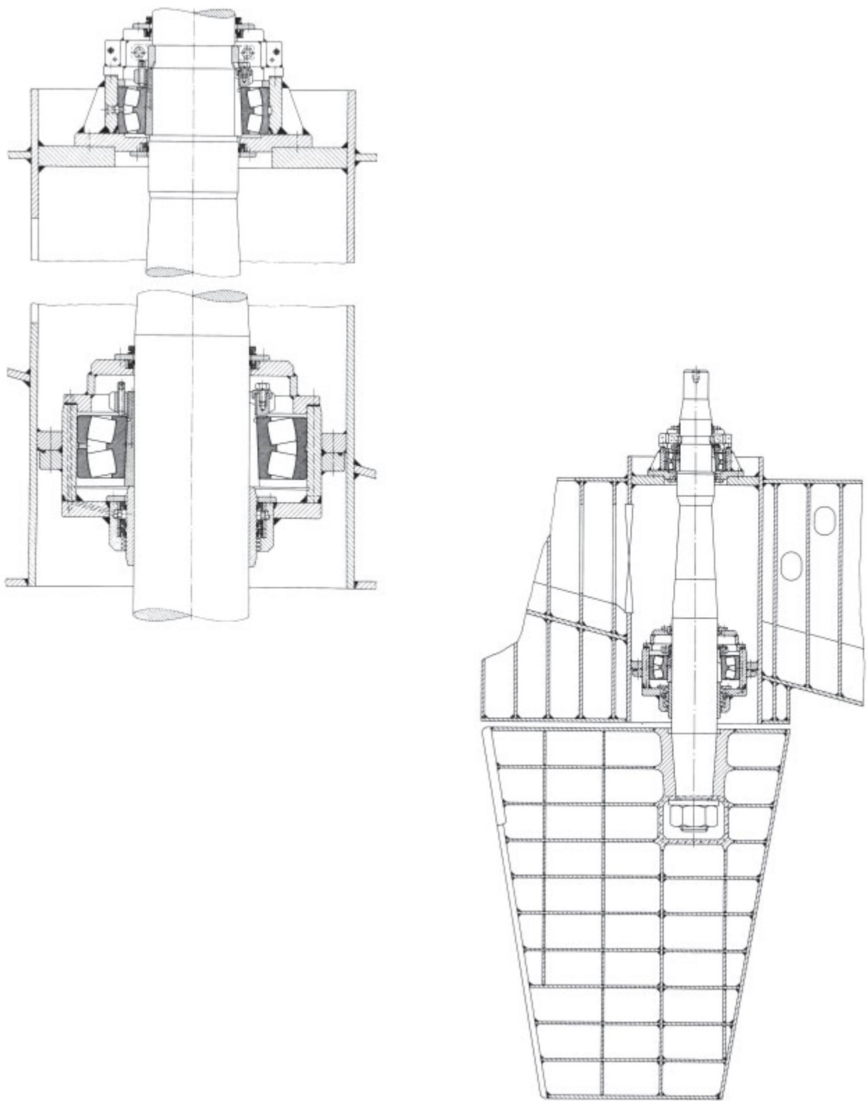
60: Spade-type rudder bearings
