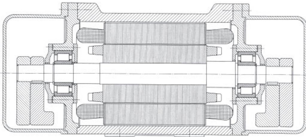
100: Imbalance rotor bearings of a vibrator motor
