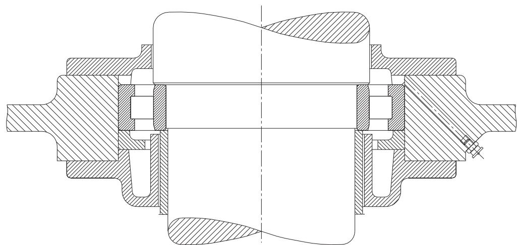
6: Rotor bearing arrangement of a vertical-pump motor
