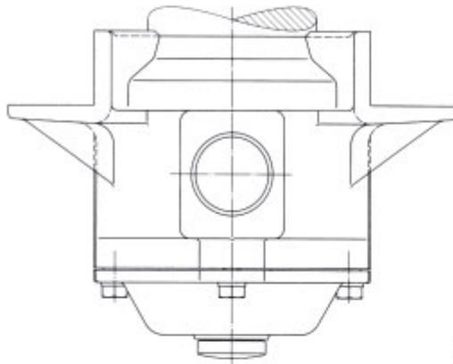
43: UIC axle boxes with cylindrical roller bearings
