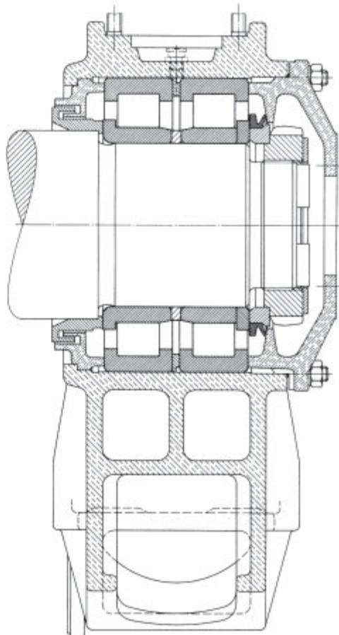
45: Axle box roller bearings of series 120's three-phase current locomotive
