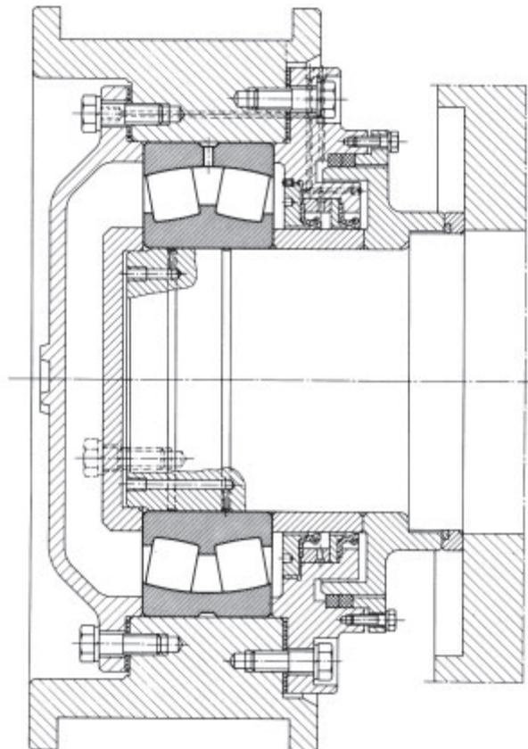
88: Bottom sprocket of a bucket chain dredger
