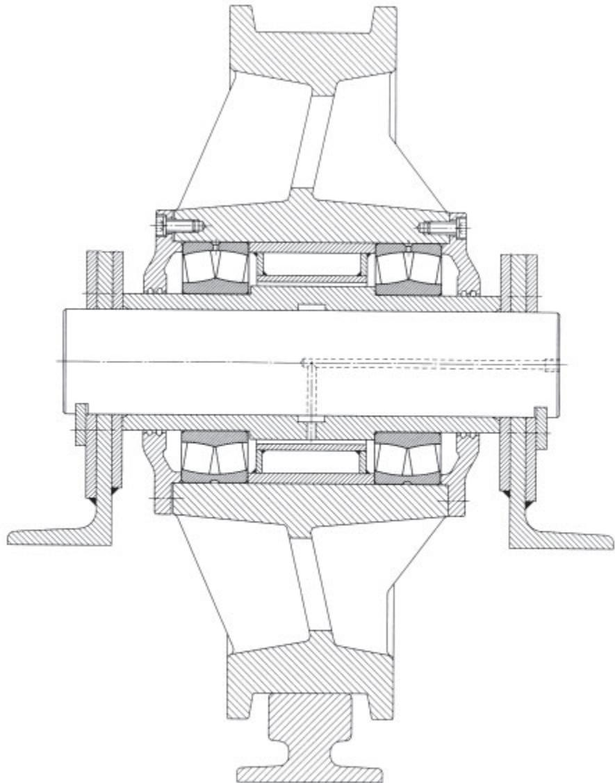
80: Crane run wheel with spherical roller bearings
