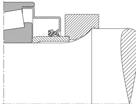
a: Rubbing radial shaft seal
