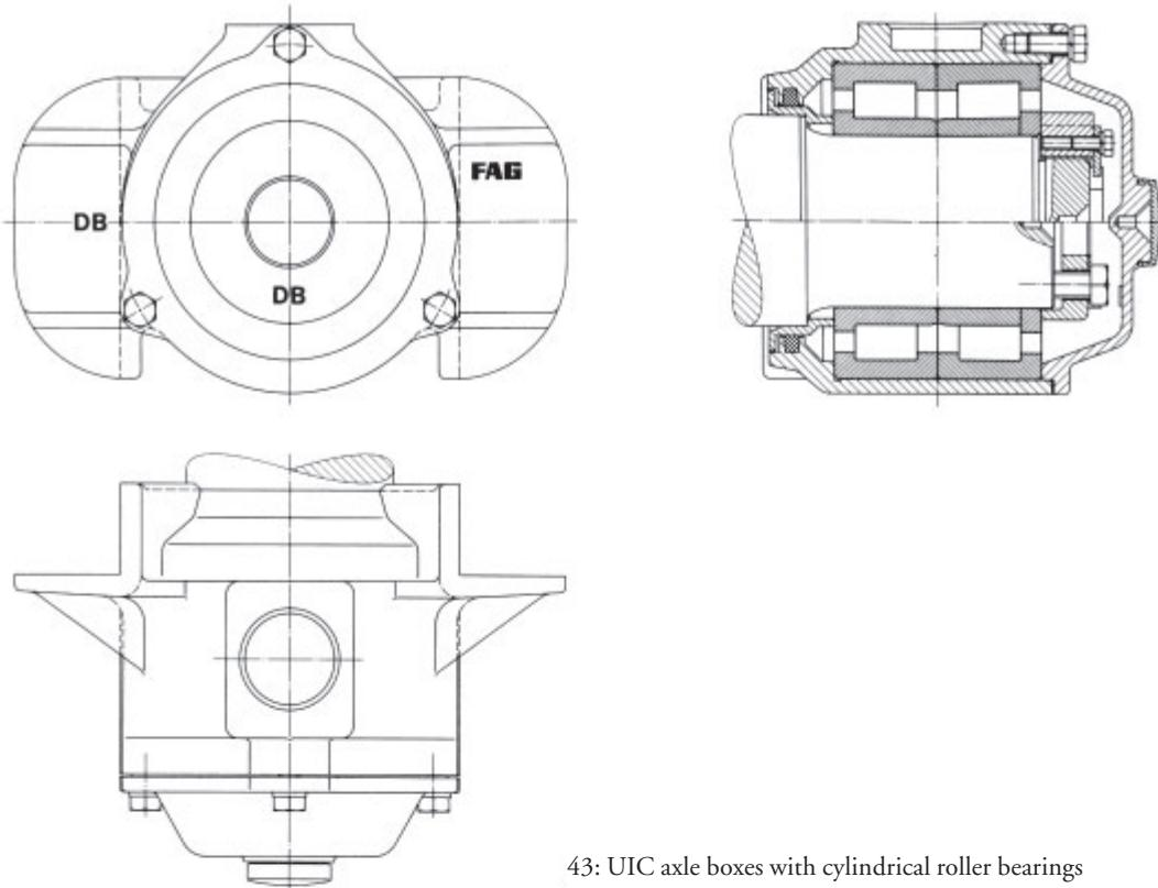
43: UIC axle boxes with cylindrical roller bearings
