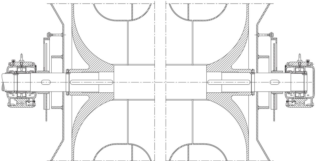
118: Rotor mounting of an exhauster
