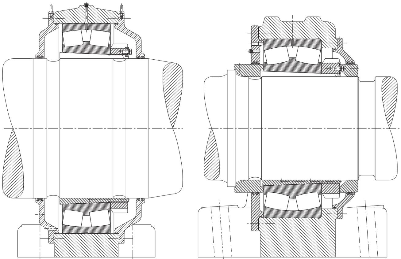
8: Rotor shaft bearings of a wind energy plant
