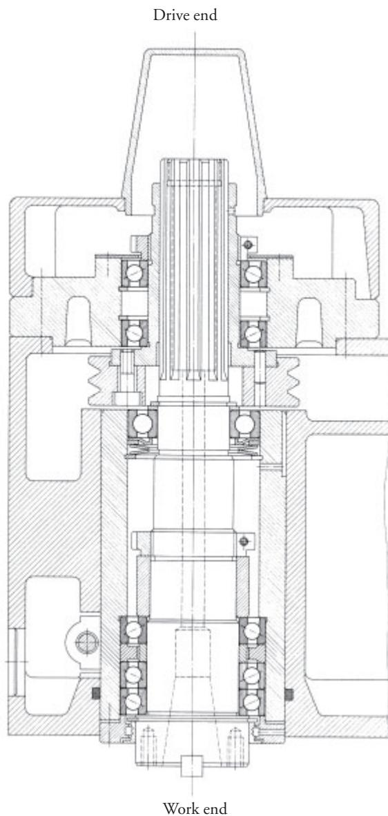
15: Bearing arrangement of a vertical high-speed milling spindle
