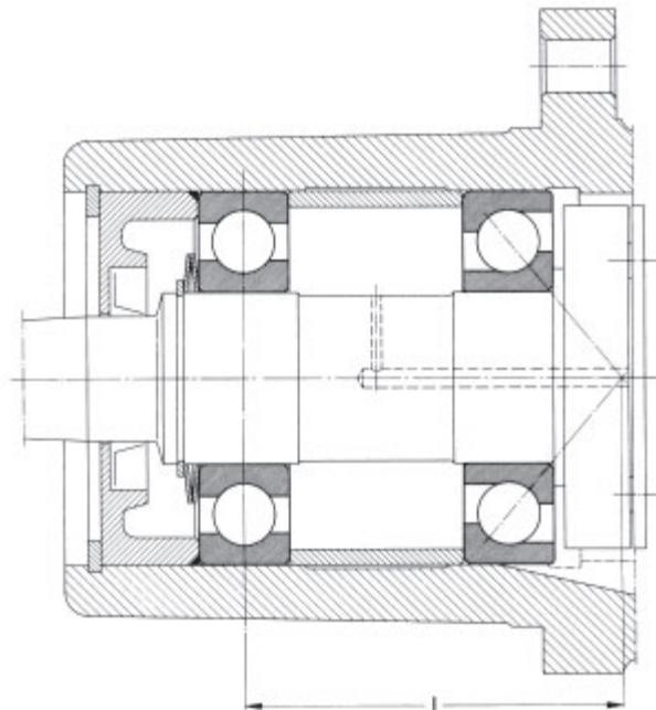
117: Drive flange of an axial piston machine
