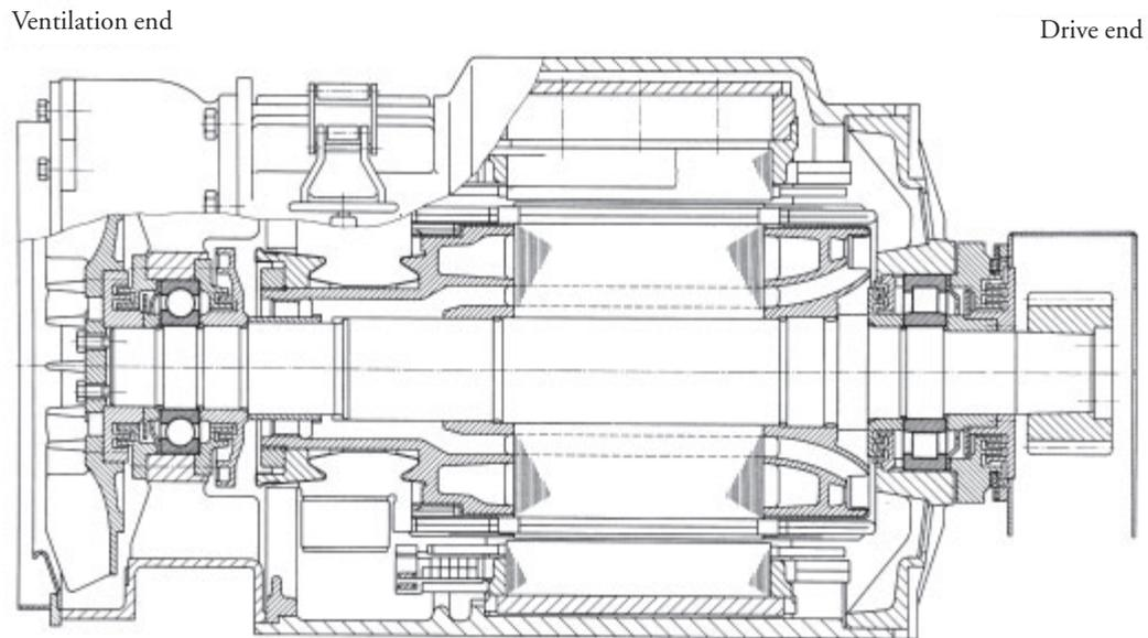
2: Traction motor of an electric commuter train
