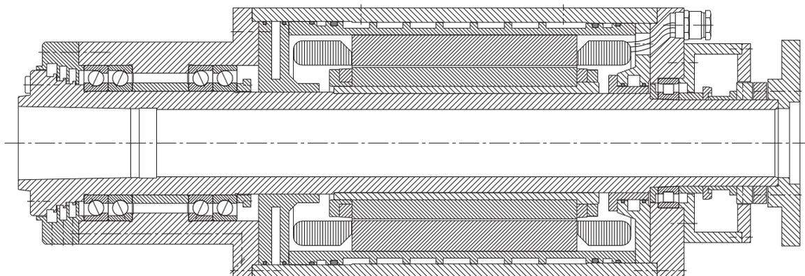
14: Motor spindle bearing arrangement of a lathe
