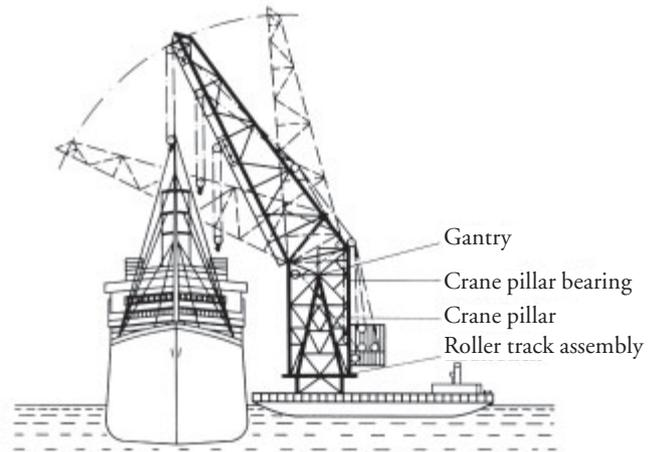
At the pillar foot the gantry is supported on a roller-track assembly (see example no. 79).
