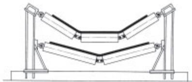
Fig. 86 shows idler garlands connected by chain links. These idlers are part of a conveying installation for rock phosphate. The bearings fitted are deep groove ball bearings FAG 6303.2ZR.C3.
