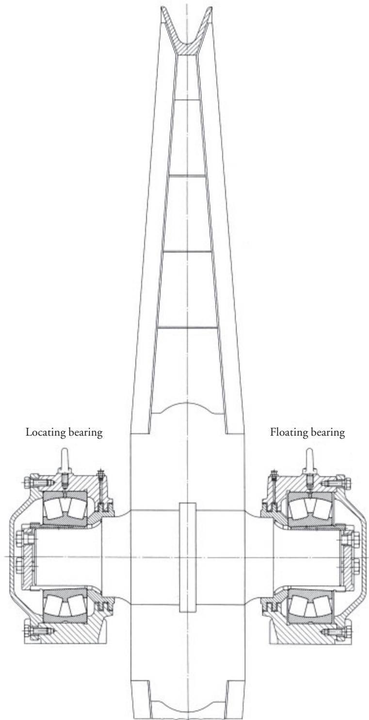
75: Rope sheave (underground mining)
