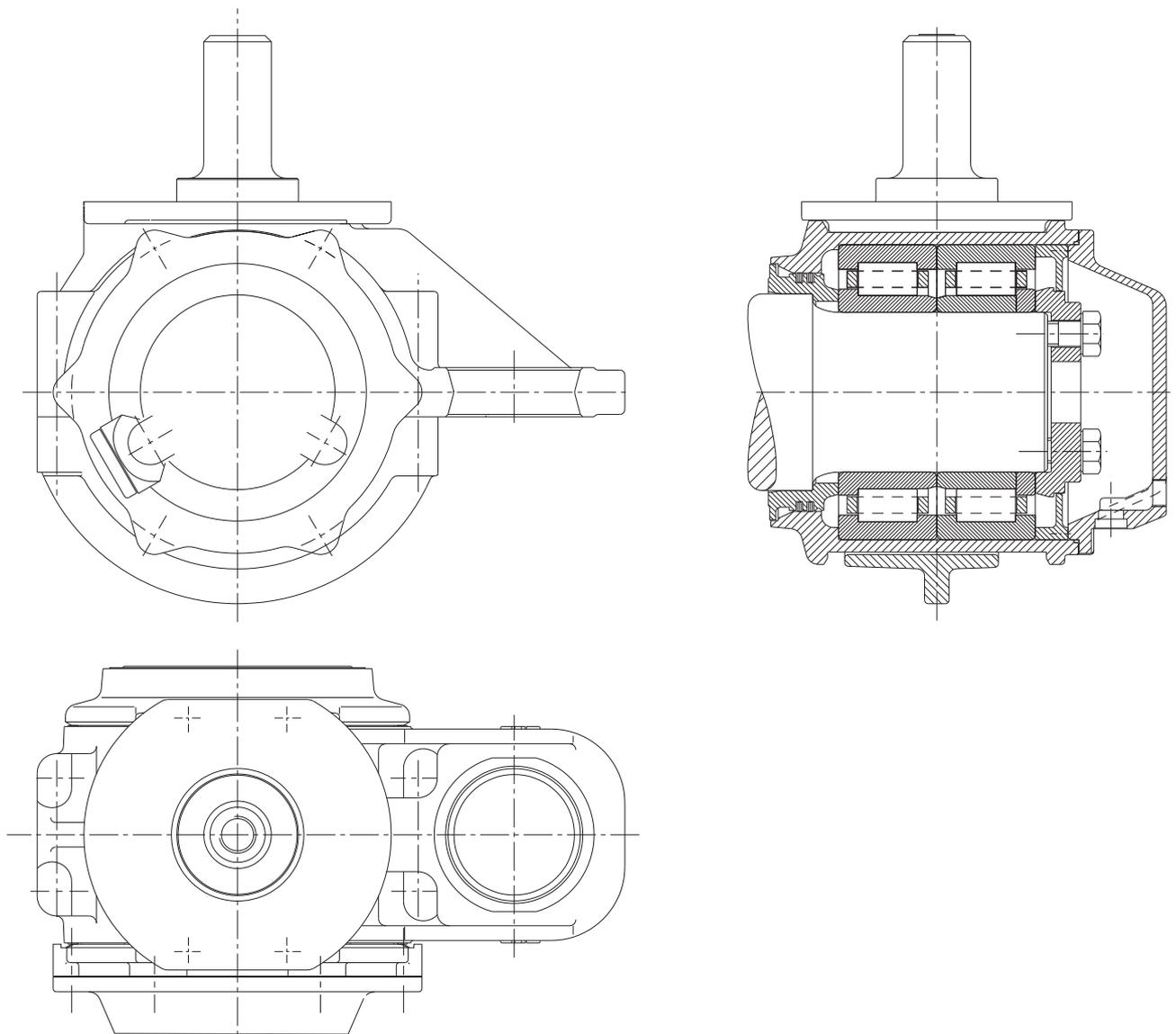
42: Axle box roller bearings of an Intercity train carriage
