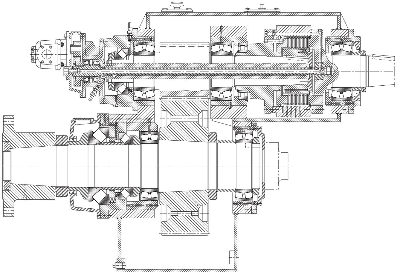
28: Bearing arrangement of a marine gear
