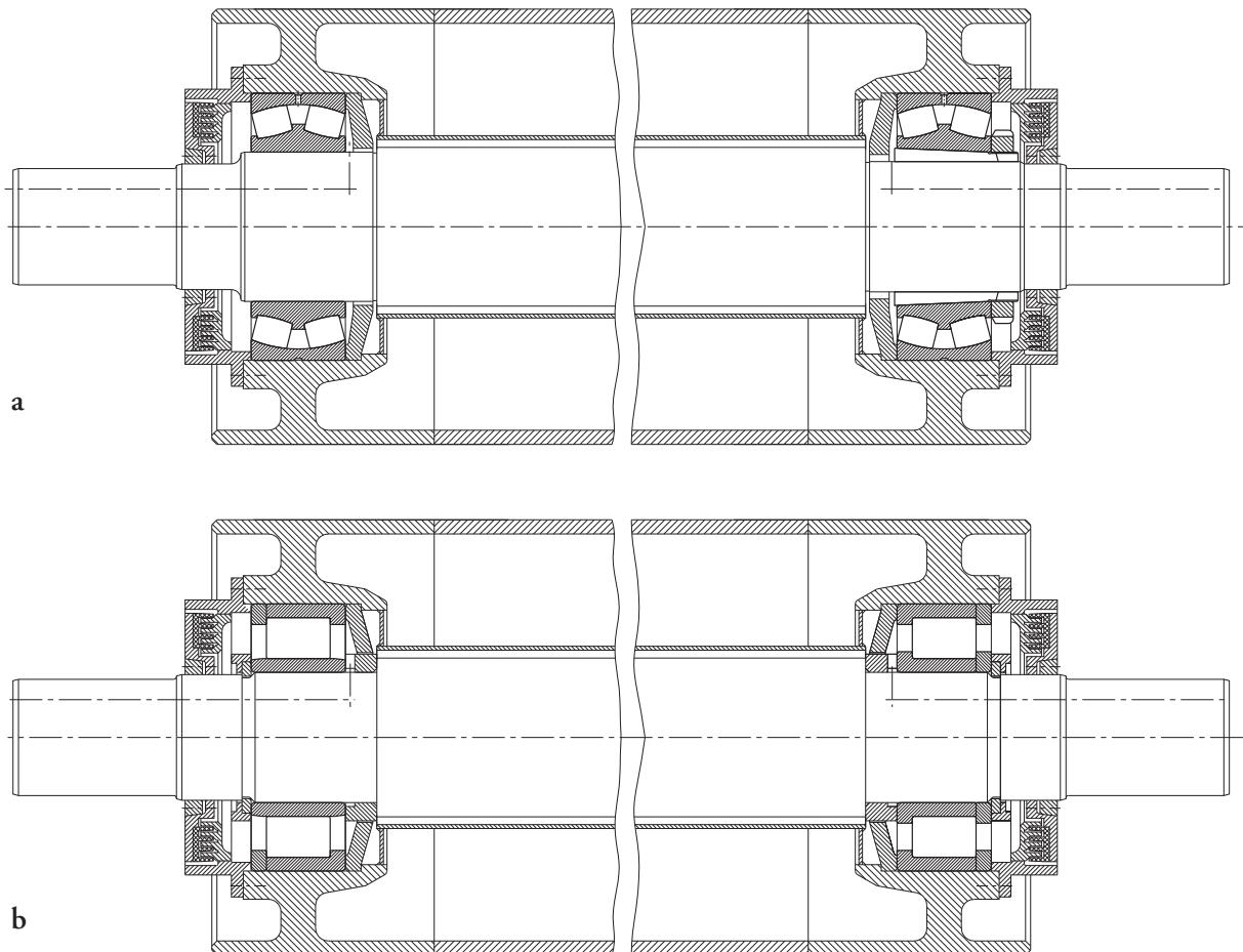
84: Internal bearings for the tension / take-up pulley of a belt conveyor
