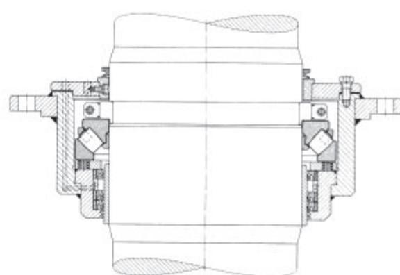
59: Rudder carrier bearing FAG RS9284W.1.....
