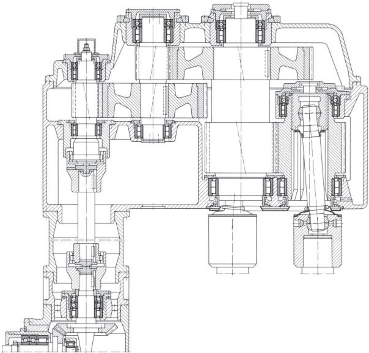
107: Combined reduction and cogging wheel gear of a billet mill
