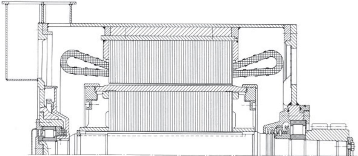
1: Traction motor for electric standard-gauge locomotive
