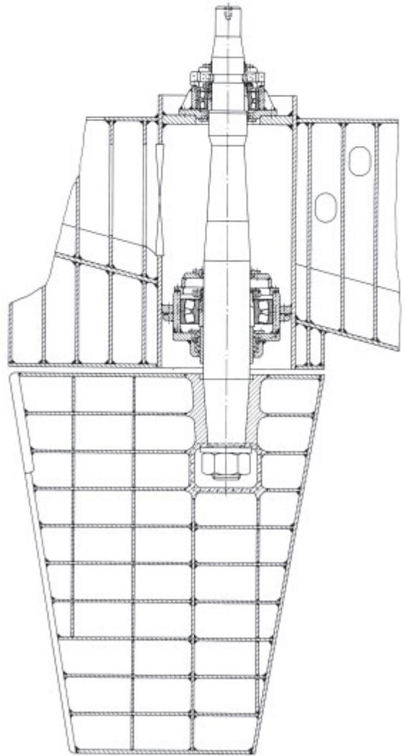
60: Spade-type rudder bearings
