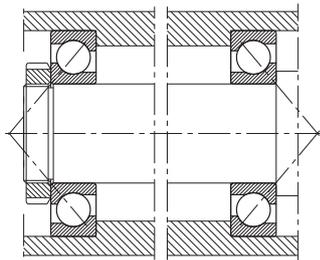
Adjusted bearing arrangement (X arrangement)
