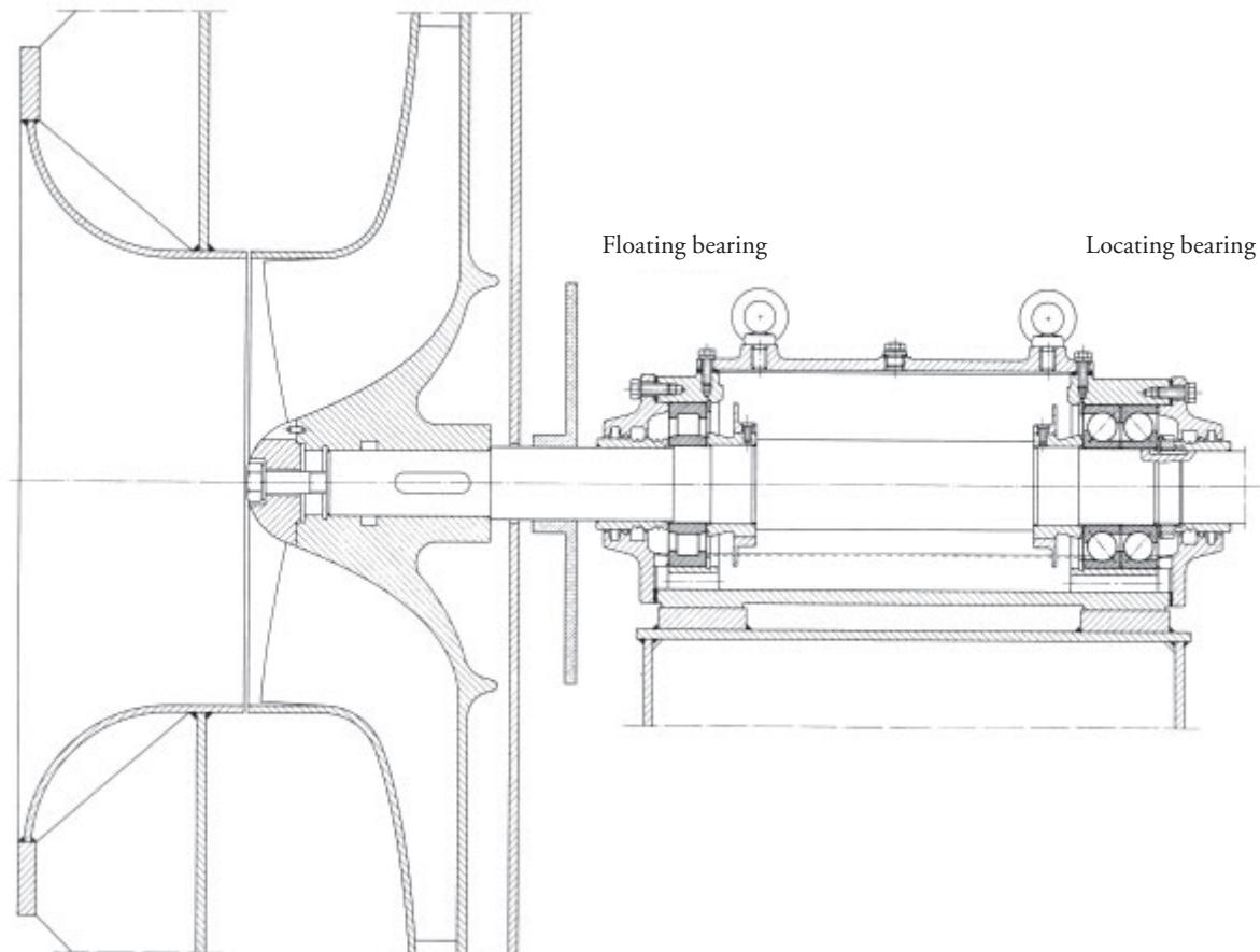
119: Rotor bearings of a hot gas ventilator
