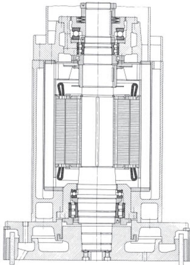
18: Bearing arrangement of a surface grinding spindle
