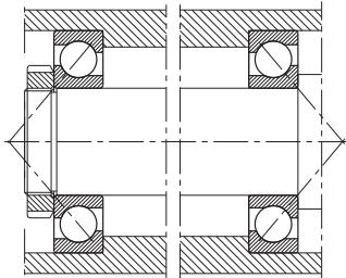
Adjusted bearing arrangement
