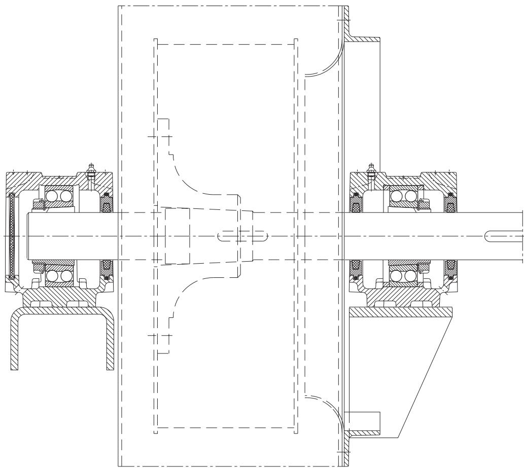
120: Rotor mounting of a fresh air blower
