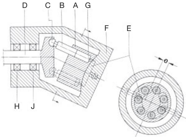
In axial piston machines only some of the pistons are pressurized (normally half of all pistons). The individual forces of the loaded pistons are combined to give a resultant load which acts eccentrically on the swash plate and/or drive flange.
