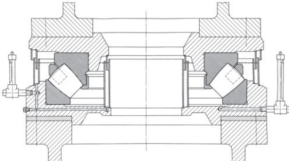
77: Crane pillar mounting with a spherical roller thrust bearing
