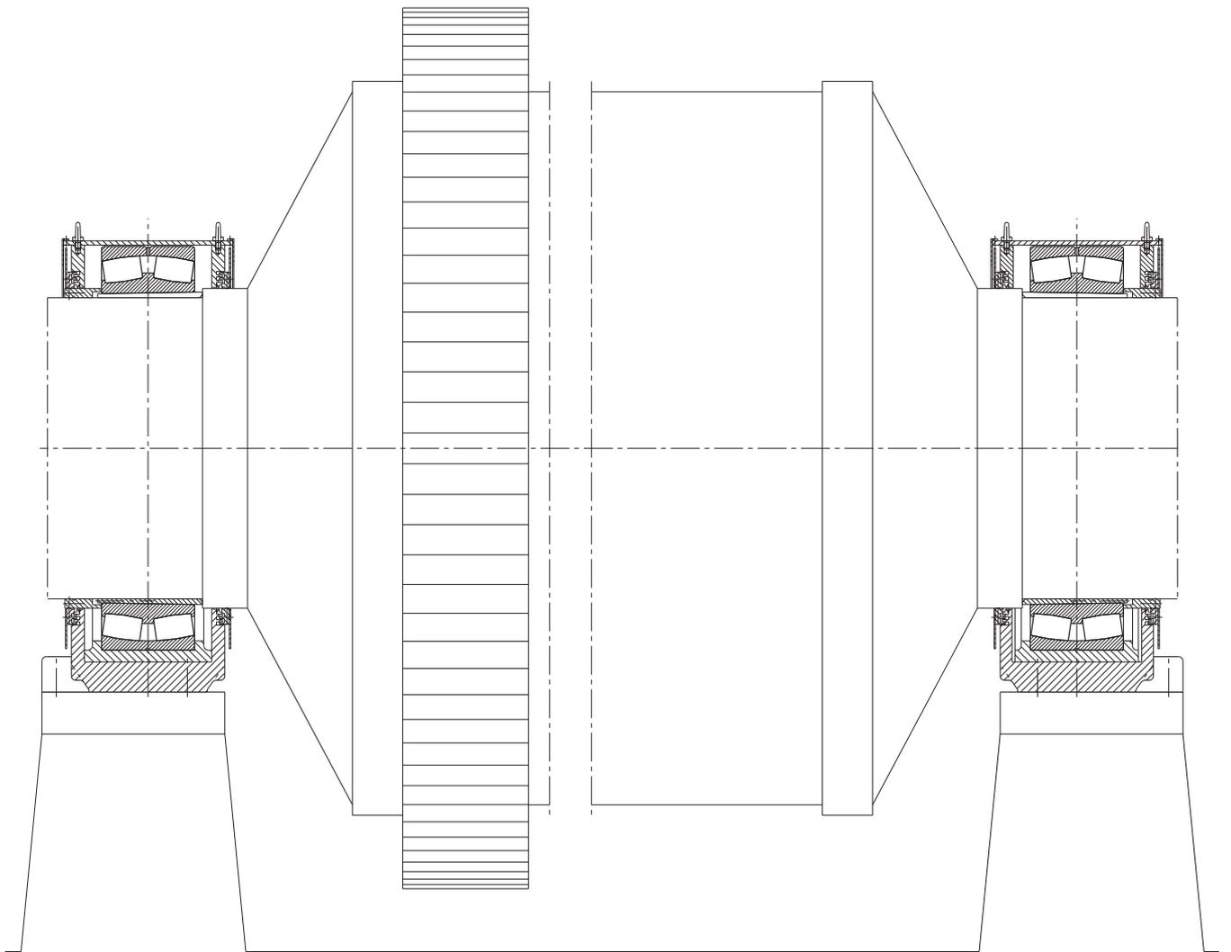
95: Ball tube mill mounting
