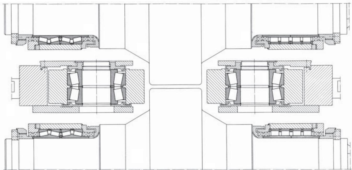
108a: Bearing mounting of horizontal rolls in the preloaded roughing stands
