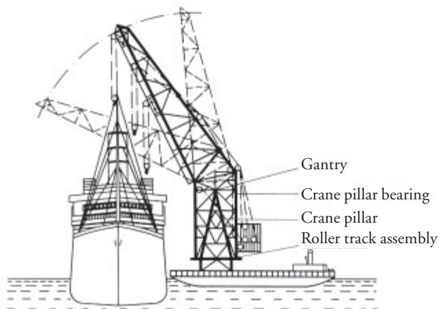
At the pillar foot the gantry is supported on a roller-track assembly (see example no. 79).
