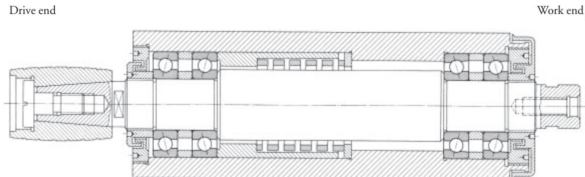
16: Bearing arrangement of a bore grinding spindle
