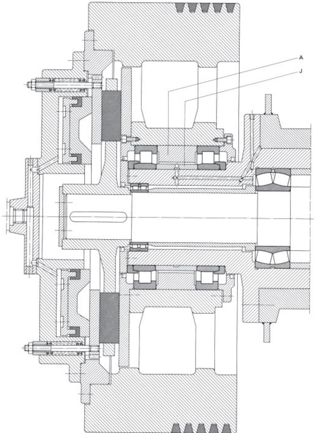
22: Flywheel bearing arrangement of a car body press
