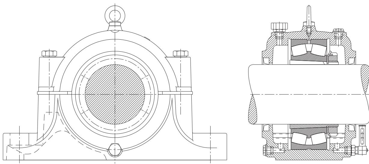
61b: Ship shaft bearing, Spherical roller bearing in S30.K housing
