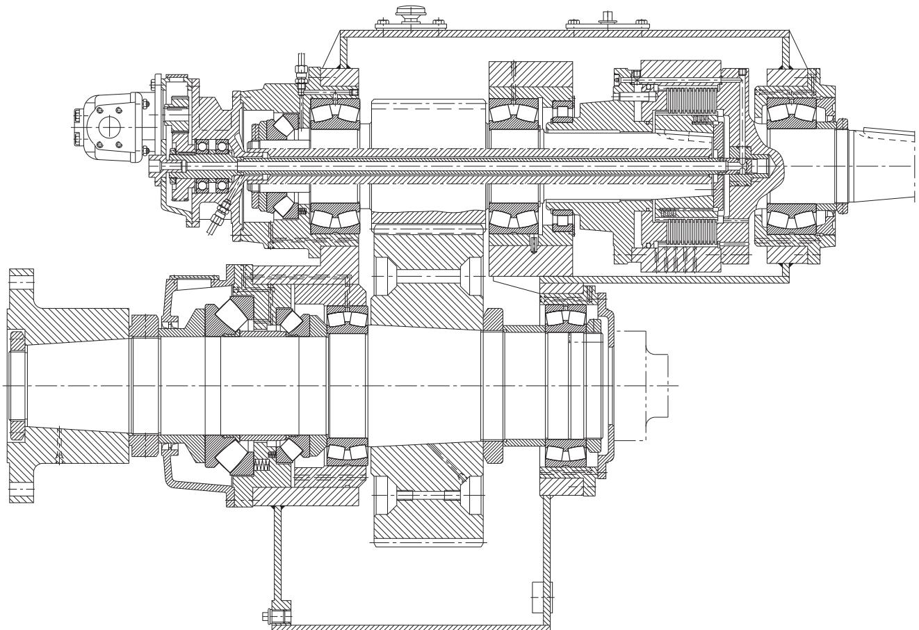
28: Bearing arrangement of a marine gear
