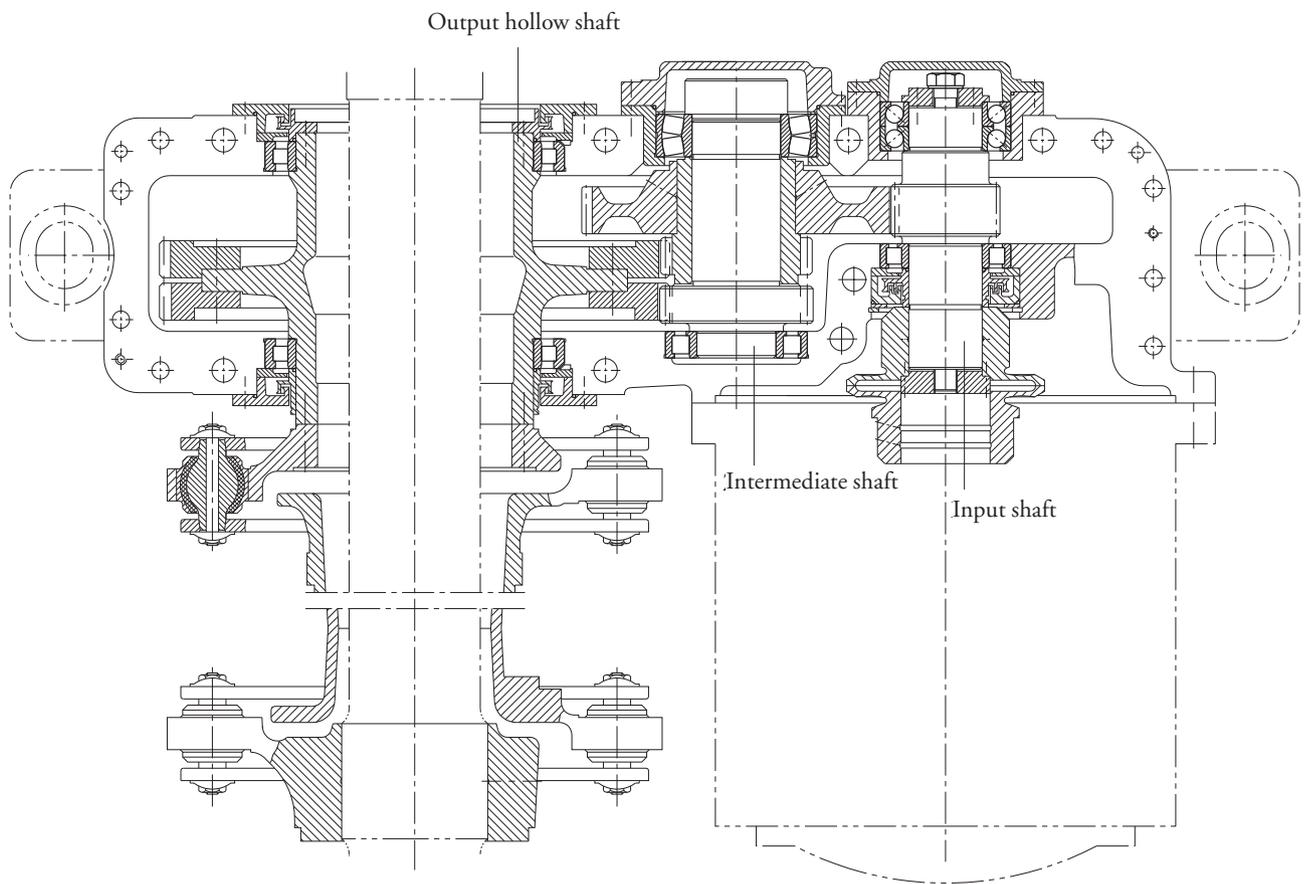
54: Spur gear transmission for the underground or subway
