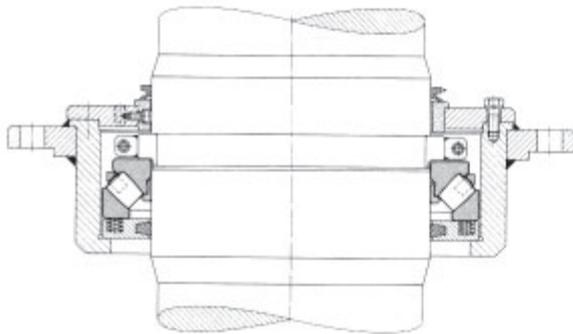
58: Rudder carrier bearing FAG RS9284N.1.....
