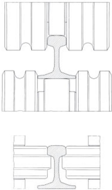
Each machine features nine straightening rolls, four of which are being driven. The straightening rolls with diameters of 600...1,200 mm form an overhung arrangement in order to allow easy replacement.
