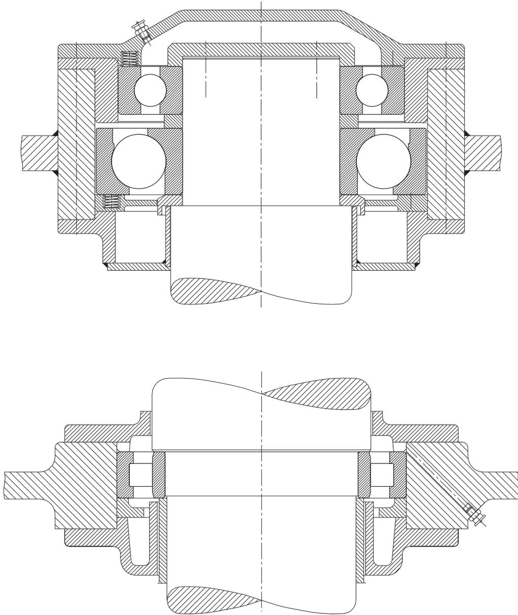
6: Rotor bearing arrangement of a vertical-pump motor
