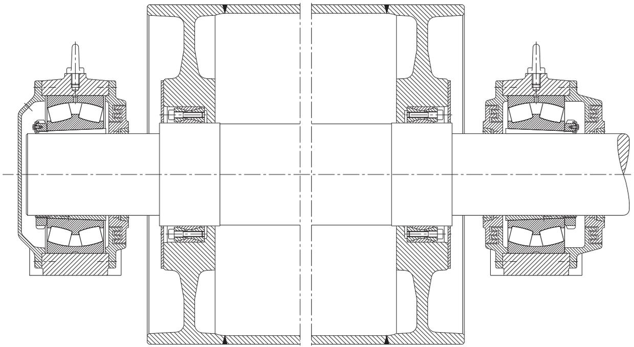
83: Head pulley bearing arrangement of a belt conveyor
