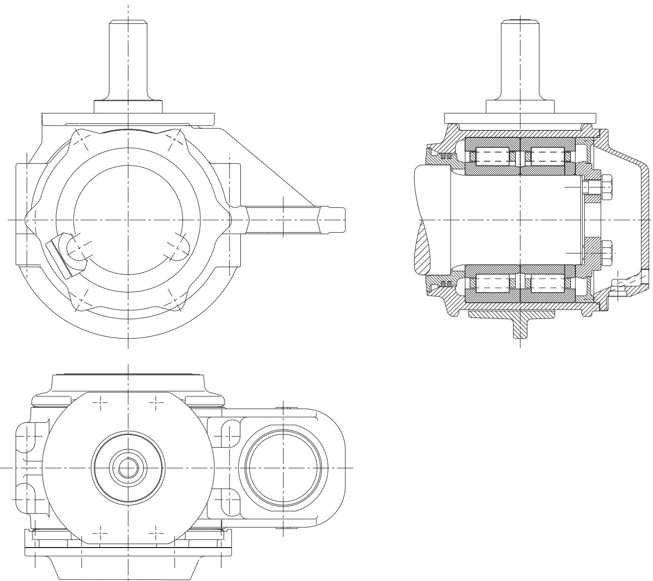
42: Axle box roller bearings of an Intercity train carriage
