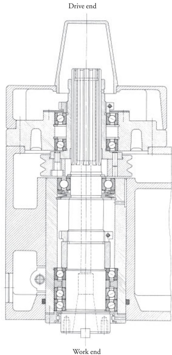
15: Bearing arrangement of a vertical high-speed milling spindle
