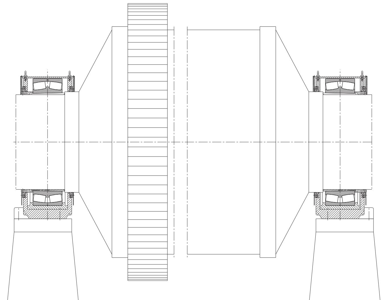
95: Ball tube mill mounting
