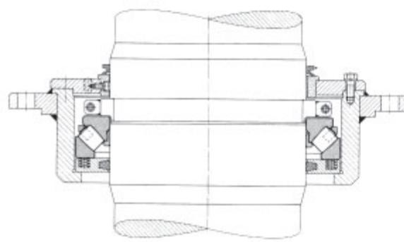
58: Rudder carrier bearing FAG RS9284N.1.....
