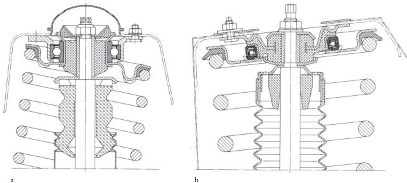
39: Shock absorbing strut for the front axle of a car; a: single path solution; b: dual path solution
