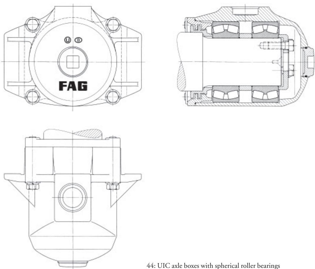
44: UIC axle boxes with spherical roller bearings
