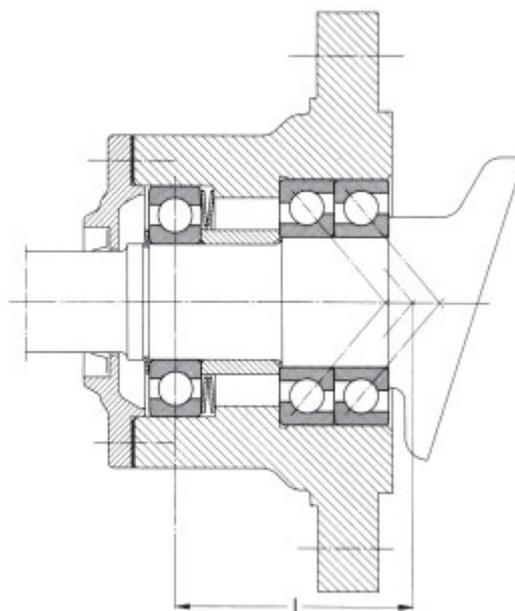
116: Drive flange of an axial piston machine
