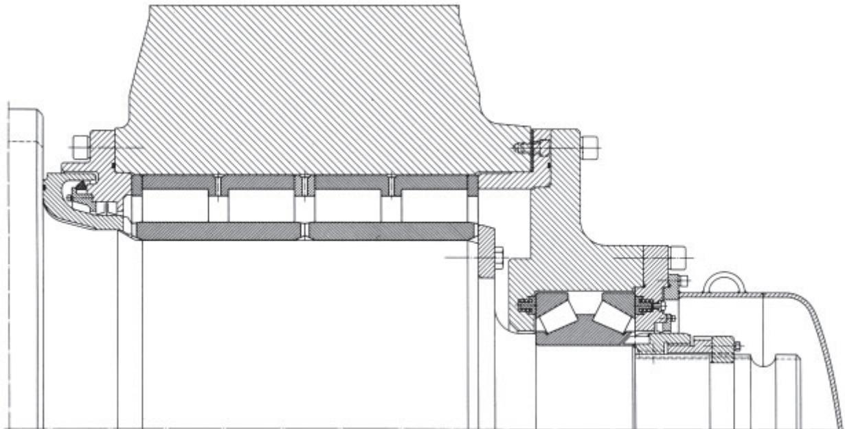
104a: Back-up roll mounting of a four-high cold rolling stand for aluminium (identical bearing arrangements at drive end and operating end)
