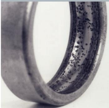
**Symptoms:** Red/brown stains or deposits on rolling elements, raceways or cages. Increased vibration followed by wear, increase in radial clearance or loss of preload.
