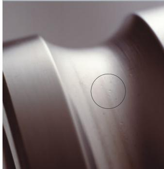
**Symptoms:** Denting of rolling elements and raceways, causing vibration.
