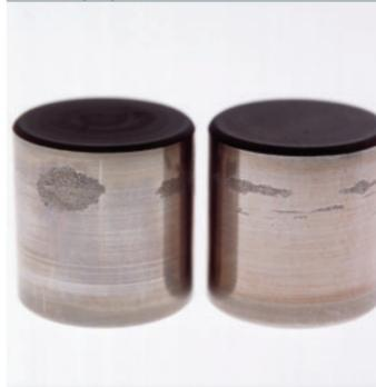
**Symptoms:** Spotted smear marks, or roughening of rolling elements or raceways.
