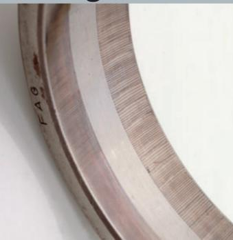
**Symptoms:** Brownish marks parallel to the axis on a large part of the raceway, or covering the entire raceway circumference.
