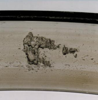
**Symptoms:** Often referred to as spalling, and indicated by the fracture of the running surfaces and subsequent removal of small discrete particles of material from the inner ring, outer ring or rolling elements. Spalling is progressive, and once initiated will spread with continued operation. It is always accompanied by a noticeable increase in vibration.
