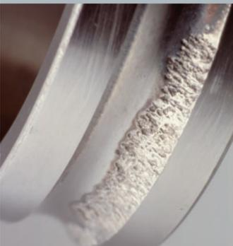
**Symptoms:** Heavy rolling element wear paths, evidence of overheating, and widespread fatigue areas (spalling).
