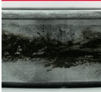
**Symptoms:** Fretting, the generation of fine metal particles which oxidize, leaving a distinctive brown color. Wear at the fitting surfaces causing noise and runout problems, possible fatigue fracture, and possible disturbance of floating bearing function.
