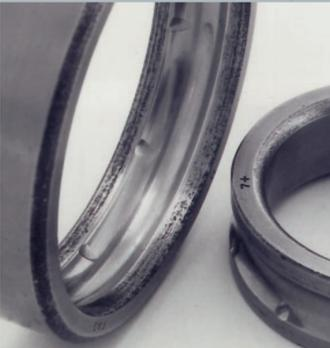
**Symptoms:** Brinell marks appear as indentations in the raceways, increasing bearing vibration (noise). Severe brinell marks can cause premature fatigue failure.
