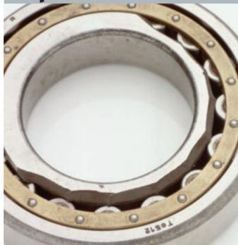
**Symptoms:** Supporting lips are partly or completely broken off or cracked.
