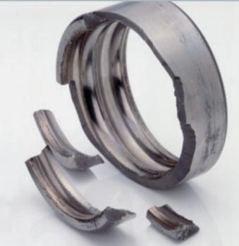
**Symptoms:** Normally a crack spreads evenly in the circumferential direction, with several fractured pieces often originating. With axial load, these fractures occur as a rule a little beyond the middle of the raceway. The outer ring outside surface normally shows an irregular load carrying pattern.
