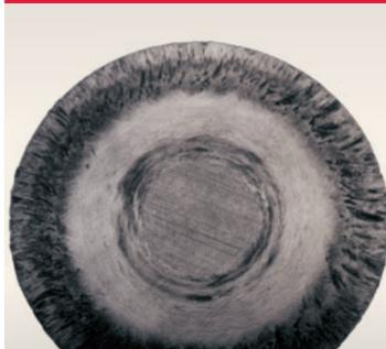
**Symptoms:** Partial or large-area welding and deep scratches in the lip and roller face areas. Also lubricant coking in this area.
