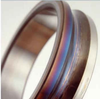
**Symptoms:** Discoloration of the rings, rolling elements and cages from gold to blue. Temperatures in excess of 400 °F can anneal ring and rolling element materials, reducing the bearing capacity and causing early failure. In extreme cases, the bearing components will deform. Temperature rise can also degrade or destroy lubricant.
