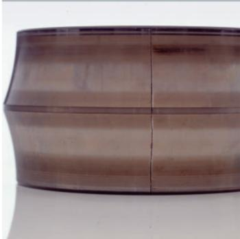
**Symptoms:** Inner ring cracked in the axial direction. Slightly rounded fractured edges indicate that fracture originated during operation and was cycled (crack edges may break off after prolonged operation). Sharp edged cracks indicate fracture during dismounting.
