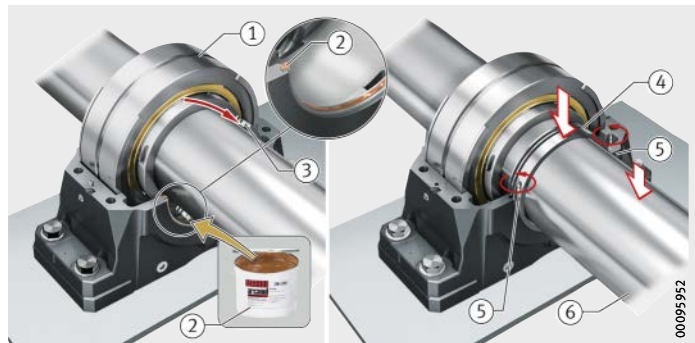
Figure 45 Mounting a split labyrinth seal
