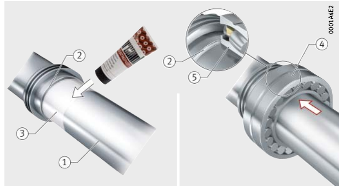
Figure 14 Applying mounting paste, sliding on the bearing
