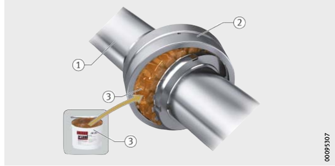
Figure 30 Greasing the bearing
