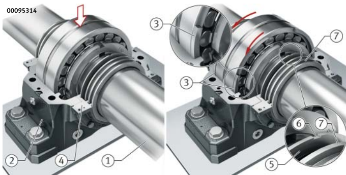
Figure 34 Inserting the shaft, locating bearing arrangement
