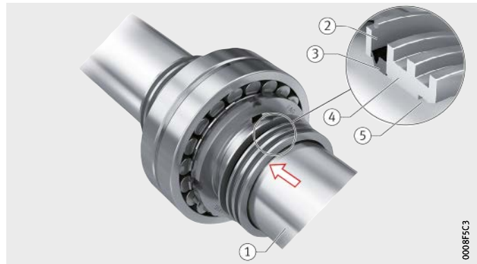
Figure 31 Mounting the Bolt-on outer seal
