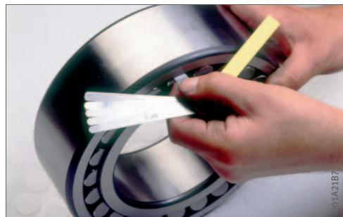
The value for the radial internal clearance  $s_i$  ► 3 must be documented after the measurement.
