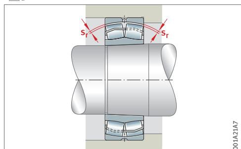
The bore and seating surfaces on the shaft, adapter sleeve or withdrawal sleeve must then be cleaned. Mounting paste or lubricant must not be used.
