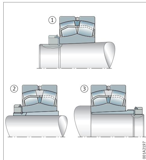
The radial internal clearance is measured over both rows of rollers using a feeler gauge, prior to mounting the spherical roller bearing ► 2.
